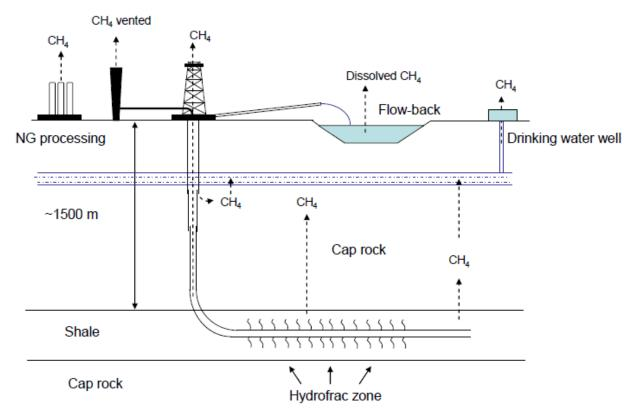
Figure 6.2.2-3. Methane (CH<sub>4</sub>) Flows during Hydraulic Fracturing
