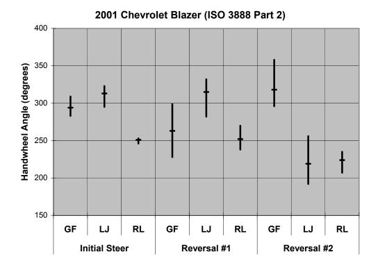
Figure 12: Handwheel input repeatability observed during ISO 3888 Part 2 Double Lane Change testing performed with the Chevrolet Blazer
