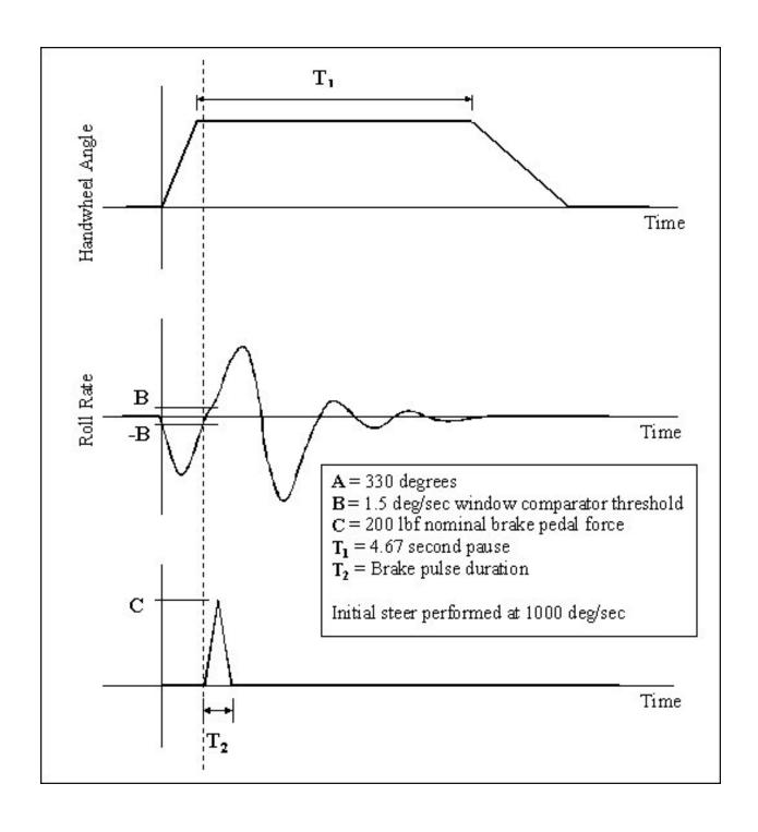
Figure 3: J-Turn with Pulse Braking Handwheel Steering Angle and Brake Pedal Force
