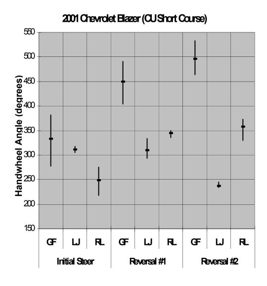
Figure 15: Handwheel input repeatability observed during Consumers Union Short Course Double Lane Change testing performed with the Chevrolet Blazer
