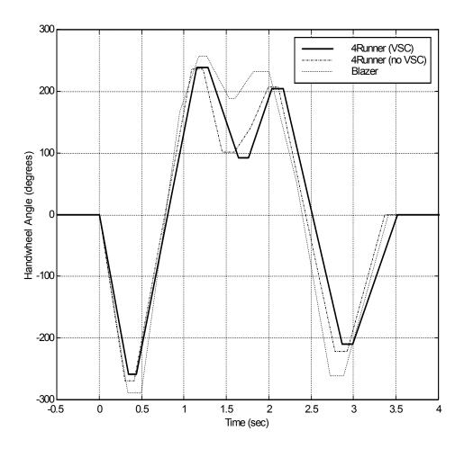
Figure 17: ISO 3888 Part 2 Pseudo-Double Lane Change Steering Inputs
