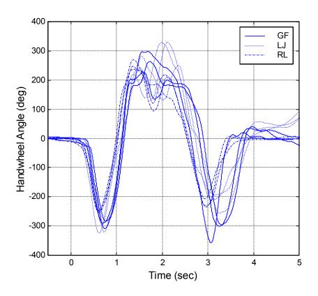
Figure 11: Handwheel input repeatability observed during ISO 3888 Part 2 Double Lane Change testing performed with the Chevrolet Blazer
