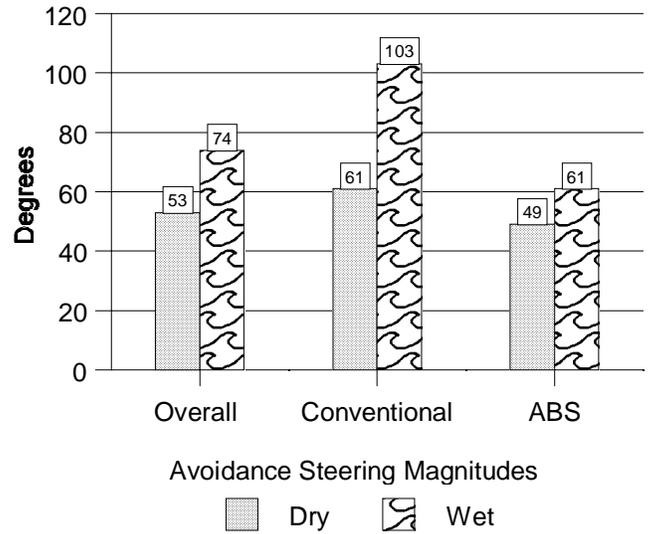
**Figure 4.** Magnitude of avoidance steering inputs.
