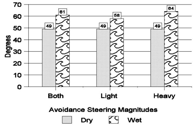
**Figure 7.** Magnitude of avoidance steering inputs by brake pedal feedback.
