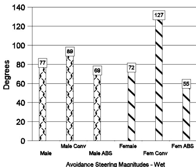
**Figure 11.** Magnitude of the avoidance steering input by gender and brake system - wet study.
