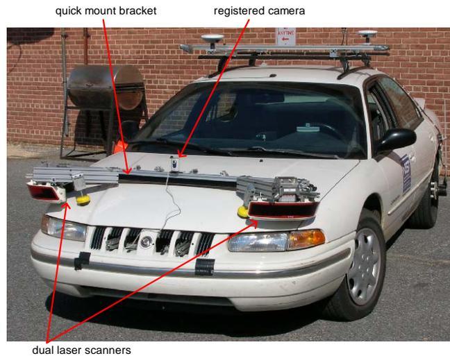
Figure 7. Dual-head laser scanner mounted on NIST/DOT vehicle
