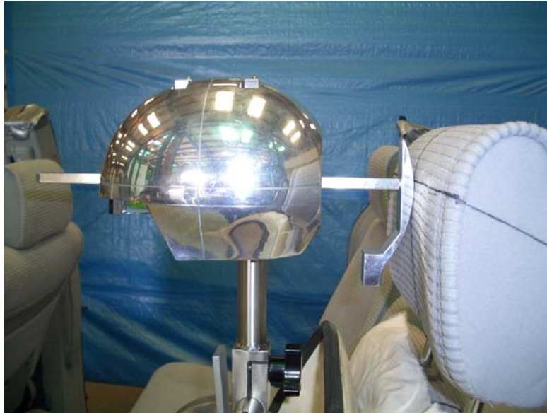
Figure 7. Measuring backset with HRMD
