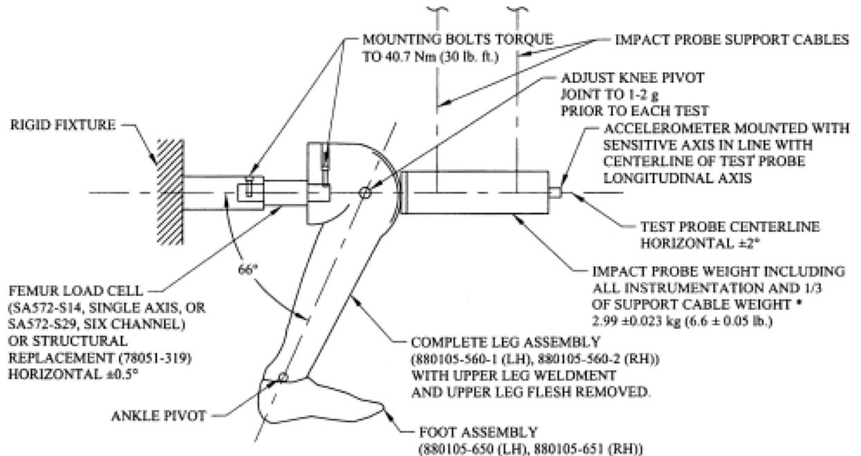
\* 1/3 CABLE WEIGHT NOT TO EXCEED 5% OF THE TOTAL IMPACT PROBE WEIGHT
