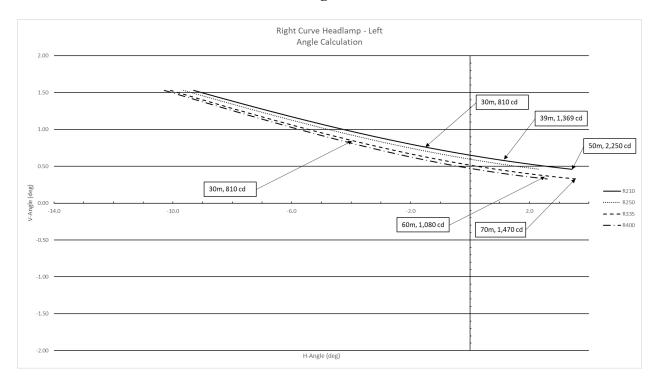
Figure A.1. Horizontal angle for each headlamp (right and left) at each extreme of each right curve
