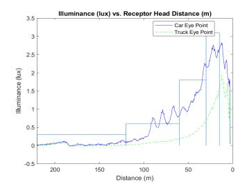
As with the other oncoming left curve scenarios, the closest SAE test analogue is with an oncoming fixture in Position 1. Again, NHTSA's testing showed that, compared to NHTSA's test, the SAE test resulted in much lower illuminance at close distances than on an actual curve. See Figure 22. Thus, data indicate again that the two test methods can yield different results, and that the actual curve test is preferable because it would be more evaluative of real-world performance.
