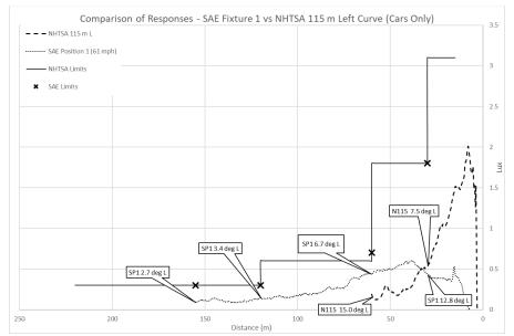
Note: Illuminance as measured from photometer corresponding to the passenger car driver's eye point.
