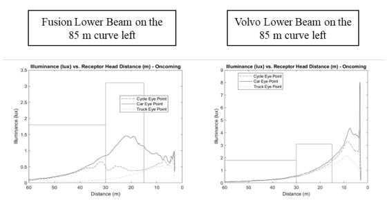
Next, NHTSA believes that this modified specification is within the capabilities of most current ADB systems. On a curve with a 100 m radius, at the highest vehicle speed specified for
