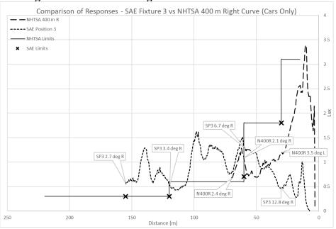
Figure 27. Lexus ADB Right 335 & SAE Fixture Position 3
