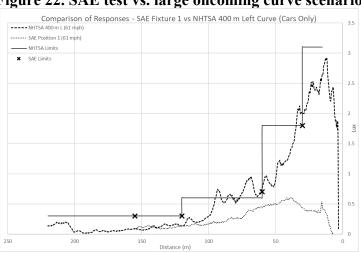
Figure 22. SAE test vs. large oncoming curve scenario
