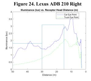
The ADB system NHTSA tested had more exceedances when tested to the most closely analogous SAE J3069 scenario (with the test fixture in Position 3) compared to NHTSA's test. See Figure 25. This is because at the measurement distances in this scenario, Fixture Position 3 is in the bright (right-side) portion of the beam pattern, while the fixture in NHTSA's test scenario is in the less-bright portion of the beam pattern (center-right to center-left).
