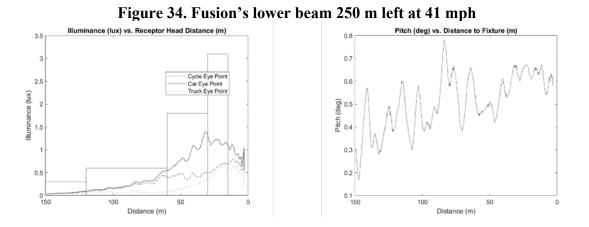
Here, where the maximum pitch occurs (at about 85 m), there is a peak in the illuminance reading. The highest illuminance value (at about 31 m) also coincides with a positive spike in pitch. (In these instances, the pitch did not exceed the average pitch by more than 0.3 degrees, so if this were a compliance test, these values would still be considered when assessing compliance; in any case, in this instance, all illuminance values are still within the glare limits).
