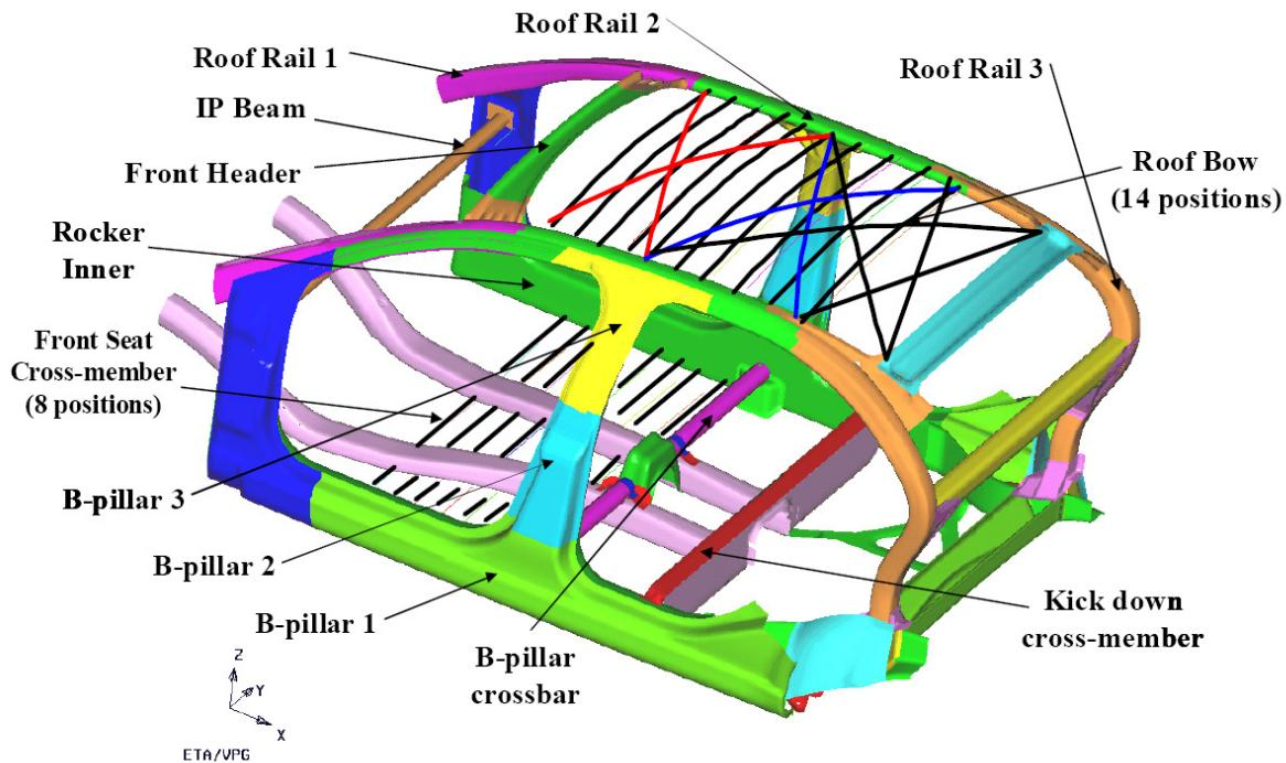
**Figure 3-4:** Example of CAE optimization of the design and position of the roof rails and front seat cross-member for the “Future Generation Passenger Compartment.”<sup>53</sup> The thin lines represent relative positions for roof bows and front cross-members considered during iterations of the CAE analysis of the vehicle structure. The different colors given to the structural components represent differences in sectional material thickness within this particular CAE modeling run.
