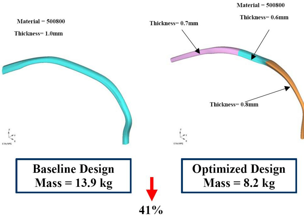
Figure 3-5: Example of CAE optimization of a roof-rail design for the “Future Generation Passenger Compartment” that reduces component mass by 41%.<sup>53</sup>
