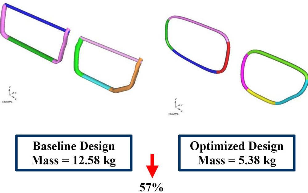
Figure 3-6: Example of CAE optimization of a door-beam design for the “Future Generation Passenger Compartment” that reduces component mass by 57% and reduces part count and assembly.<sup>53</sup>
