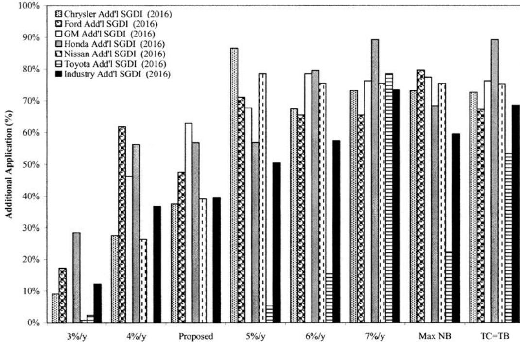
Figure IV.F.10. Additional Application of Engine Turbocharging & Downsizing (MY 2016)
