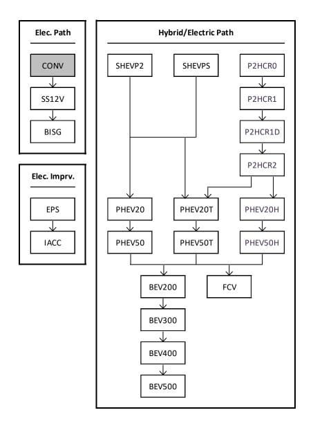
Figure 3-2 – Electrification Technology Paths in the CAFE Model
