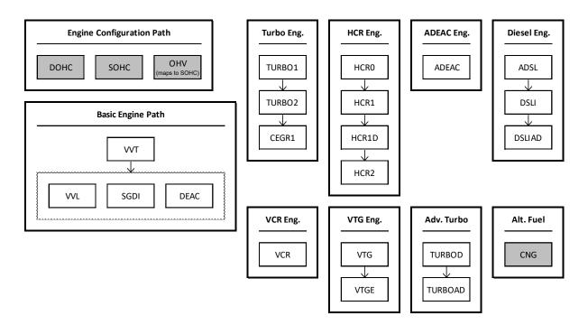
Figure 3-1 – Engine Technology Paths in the CAFE Model
