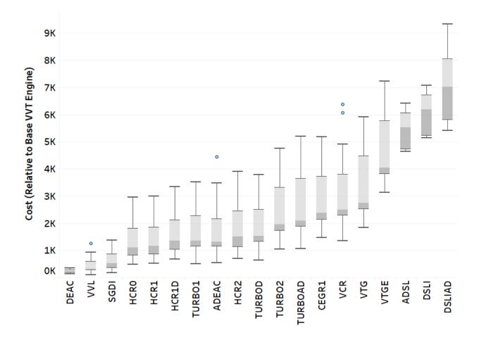
Figure 3-9 – Engine Technology Cost Distributions (Retail Price Equivalent), 2020
