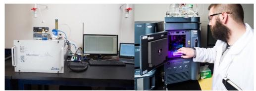
Figure 9. MKS Multigas 2030 FTIR and Waters Aquity HPLC in the DADSS Research Laboratory
