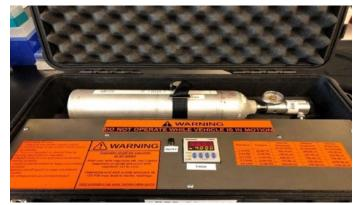
Figure 10. Portable Gas SCD
