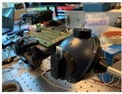
Figure 8. The sensor setup includes a 3" integrating sphere, laser package, and electronic board
