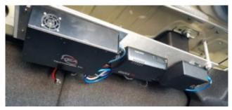
Figure 16. Equipment located in the trunk, from left to right, DAS, WIFI LTE, network switch, and DVR
