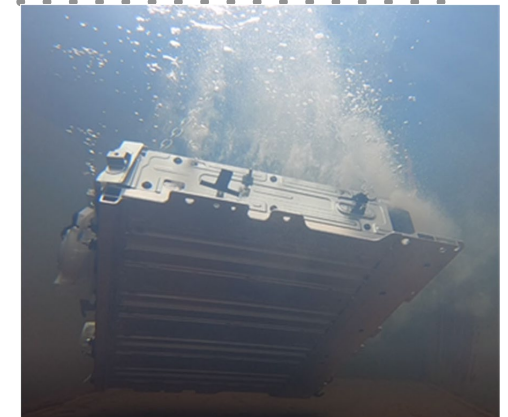
Water ingress and reaction
