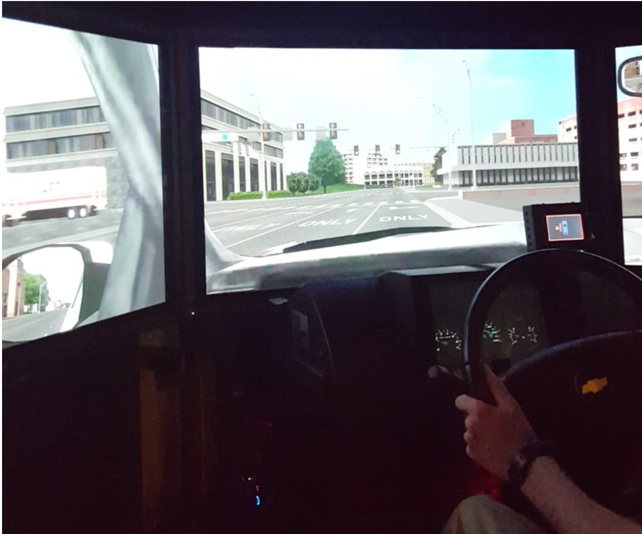
Figure 3. Level 2 (audio-visual) display on simulator dash to right of steering wheel
