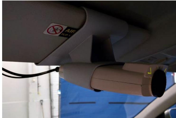
Figure 1. 3 rd Generation breath-based sensor
