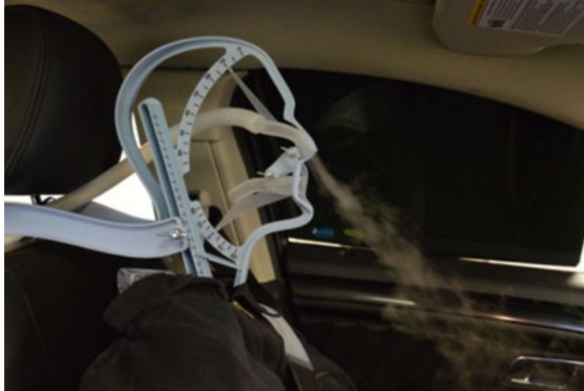
Figure 11 Anthropomorphic Manikin with Simulated Breathing Developed to test Breath-based DADSS Technology in DADSS X1 Research Concept Vehicle
