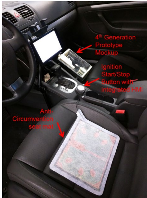
Figure 2. Ignition Start/Stop anti-circumvention concept with 4 th Generation touch-based mockup
