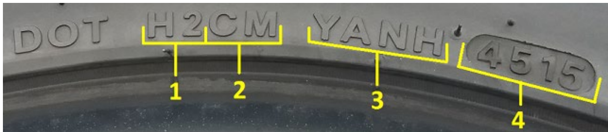
Figure 1. Example of a TIN following the “old requirements” with individual sections indicated
