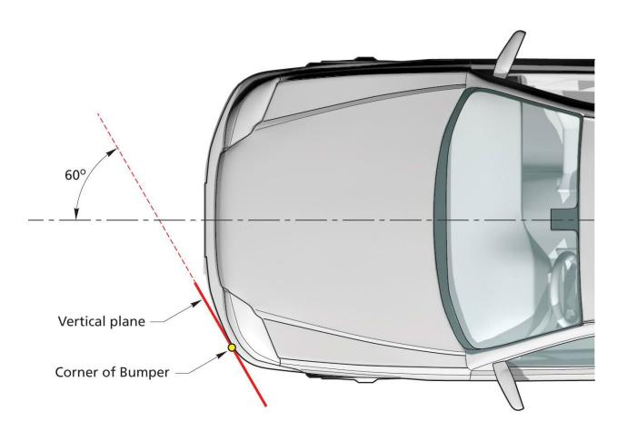
Figure 9: Determination of the Bumper Corner in Euro NCAP  $^{102}$
