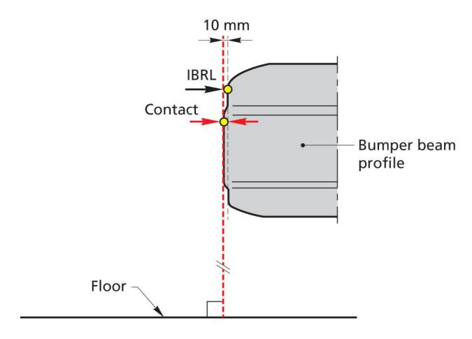
Figure 6: Internal Bumper Reference Line (IBRL)<sup>77</sup>
