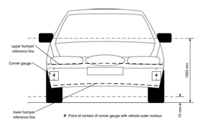
Figure 11: Determination of Bumper Corner with Corner Gauge 104
