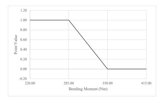
Figure 13: Upper Legform Bending Moment Scoring
