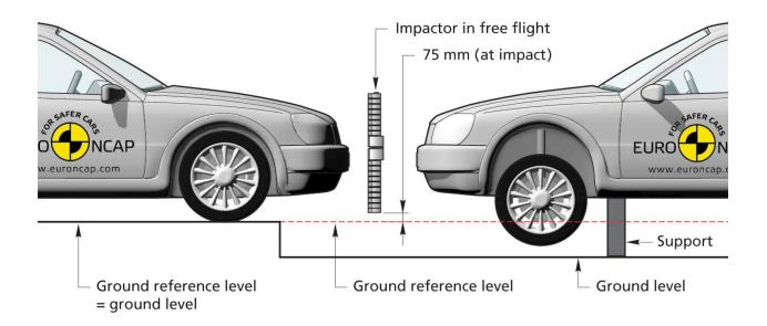
Figure 8: FlexPLI to Bumper Test Setup<sup>82</sup>
