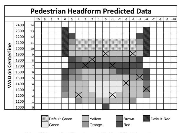
Figure 17: Example of Manufacturer's Predicted Head Impact Data
