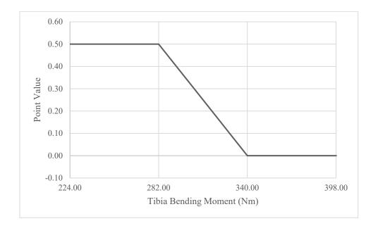
Figure 15: FlexPLI Tibia Bending Moment Scoring
