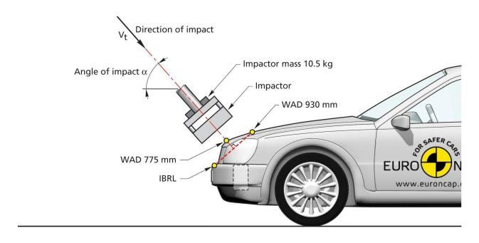
Figure 7: Upper Legform to WAD775 Test Setup<sup>78</sup>
