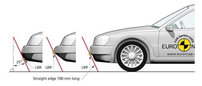
Figure 5: Marking the Lower Bumper Reference Line (LBRL)<sup>74</sup>
