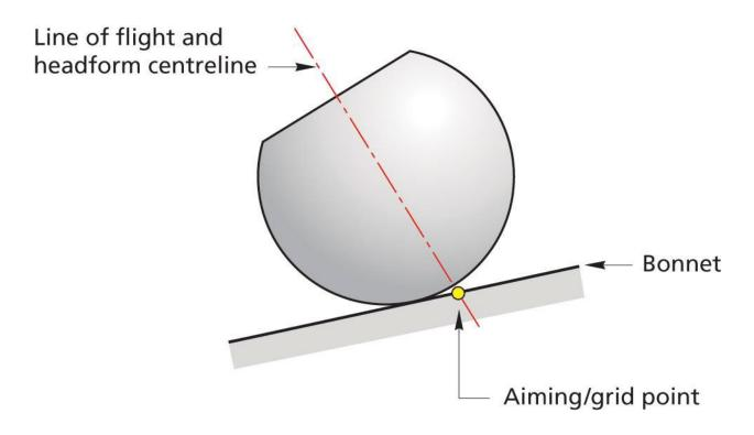
Figure 4: Head Impact Test Setup<sup>67</sup>
