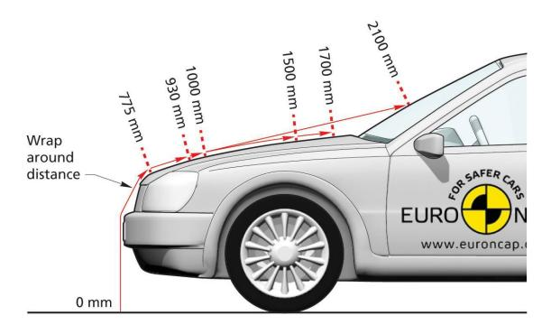
Figure 3: Wrap Around Distance (WAD)<sup>56</sup>
