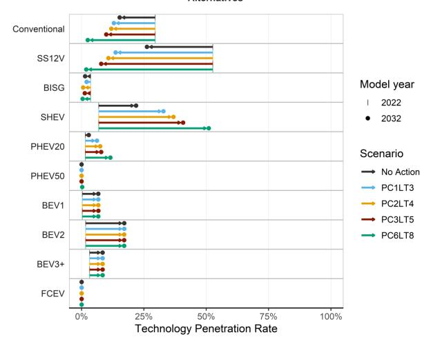
Figure 8-10: Electrified Powertrain Technology Penetration Rates by Model Year
