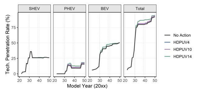
Figure 8-65: Hybrid and Electrified Technology Penetration Rates by Model Year
