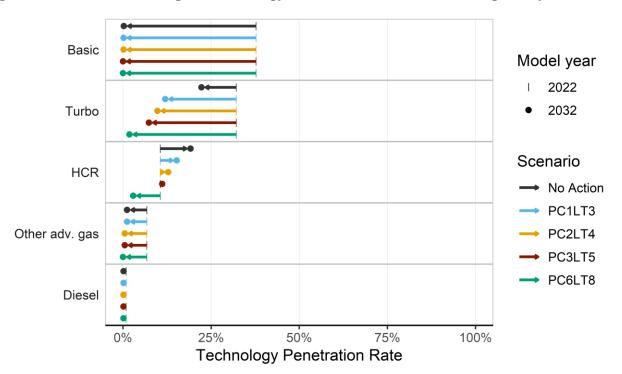
Figure 8-7: Prevalence of Engine Technology in the Fleet Under Different Regulatory Alternatives
