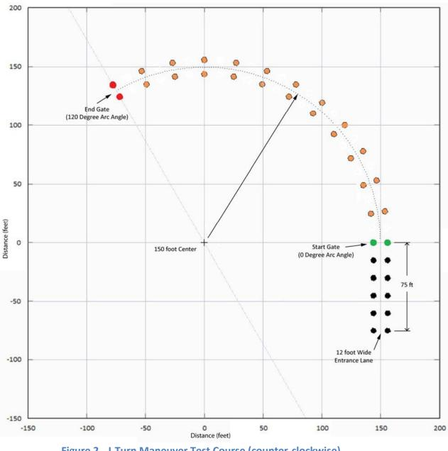
Figure 2 - J-Turn Maneuver Test Course (counter-clockwise)
