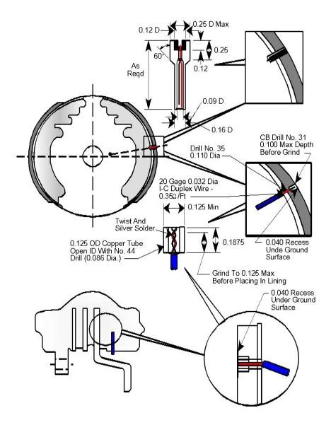
Figure 1 – Typical Plug-type Thermocouple Installation
