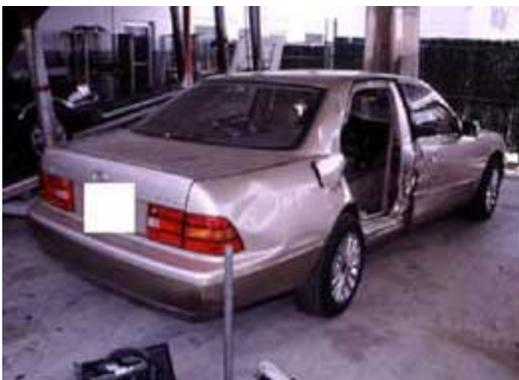
This case involved a 12 year old female who was the left rear-seat occupant in a 1997 Lexus LS 400. The occupant was wearing the available 3-point lap and shoulder restraint. The case vehicle was struck on its right side by a 1997 Toyota Tercel. The point of impact was at the rear right door opposite from the case occupant (see Figure 2.6). The lateral delta V was estimated to be 15 mph and the PDOF was 2 o'clock.
