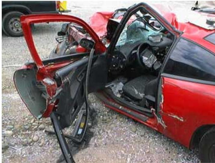
The bumper frame height mismatch and override resulted in significant intrusion of the instrument panel and consequent lower extremity injuries.
