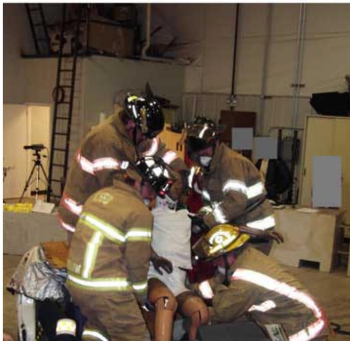
The dummy neck loads are monitored to give firefighter rescuers feedback on techniques.
