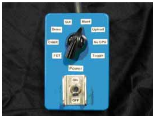
Figure 15. DAS mode control box
