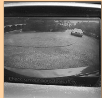
Rear-view cameras show a wide angle view of the area behind the vehicle.
