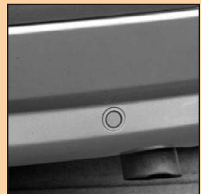
Some backing aids use sensors placed on the rear bumper which alert drivers if there are obstacles behind the bumper.
