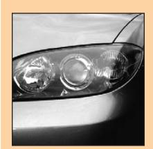
Directionally Adaptive Headlamps adjust the aim of the headlight beams to illuminate the roadway based on inputs from the vehicle (steering wheel, speed, yaw). "I'm pleased with
