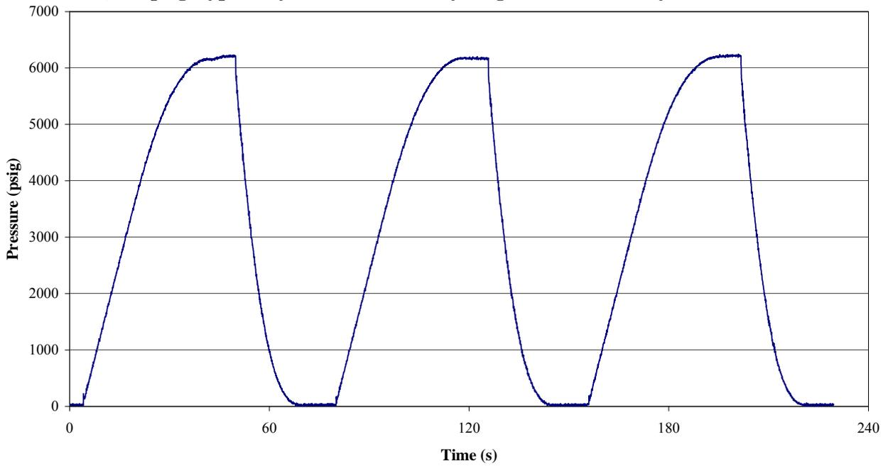
**Figure B-2. 5000-psig Type 3 Cylinder Pressure Cycling Test Data (2 of 2).**
