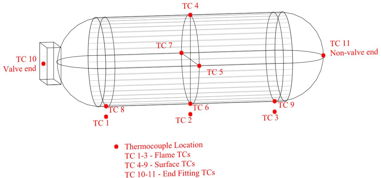
**Figure 2. Thermocouple Layout.**
