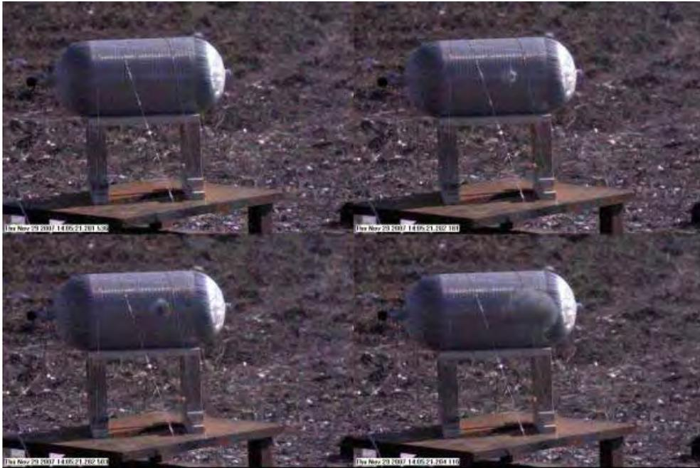
Figure 6. High-Speed Video Frames of 5,000-psig Type 3 Cylinder Penetration Test.
