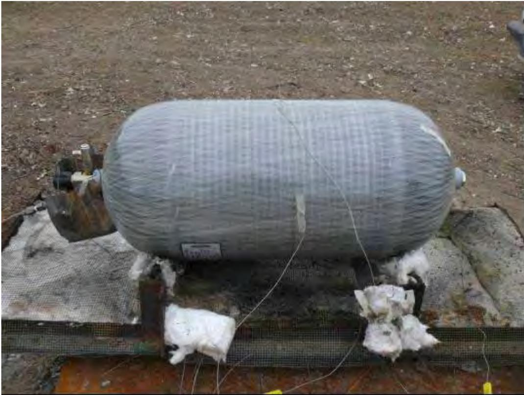
**Figure C-1. Overall Setup for Cylinder Bonfire Tests – 5,000-psi Type 3 Cylinder Shown.**
