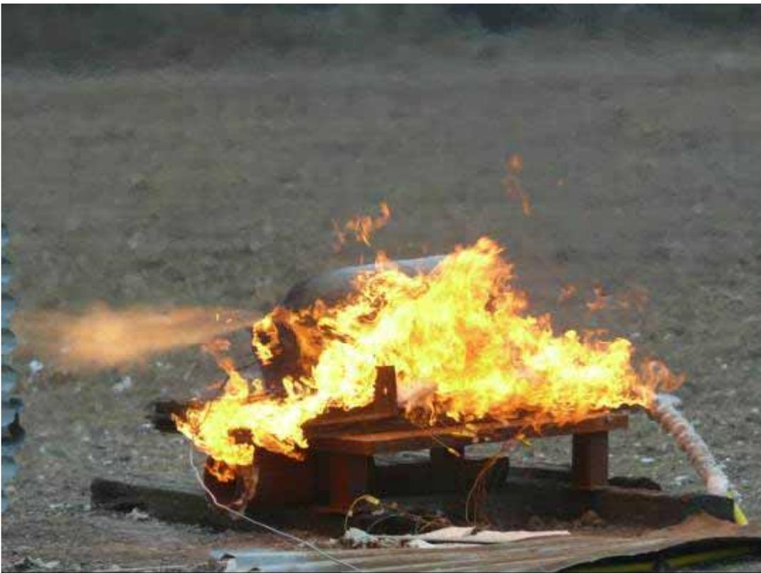
**Figure C-2. View of 5,000-psi Type 3 Cylinder Venting.**
