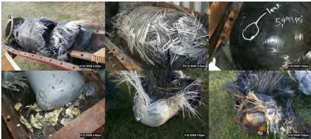
**Figure 5. Cylinders Following Burst Pressure Tests.
