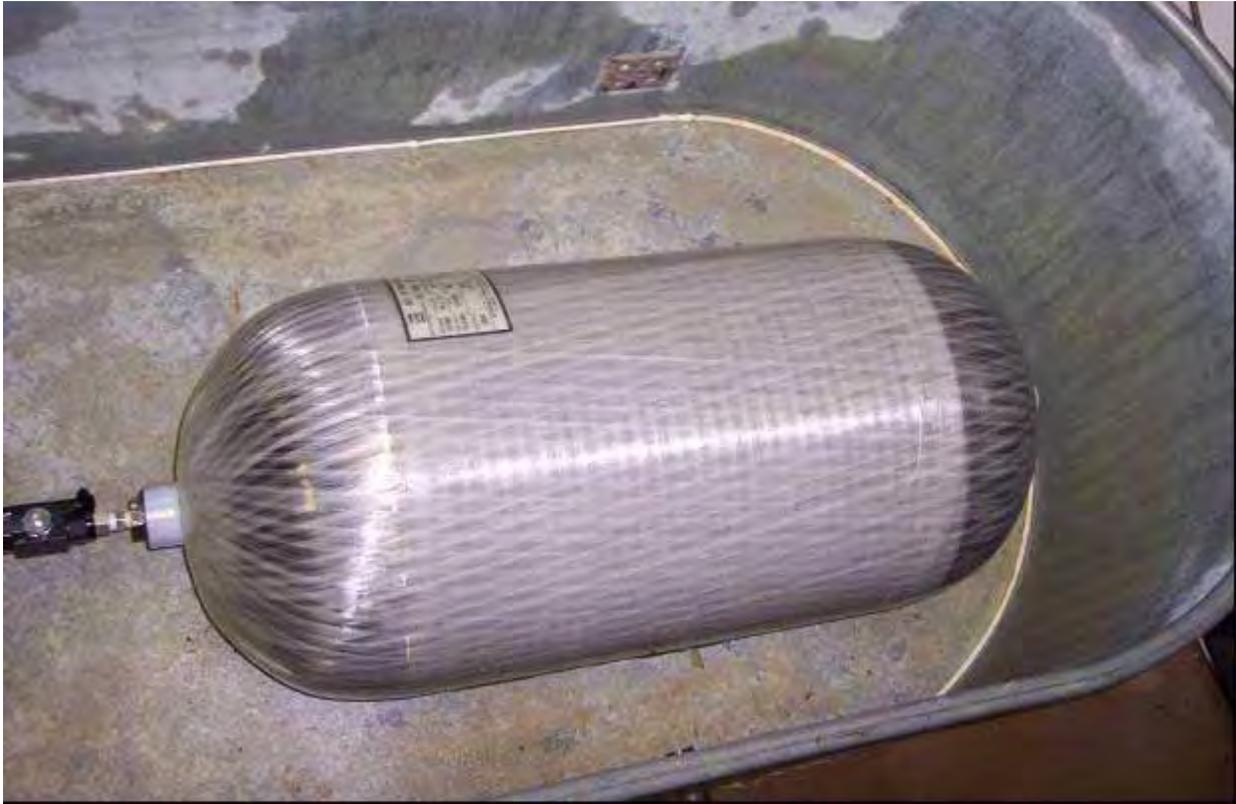
**Figure C-5. View of 10,000-psi Type 4 Cylinder Venting.**
