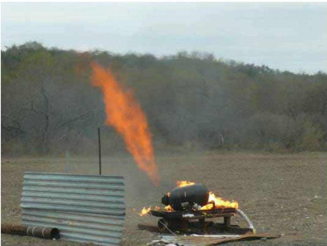
**Figure C-4. View of 5,000-psi Type 4 Cylinder Venting.**
