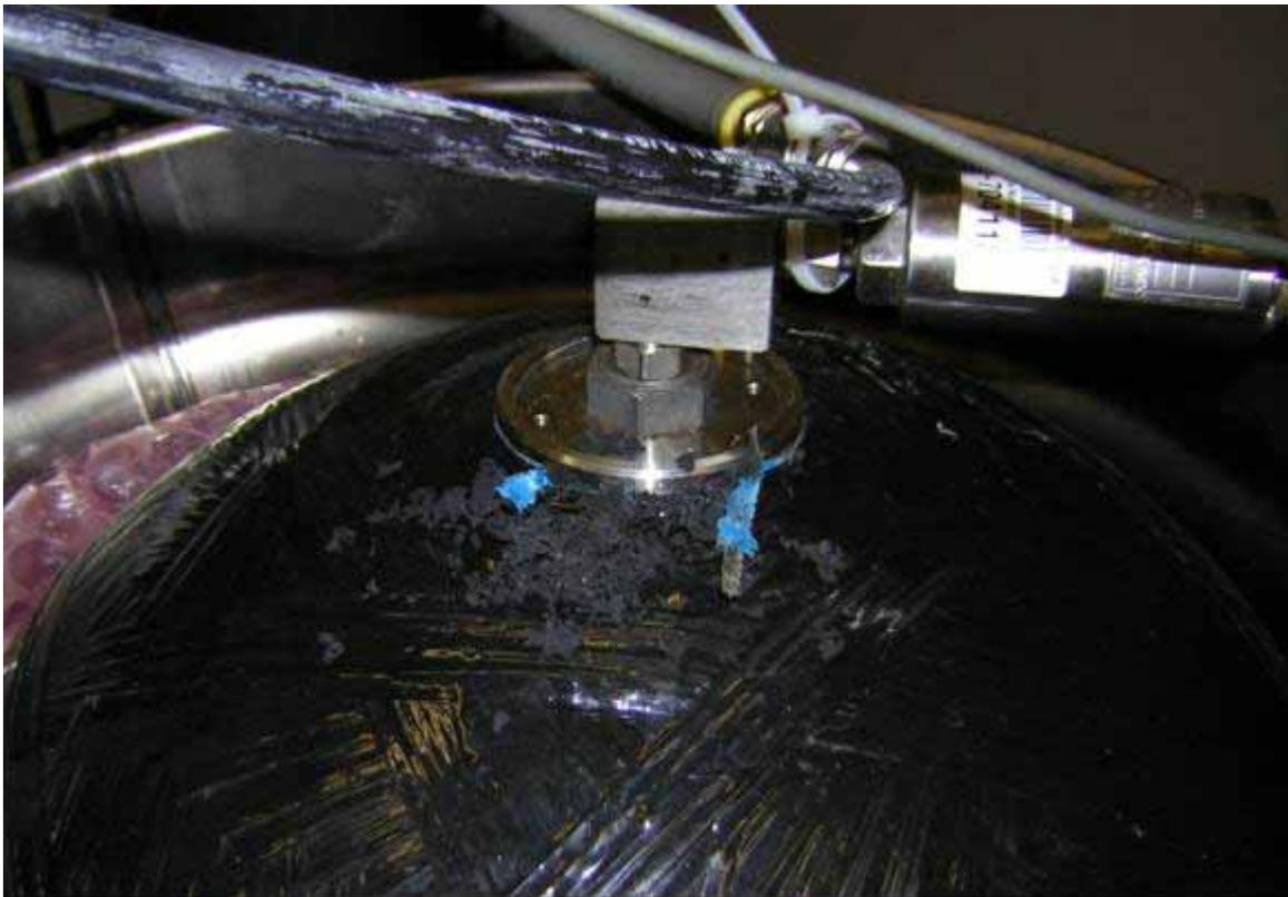
**Figure 4. Condition of 10,000-psig Type 4 Cylinder Following Initial 13,000 Cycles.**
