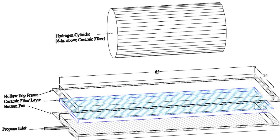
**Figure 1. Exploded View of Test Bench Assembly.**
