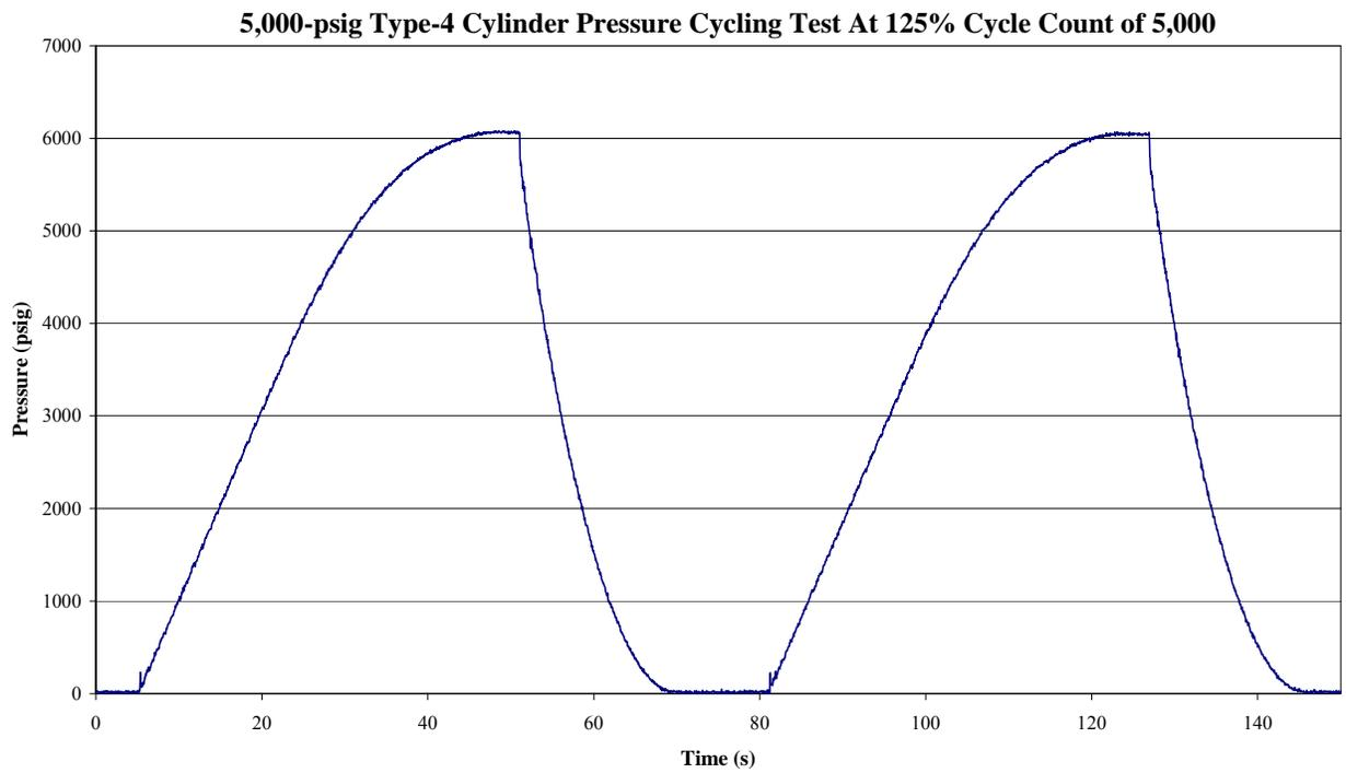
**Figure B-4. 5,000-psig Type 4 Cylinder Pressure Cycling Test Data (2 of 2).**
