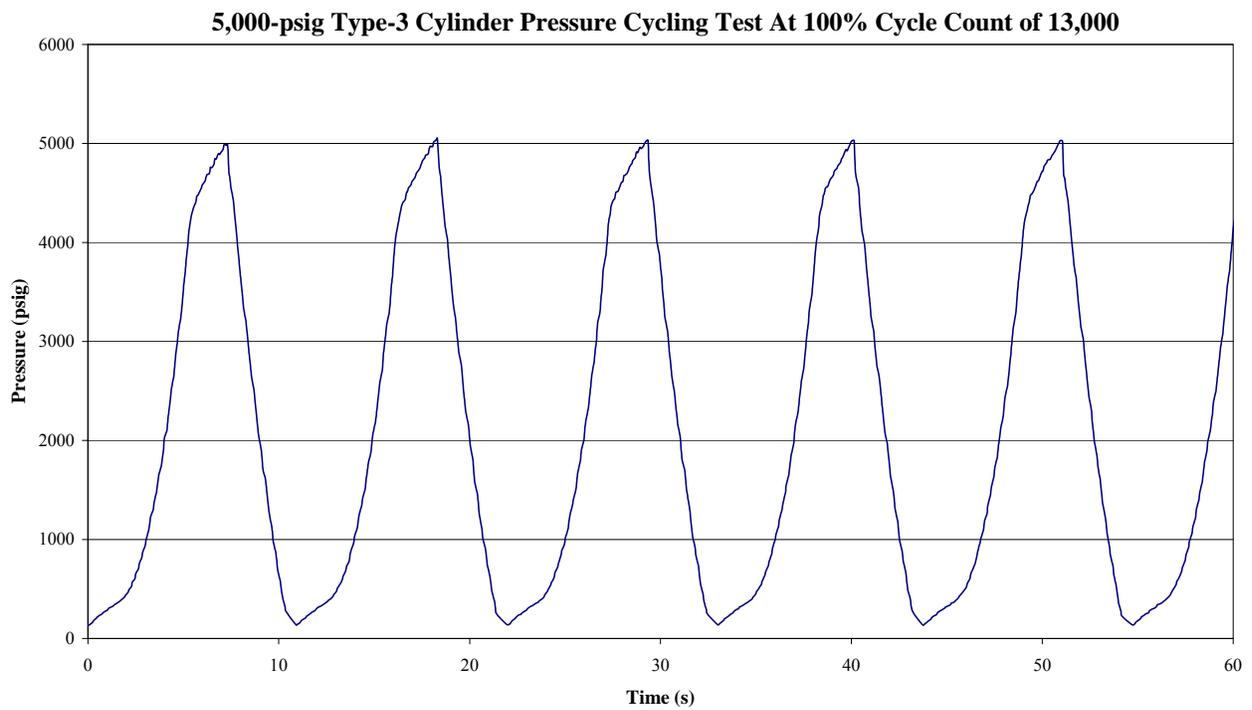
**Figure B-1. 5000-psig Type 3 Cylinder Pressure Cycling Test Data (1 of 2).**
