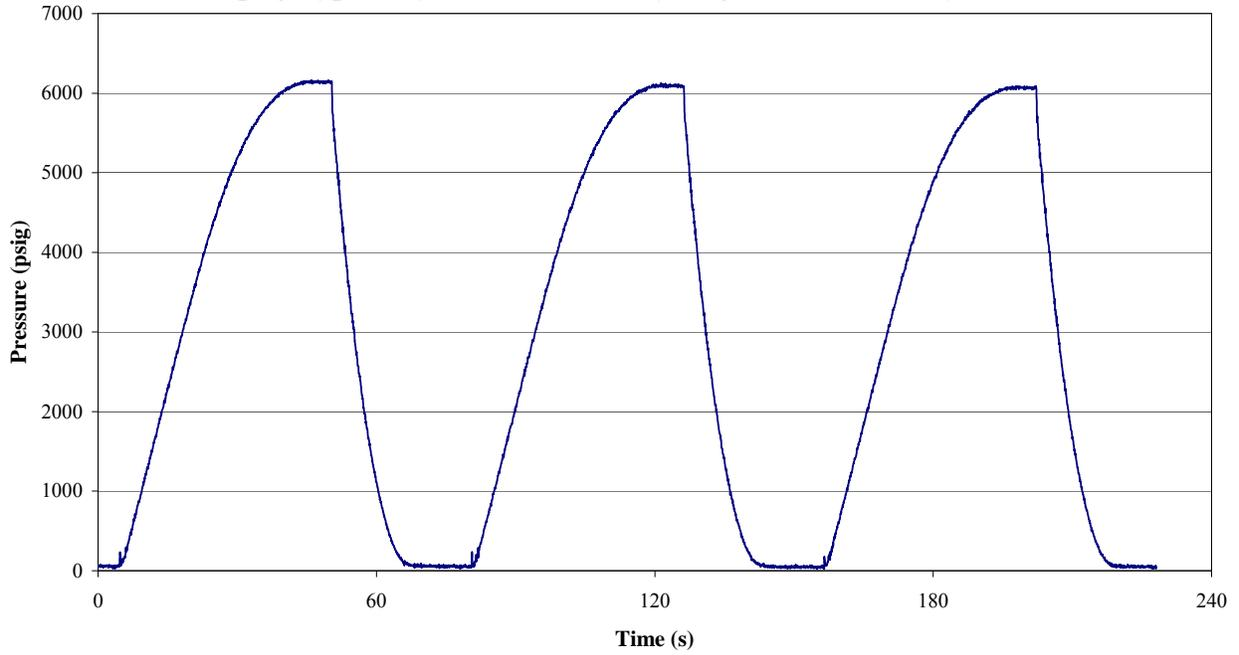
**5,000-psig Type-3 Cylinder Pressure Cycling Test At 125% Cycle Count of 3300**
