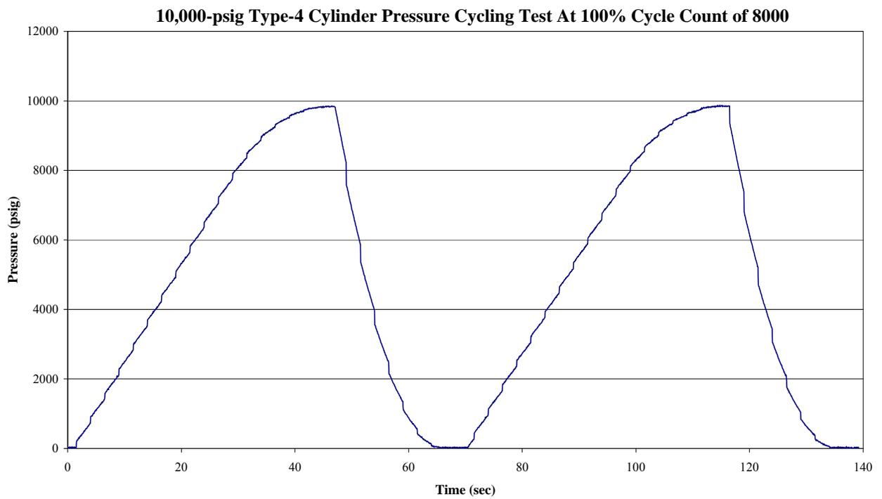
**Figure B-5. 10,000-psig Type 4 Cylinder Pressure Cycling Test Data (1 of 1).**
