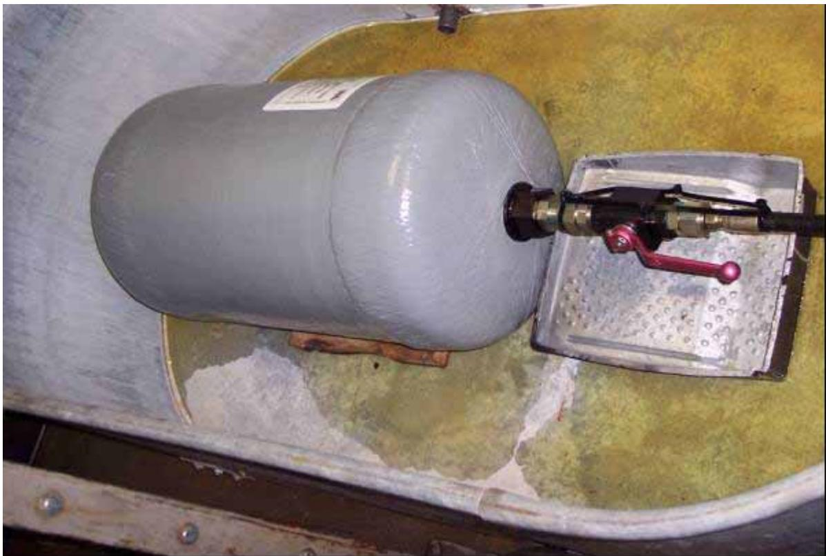
**Figure C-6. 5,000-psi Type 4 Cylinder Setup for Pressure Cycling Tests.**
