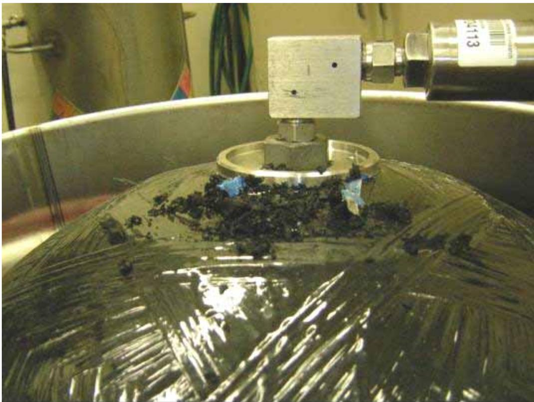
**Figure C-8. Damage at Fitting on 10,000-psig Cylinder Following Pressure Cycling Tests.**
