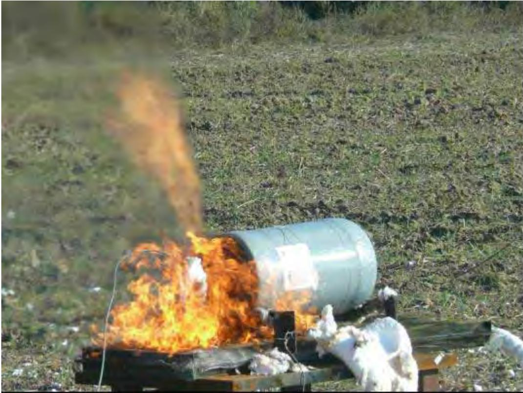
**Figure C-3. View of 5,000-psi Type 4 Cylinder Venting.**
