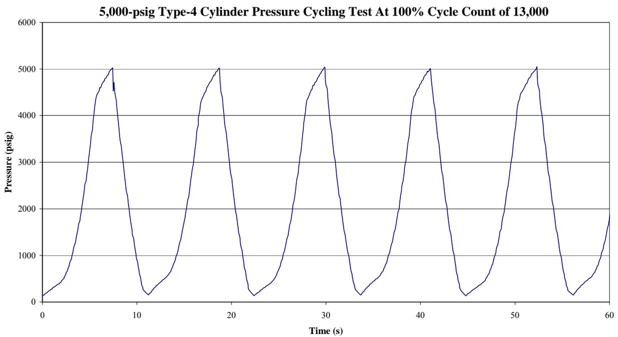
**Figure B-3. 5,000-psig Type 4 Cylinder Pressure Cycling Test Data (1 of 2).**
