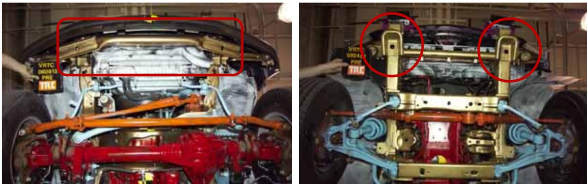
Figure 4-1: Different Type of Secondary Energy Absorbing Structure (SEAS)
