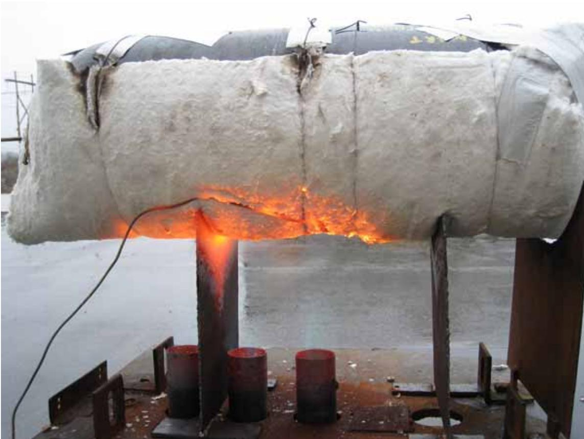
Figure 13 – Localized fire test of SuperWool 607 Plus blanket
