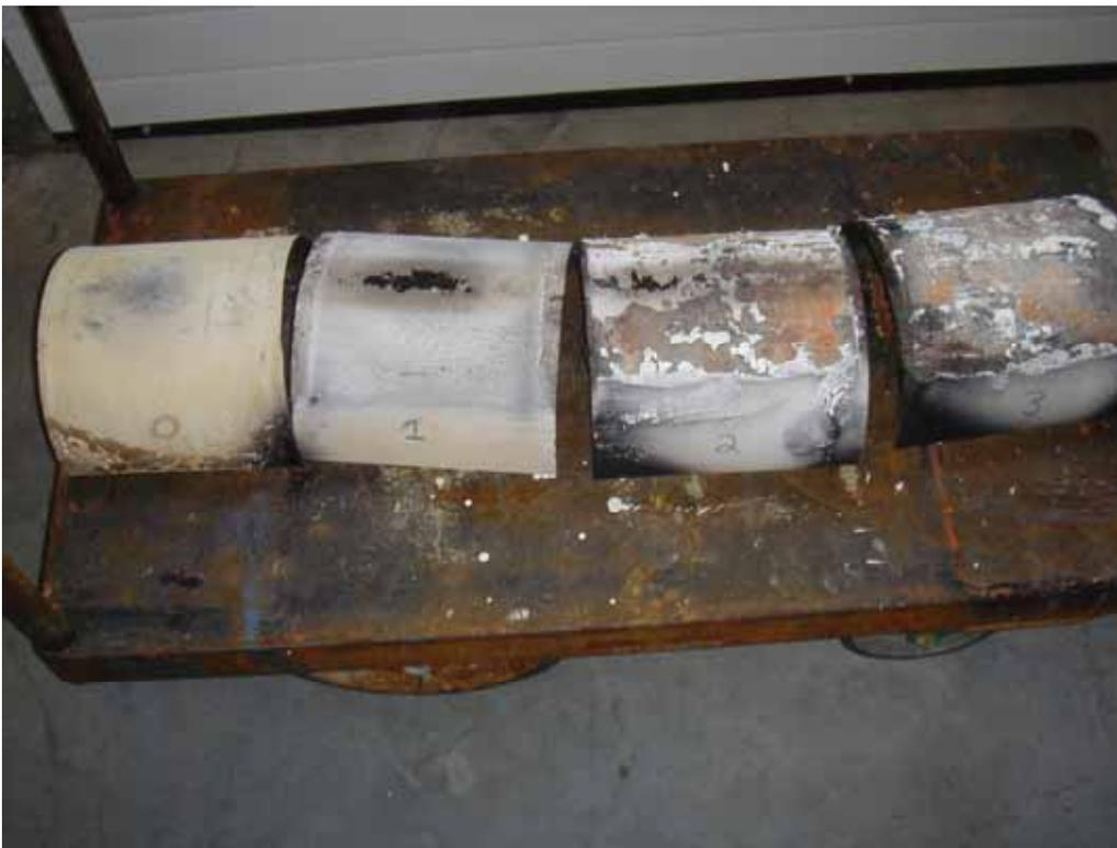
Figure 2 – Results of fire testing on PyroCide II paint coating of various thicknesses (#0 = bare steel, #3 = 3 coats of paint).
