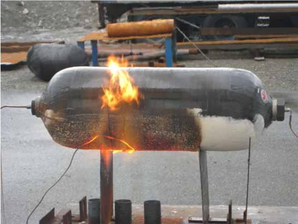
Figure 4 – Performance of PyroCide II intumescent paint coating on bottom of carbon fiber composite tank during exposure to 3-burner fire test.
