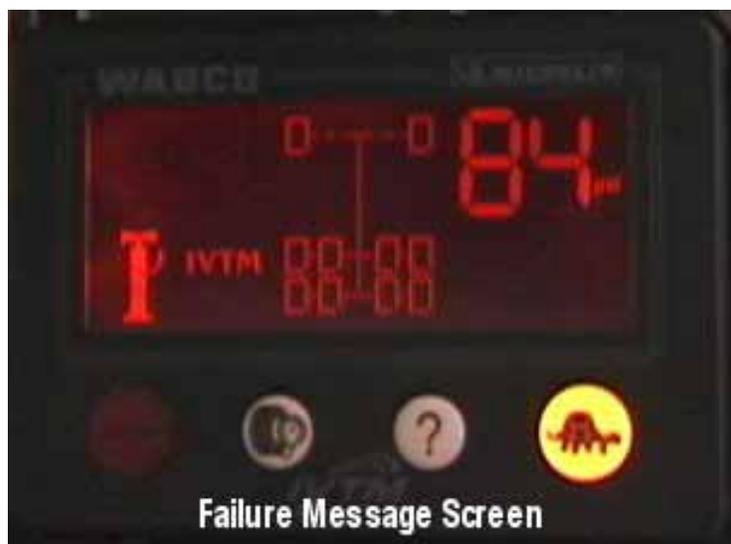
Figure 2.31. Information Screen Showing Tire Pump Signifying that a Tire Needs to be Re-Inflated
