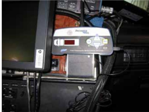
Figure 2.12. PressurePro Driver Display Mounted in the Truck
