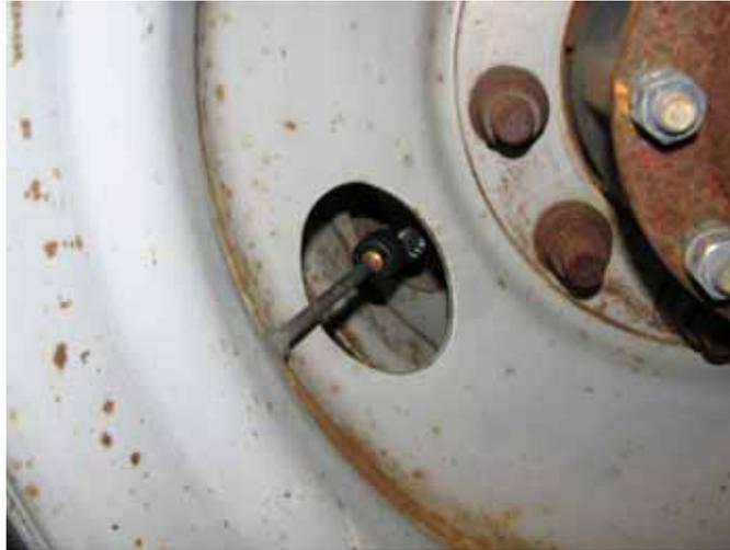
**Figure 2.14. Side View of Two PressurePro Sensors Mounted on Dual Steel Wheels
