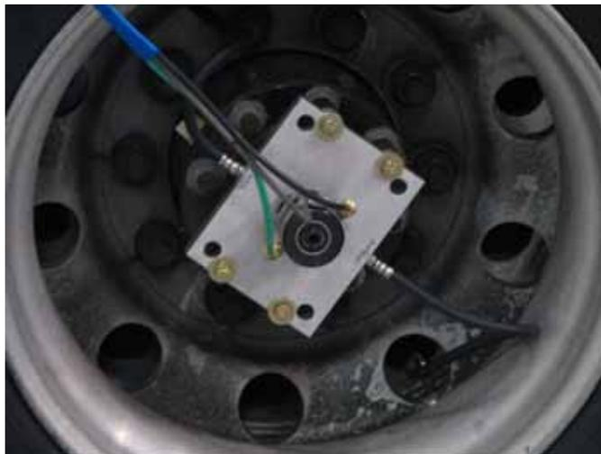
**Figure B.6. Two Port Rotary Union on Drive Wheel**
