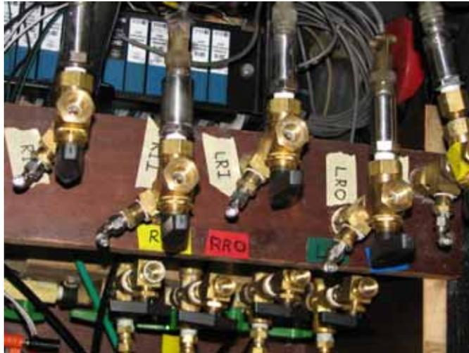
Figure B.1. Pressure Transducers and Signal Conditioners
