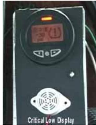
**Figure 2.21. Critical Low-Pressure Warning**
