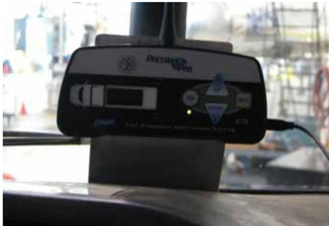
**Figure 2.37. PressurePro Driver Display Showing “Ready Mode” on Screen; Only the Green Light is Visible in This Mode When Not Hand Selecting Pressures**
