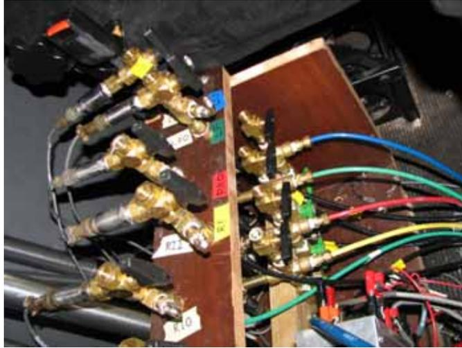
**Figure B.5. Close-up View of Pressure Control Manifold**
