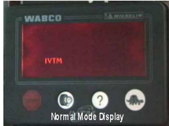
Figure 2.27. Display in Ready Mode – for Normal Operation
