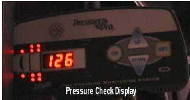
Figure 2.34. Current Pressure is 126 psi in Left Front Steer Tire
