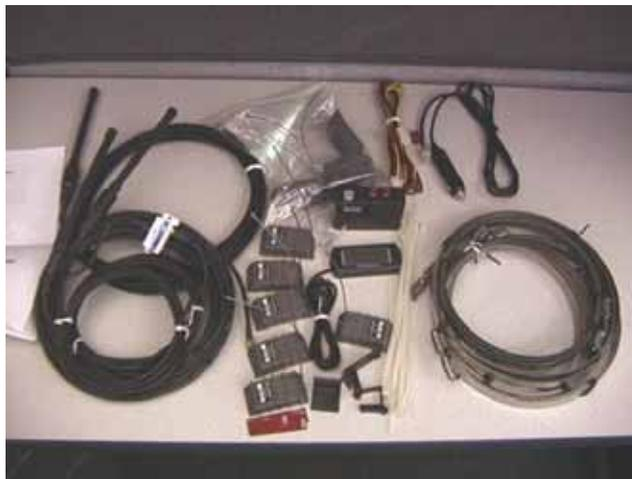
**Figure 2.7. Components Kit for Tire-SafeGuard 10-Tire Rim-Mount TPMS**
