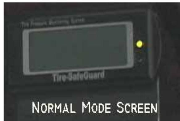
**Figure 2.23. Display in “Run” Mode Immediately After Power-up Cycle**
