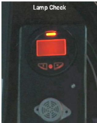
**Figure 2.17. Power-Up Lamp Check**
