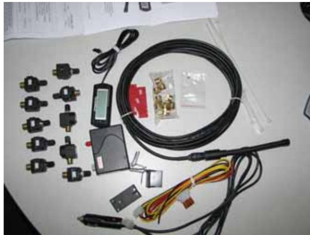
**Figure 2.8. Components Kit for Tire-SafeGuard Flow-Through 10-Tire System**
