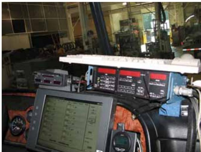
**Figure C.2. SmartWave Display (Lower-Right) Along with CDAS Screen and Speed and Distance Measuring Equipment**
