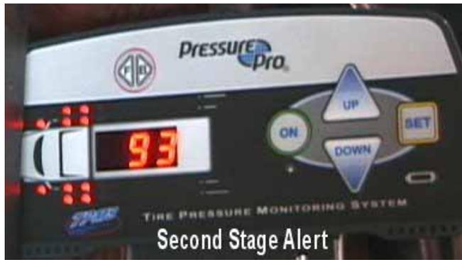
**Figure 2.36. Left Front Steer Tire Channel Is Warning of a Second Stage Low-Pressure Detection**
