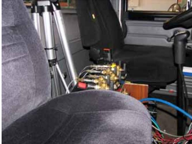
**Figure B.3. Observer's View of Tire Pressure Control Manifold**
