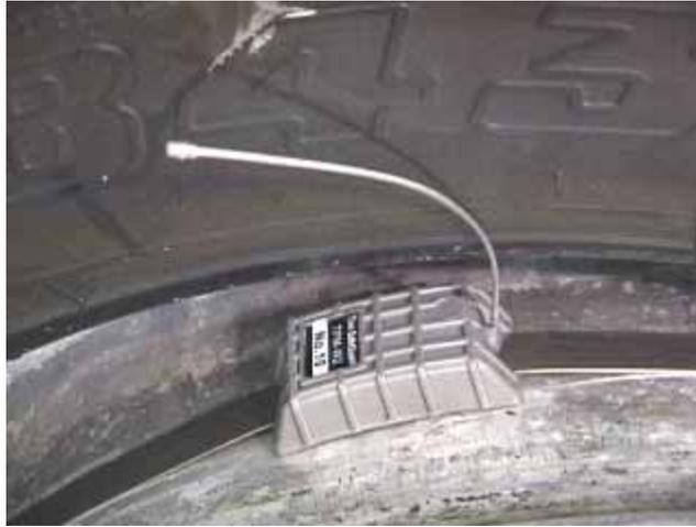
**Figure 2.4. Rim-Mounted Tire-SafeGuard Sensor with High-Gain Antenna
