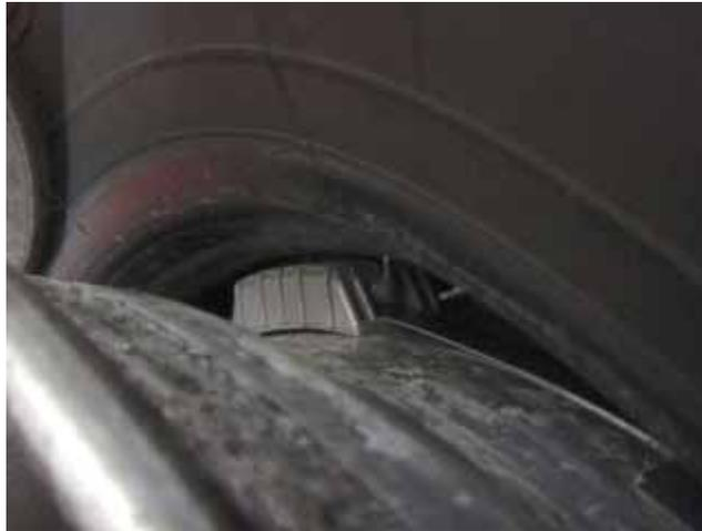
**Figure 2.5. Rim-Mount Tire-SafeGuard with Antenna Pushed Inside Tire
