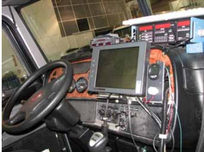
**Figure C.3. Right-Seat Observer's View of Instrumentation Displays**
