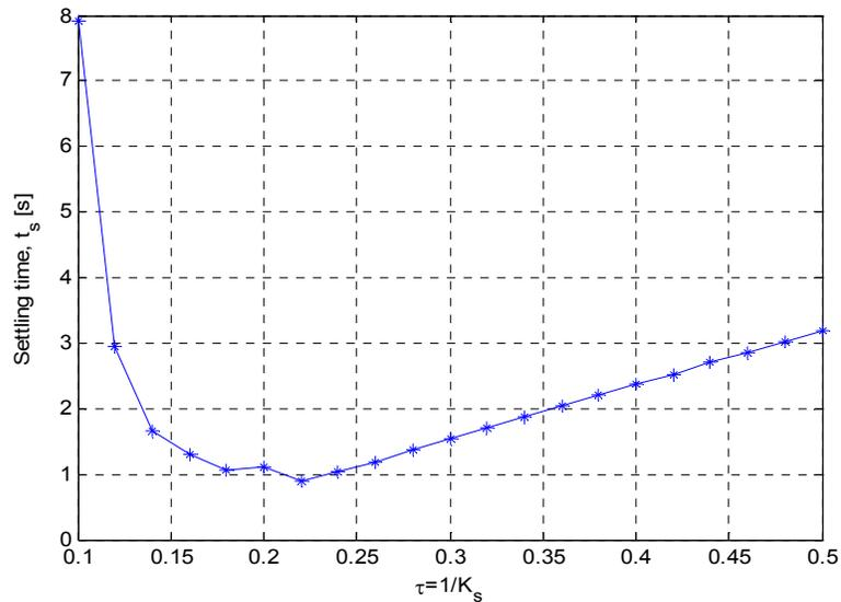
**Figure C.4. Settling Time for Different Control Gains ( $T_s = 0.05$ )**
