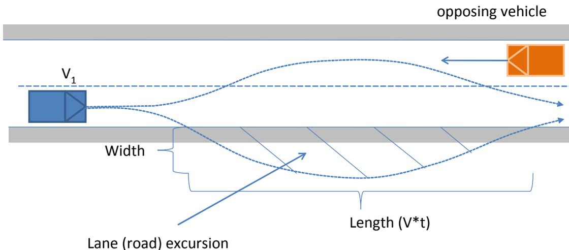
**Figure 7.6. Crash Risk Related to Trajectory Output From Simulation.**
