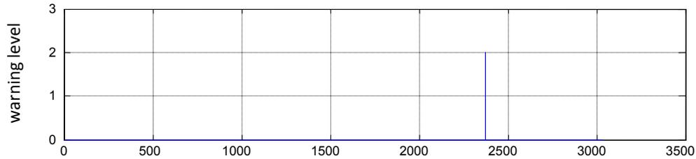
**Figure D.2. Time History of DAC Warning Signal** (0 = off, 1 = left side warning, 2 = right side warning)
