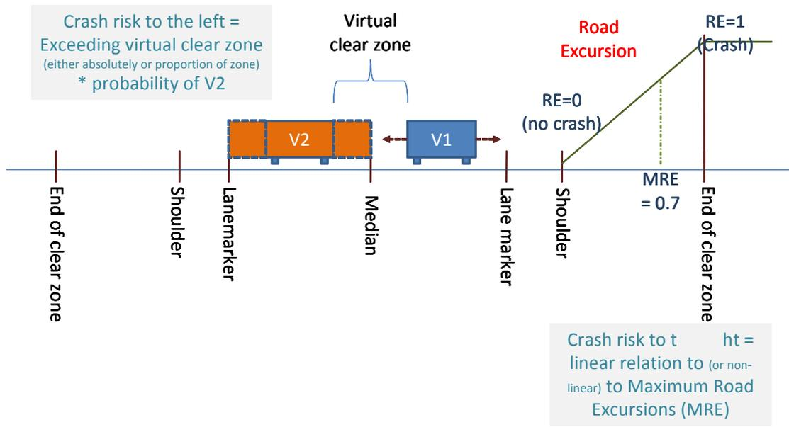
**Figure 7.7. Crash Metric Definition as a Function of Maximum Road Excursion** (V1 denotes subject vehicle, V2 a principal other vehicle; MRE corresponds to the edge of the clear zone, and crash probability does not increase beyond this point).
