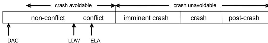
**Figure I: NHTSA Crash Phase Timing Diagram**
