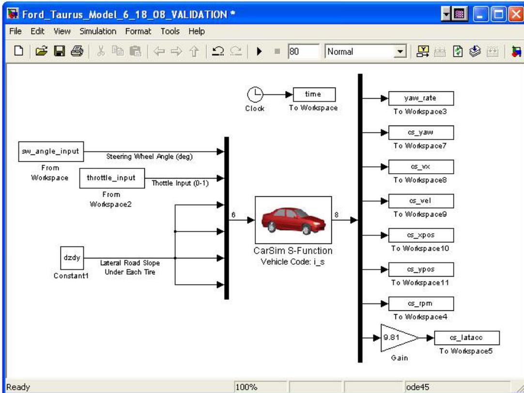
Figure 6.4. Simulink Diagram Used During CarSim Vehicle Model Validation
