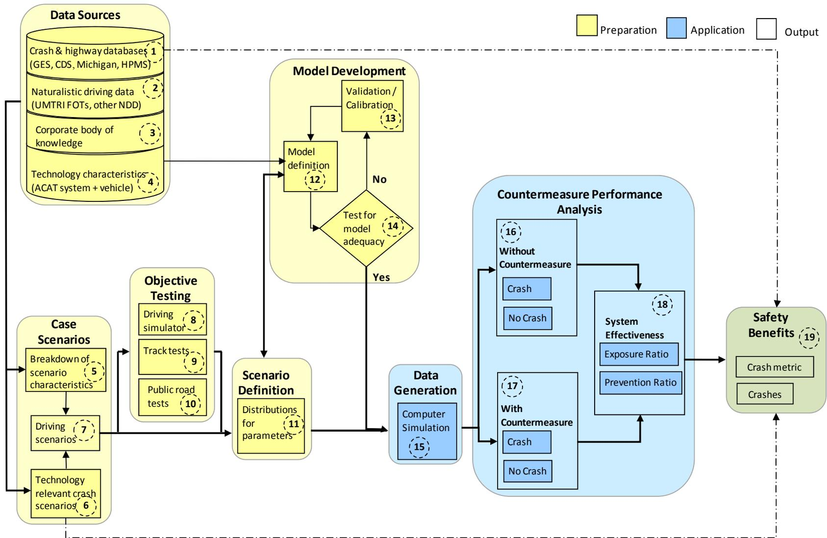
Figure 2.1. Overview of the SIM Components
