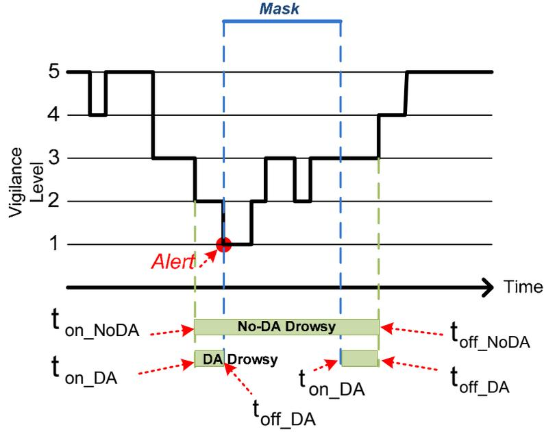
Figure D.3. DAC Exposure Effect: Estimated Reduction in “Drowsy Driving Time”
