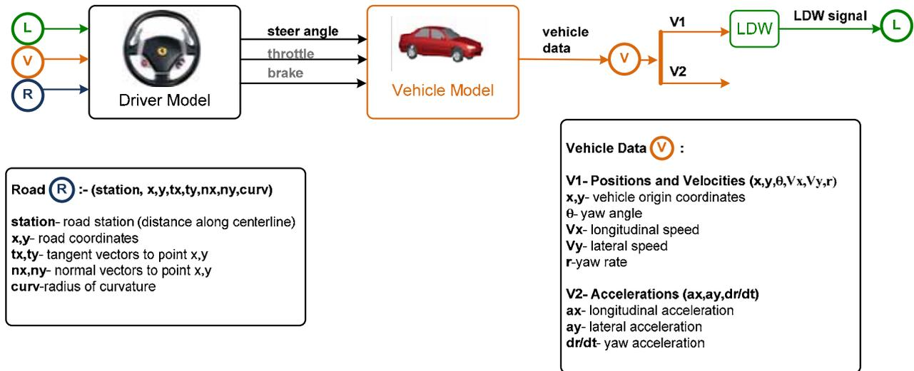
Figure 6.1. Architecture of the Coupled Vehicle-Highway-Driver Model
