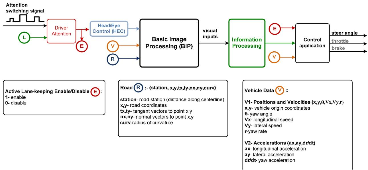
Figure 6.18. Driver Model: Overall Architecture
