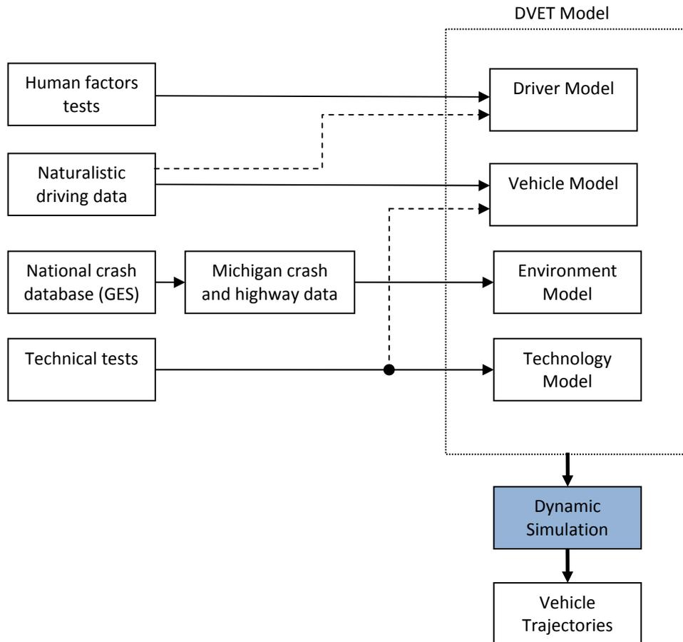
Figure 3.1. Major Data Sources used to Support Batch Simulations
