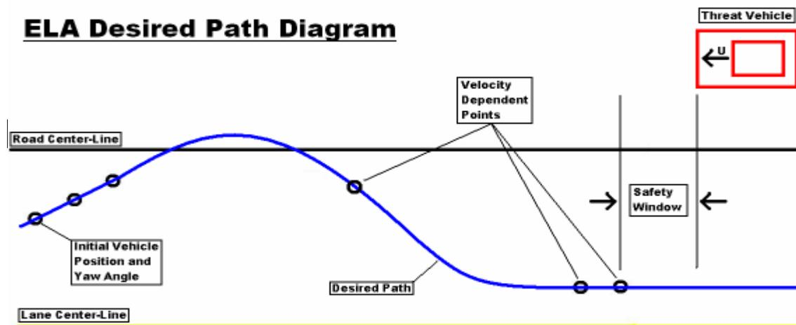
Figure D.4. Schematic of ELA Operation
