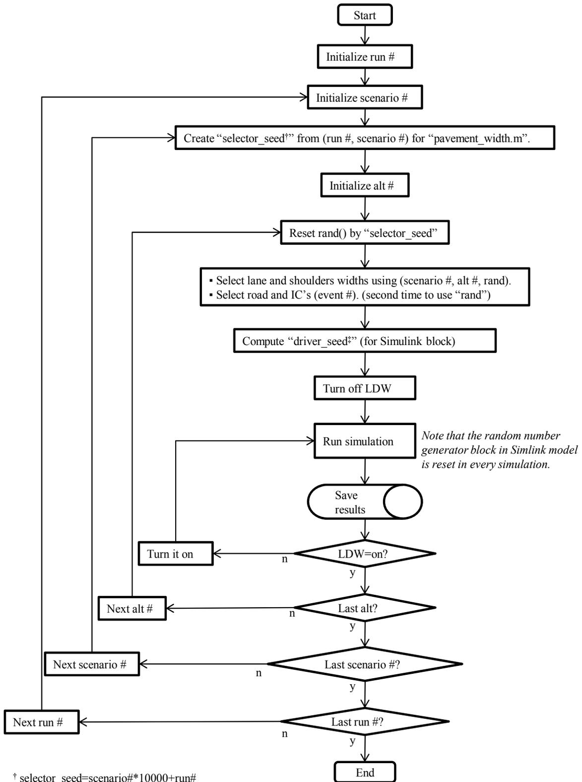
Figure 7.4. Flow Chart for Batch Run Control (# denotes run counter or identifier, and IC denotes initial condition).
