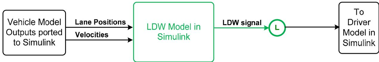
Figure 6.12. Architecture of the LDW Model
