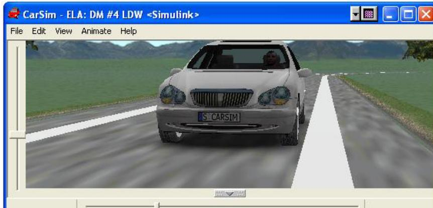
Figure 6.16. Vehicle Location when the First Lane Departure is Detected (2.04 sec)
