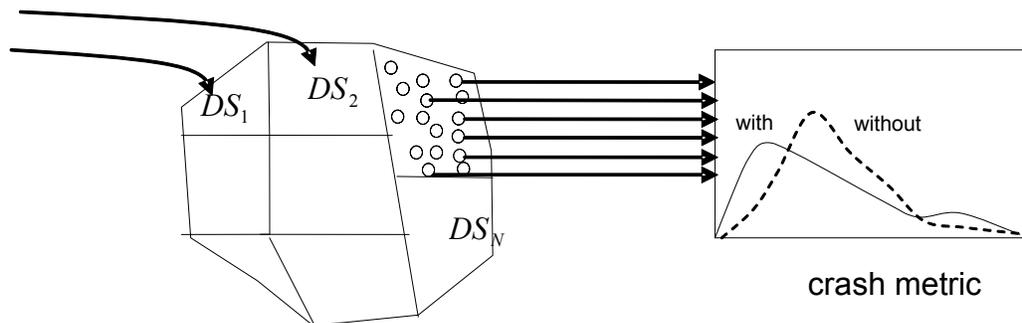
**Figure 4.1. Driving Scenario Resolution for Monte Carlo Simulation - With and Without the Specific Safety Technology Being Evaluated.**
