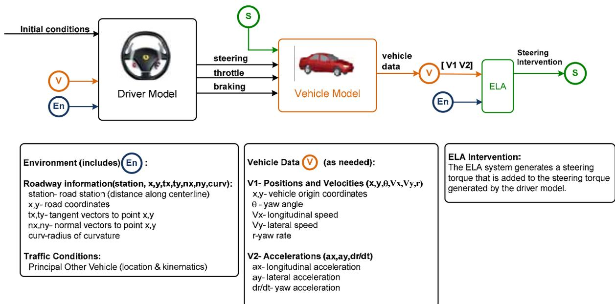
Figure D.5. ELA Functionality Added to the DVET Model
