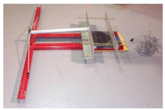
Figure 6. Apparatus for Recording Steering Wheel Movement
