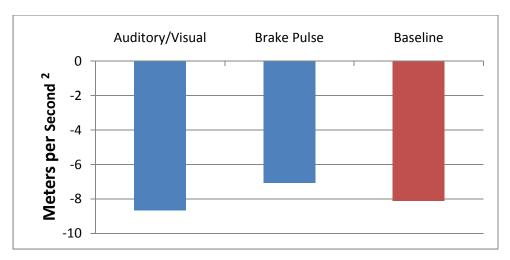
Figure 14. Peak deceleration while braking for FCW systems
