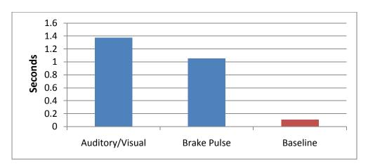
Figure 15. Minimum time to collision for FCW systems
