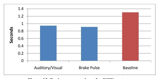
Figure 13. Brake response times for FCW systems
