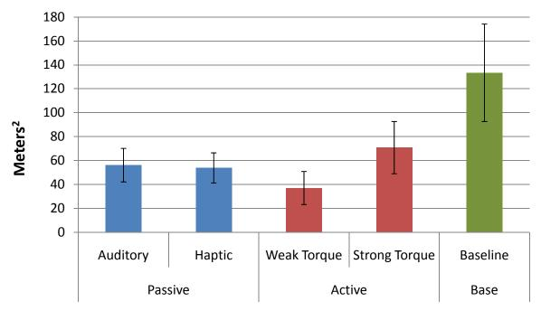
Figure 3. Area of lane exceedance as a function of LDW warning condition
