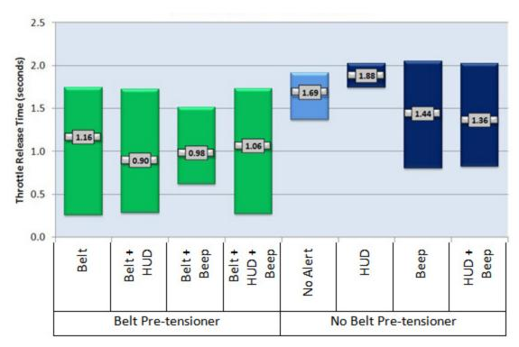
Figure 12. Throttle release times for FCW systems
