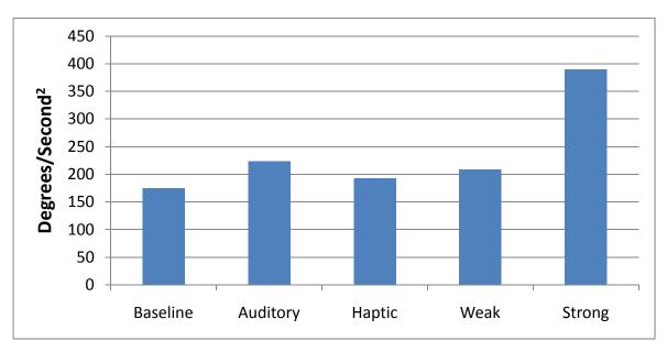
Figure 11. Peak steering acceleration in a false alarm situation
