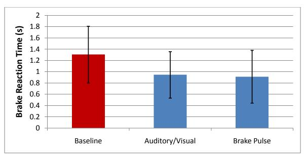
Figure 4. Elapsed time between initiation of FCW alert and brake pedal pressed (with standard error bars)
