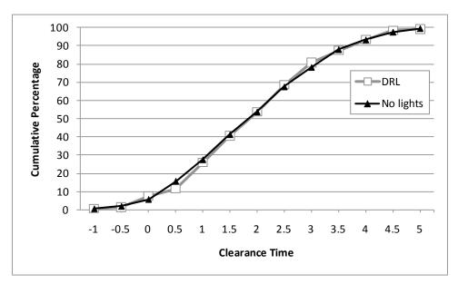
Figure 9. Cumulative Distributions of Clearance Times for Vehicles Turning in Front of Approaching Vehicles with DRL or No Lights (Boyds Site)
