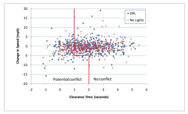
Figure 11. Potential Conflicts and Non-Conflicts for 778 Left-Turning Vehicles Based on Clearance Time and Changes in the Approaching Vehicle's Speed (Boyds Site)
