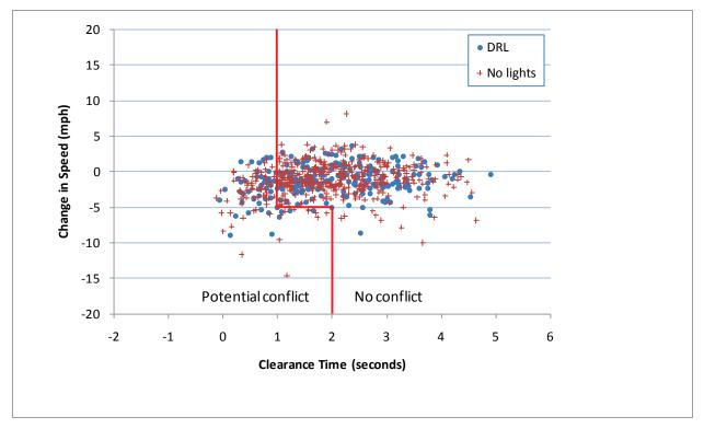
Figure 12. Potential Conflicts and Non-Conflicts for 661 Left-Turning Vehicles Based on Clearance Time and Changes in the Approaching Vehicle's Speed (Burtonsville Site)
