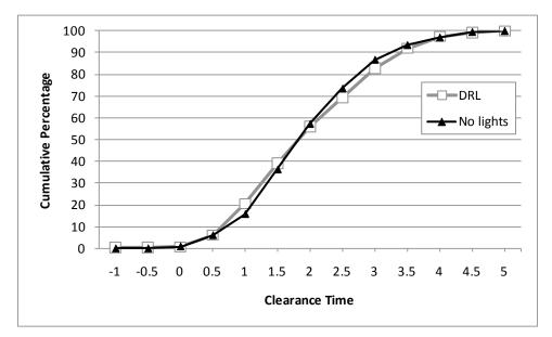
Figure 10. Cumulative Distributions of Clearance Times for Vehicles Turning in Front of Approaching Vehicles with DRL or No Lights (Burtonsville Site)
