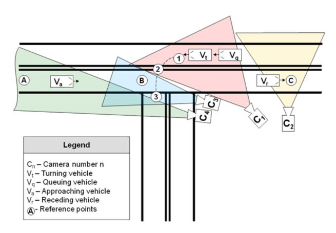
Figure 5. Simplified Plan View of an Intersection Showing Approximate Camera Coverage Zones and Reference Points
