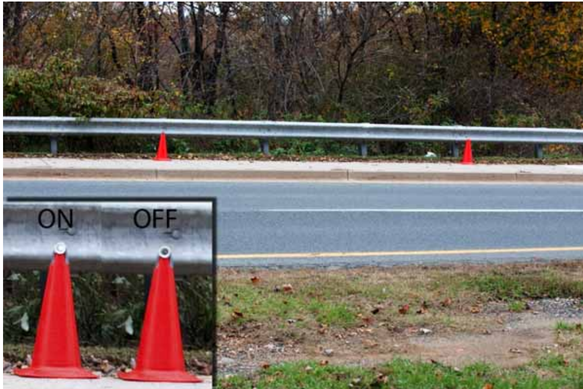
Figure 3. Participants' View of Traffic Cones with Detailed Views (Inset) of the Secondary Task Signal Light in ON and OFF States
