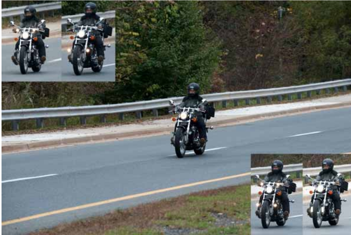
Figure 6. Motorcycle Rider Passing Study Site with Various Sets of Auxiliary Lamps Illuminated
