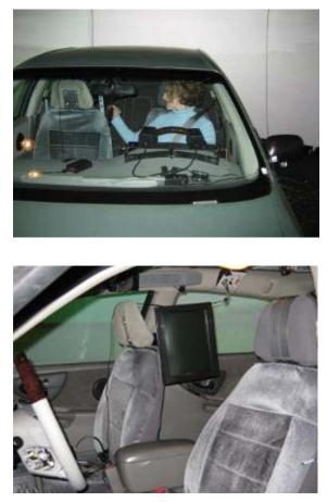
Figure G-2 Reaching task hardware setup; Top: head and body orientation; Bottom: display location and orientation.
