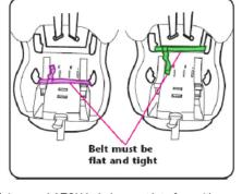
Make sure LATCH belt does not interfere with the harness or the crotch strap.
