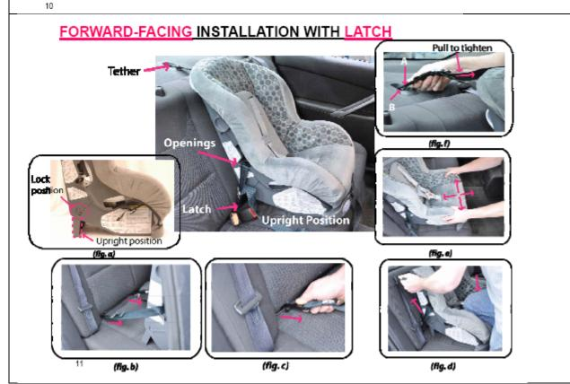
Revised text (top) and photo (bottom) ComfortSport LATCH installation. Revised text includes simplified text and color-coded headings.
