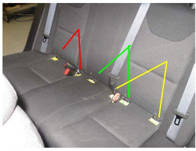
Figure 2. Locations of 2006 Pontiac G6 rear seat lower anchorages and seatbelt buckles.
