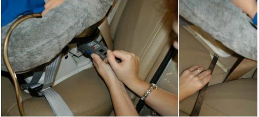
Figure 10. Measuring amount of CRS lateral displacement under applied load.
