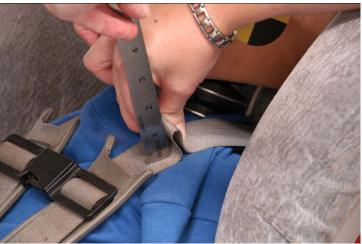
Figure 8. Measuring amount of harness slack.
