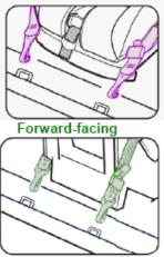
Pull connectors to make sure they are really attached to the vehicle anchorages.
