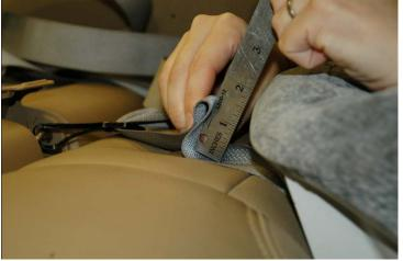
Figure 9. Measuring amount of tether slack.
