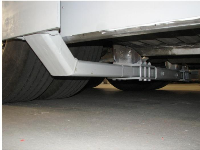
AP Figure 13. Photograph of the tube center joiner
