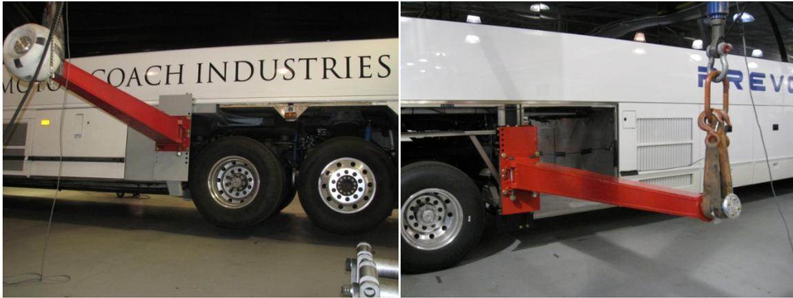
AP Figure 30. Photographs of the motorcoach outrigger and mount static load testing. Left: MCI motorcoach. Right: Prevost motorcoach.
