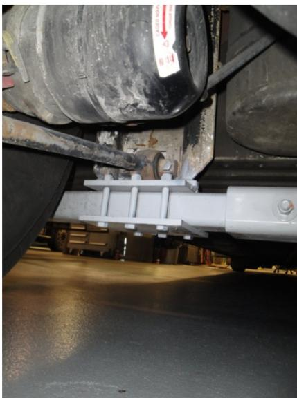
AP Figure 11. Photograph of the under-slung (lower) mounting frame installed on the MCI motorcoach.
