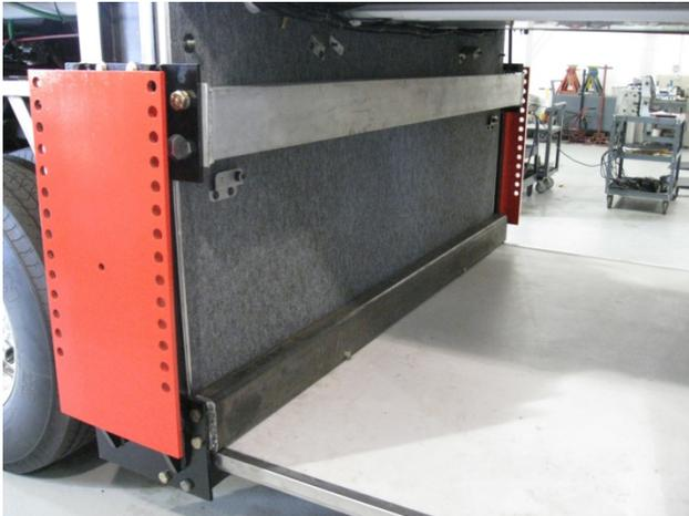
AP Figure 19. Photograph of PrevoSt lower 6 inch x 3 inch steel tube and the 6 inch x 4 inch aluminum rectangular tube.
