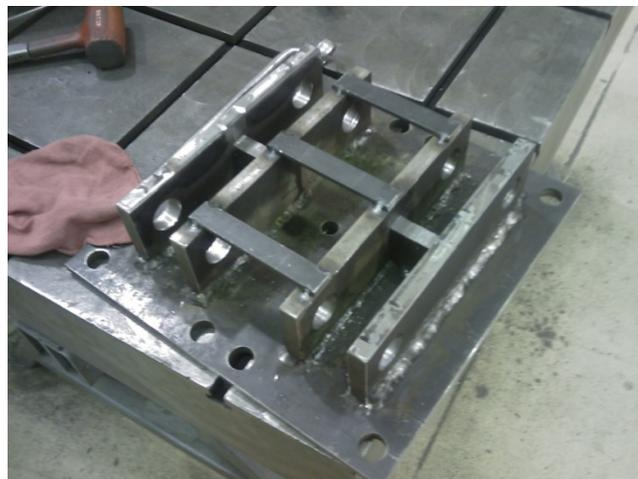
AP Figure 9. Photograph of the outrigger mounting plate during fabrication.
