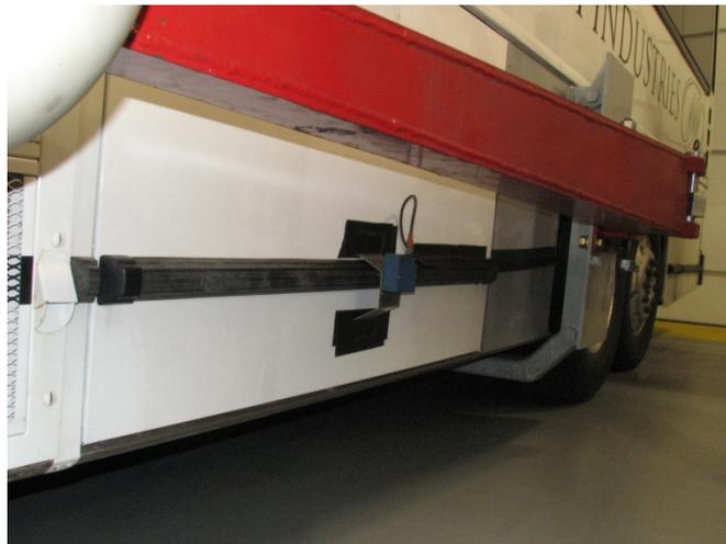
AP Figure 6. Completed outrigger assembly installed on a motorcoach.
