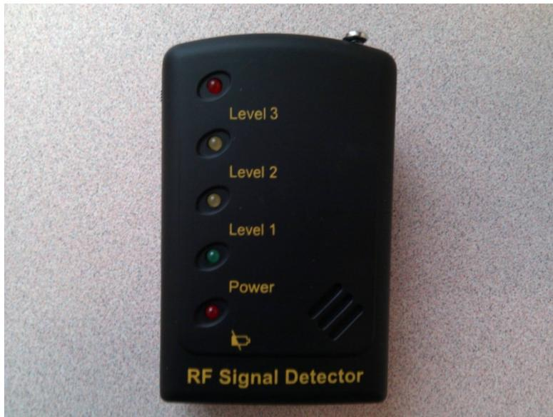
**Picture 6: The SureSafe SH-055SRV RF signal detector**
