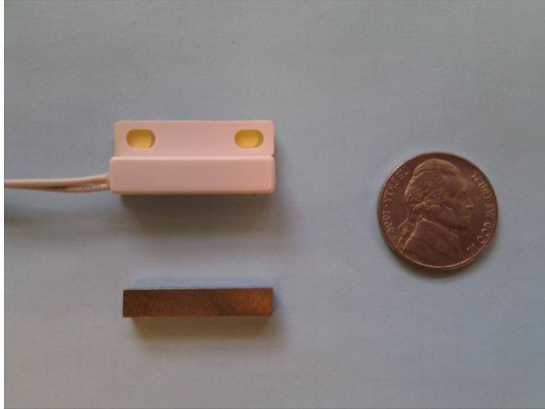
**Picture 2: Honeywell reed switch and magnet**
