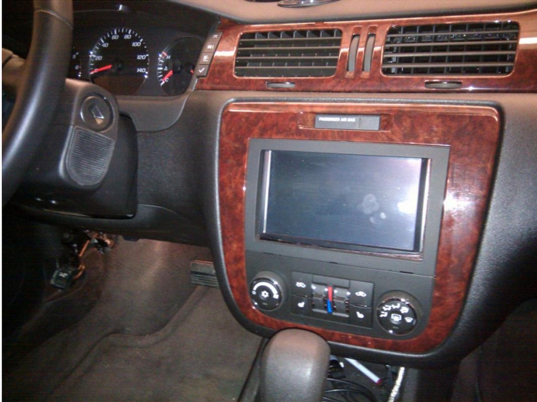
Figure 3-1. STC demonstration vehicle visual feedback display integrated into the vehicle.
