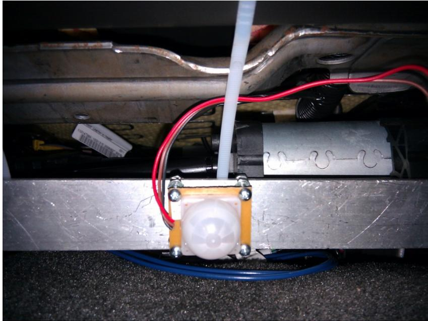
**Picture 3: Passive infrared sensor mounted near the bottom of the passenger seat in a 2009 Chevrolet Impala.**
