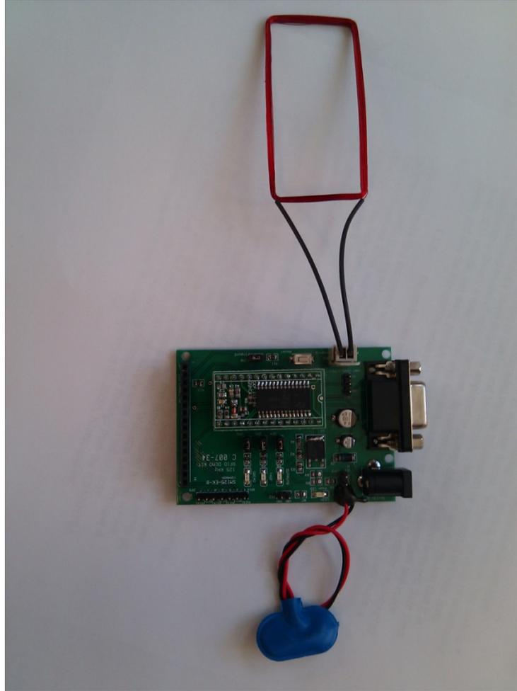
**Picture 1: Low frequency RFID transceiver with external antenna (top) and battery pack connector (bottom)**
