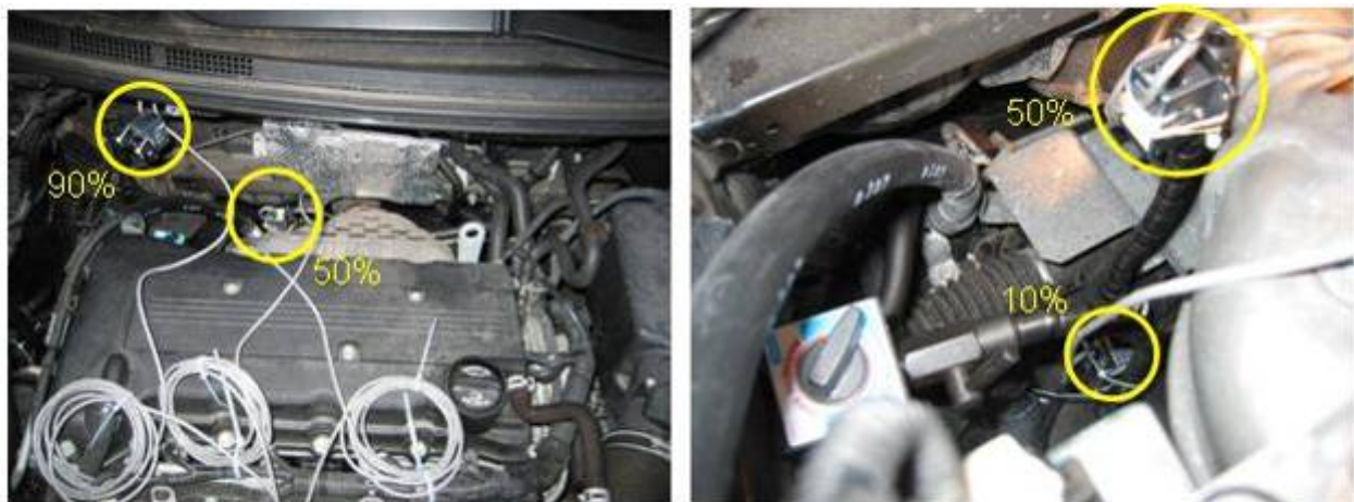
Figure I-6. Positioning of engine compartment sensor suite at 10 percent, 50 percent, and 90 percent heights.
