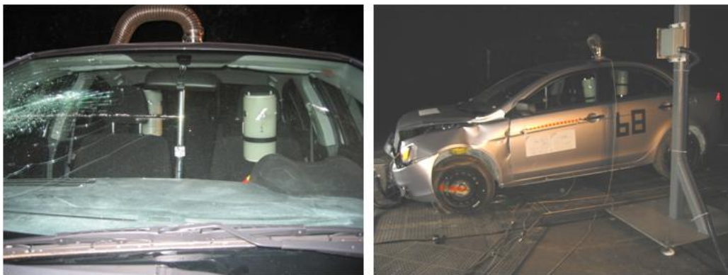
Figure III-18. Heat flux gauges and pressure transducers mounted in plastic cylinders at driver's and rear passenger's head locations and exterior (first responder) test stand (right) in Test 68.
