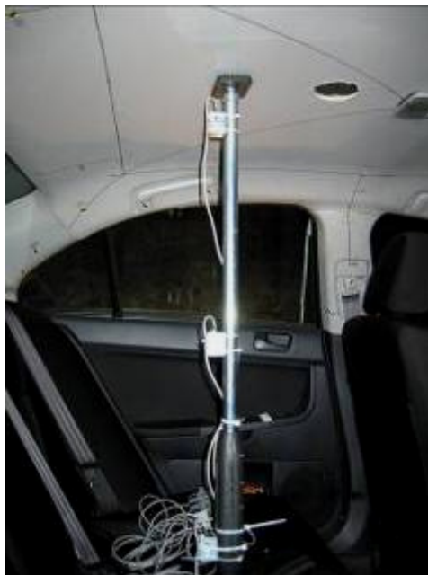
Figure I-4. Positioning of rear-passenger compartment sensor suite at 10 percent, 50 percent, and 90 percent heights.
