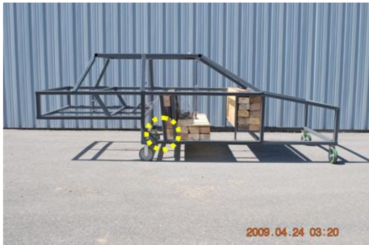
Figure II-12. Hydrogen leak originating in rear passenger compartment, flowing to rear of ACS.
