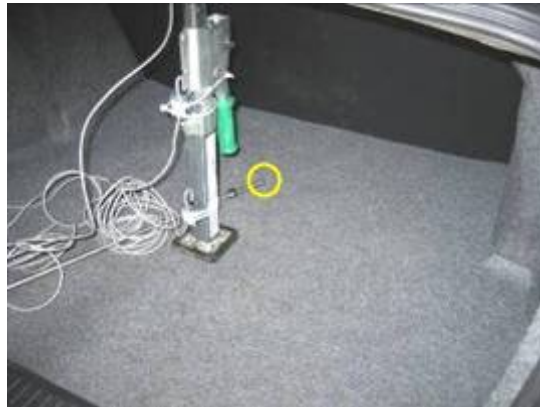
Figure I-7. Hydrogen leak originating in the trunk.
