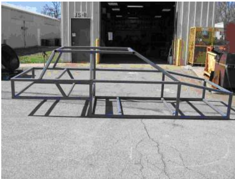
Figure II-3. Welded framework of ACS.
