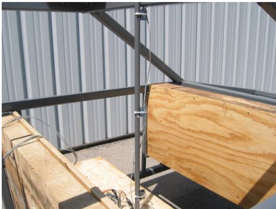
Figure II-10. Position of front passenger compartment sensor suite at 10 percent, 50 percent, and 90 percent height.
