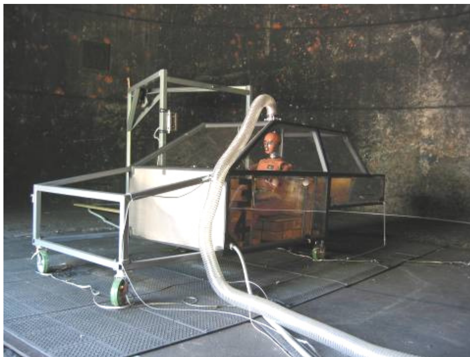
Figure II-1. ACS and manikin in JS-10 blast chamber for hydrogen ignition testing.
