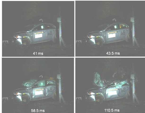
Figure III-19. High-speed imagery stills for showing first observed light (41 msec), rear headliner motion (43.5 msec), glass fracture/door bulge (58.5 msec), and glass ejection (110.5 msec) in Test 68.
