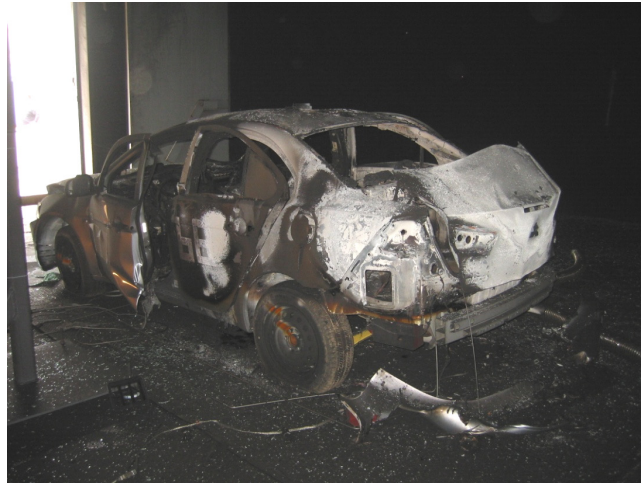
Figure III-40. Damage to front-impact vehicle after secondary fire burned to completion in Test 68.
