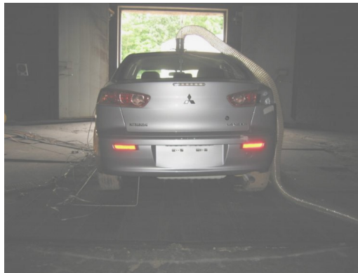
Figure III-1. JS-10 blast chamber used for indoor testing of hydrogen leaks into vehicles and ignitions.
