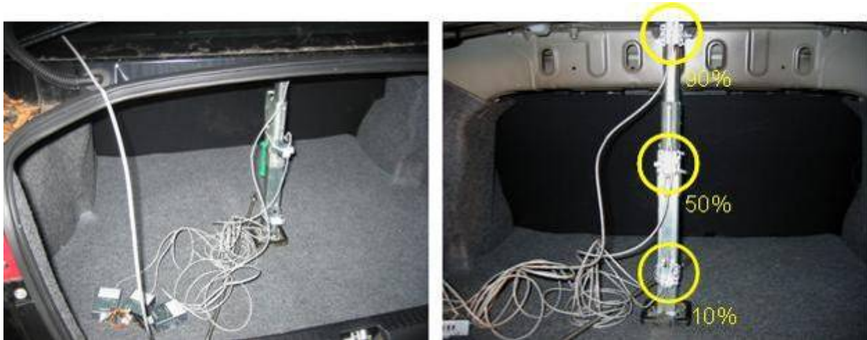
Figure I-3. Positioning of trunk compartment sensor suite at 10 percent, 50 percent, and 90 percent heights.
