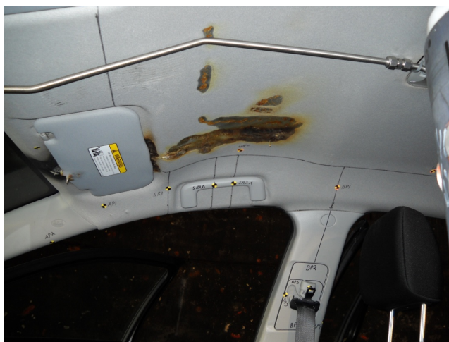
Figure III-42. Damage to headliner above front-passenger seat after secondary fire was extinguished in Test 83.
