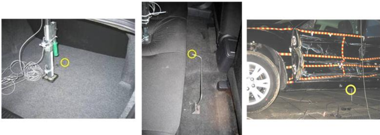
Figure III-5. Hydrogen leak locations in trunk floor (left), rear-passenger compartment floor (center), and underneath vehicle (right).
