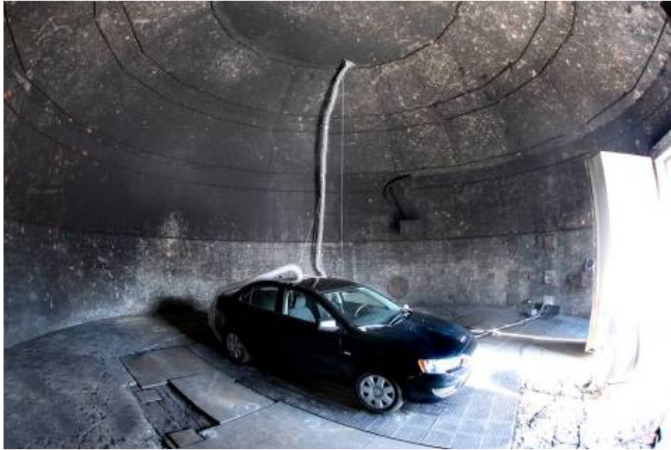
Figure I-1. JS-10 blast chamber/dome used for indoor testing of leak rates with car.
