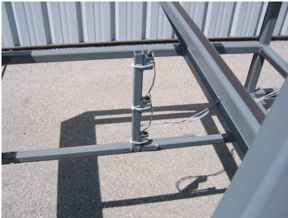
Figure II-8. Position of trunk compartment sensor suite at 10 percent, 50 percent, and 90 percent height.
