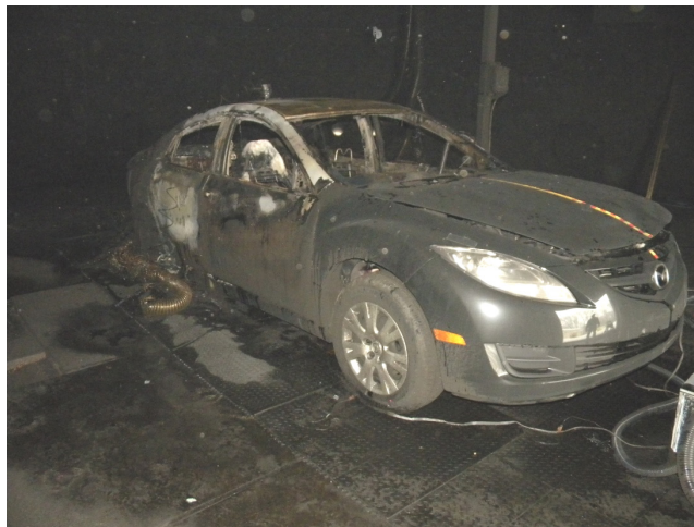
Figure III-44. Damage to front-impact vehicle after secondary fire burned to completion in Test 88.
