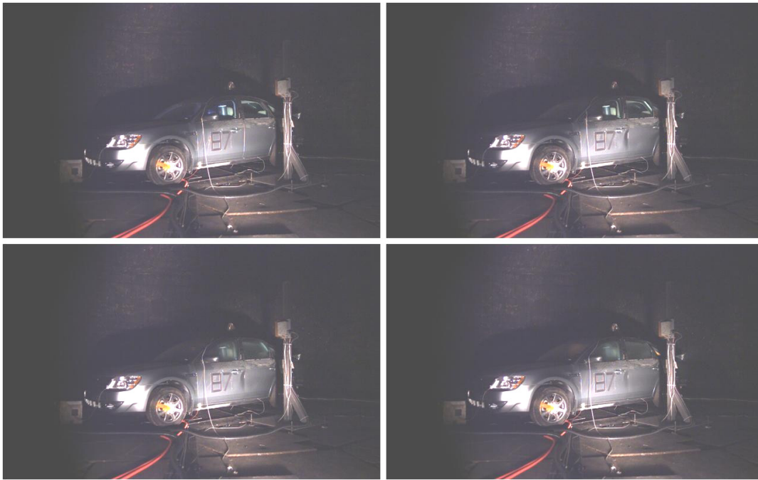
Figure III-31. High-speed imagery stills showing rear-impact vehicle at moment of first spark (top left at T = 0 sec); deformation of vehicle doors (top right at \sim T = 0.28 sec); noticeable smoke accumulation (bottom left at \sim T = 0.34 sec); and fireball inside vehicle (bottom right at \sim T = 0.61 sec) in Test 87.
