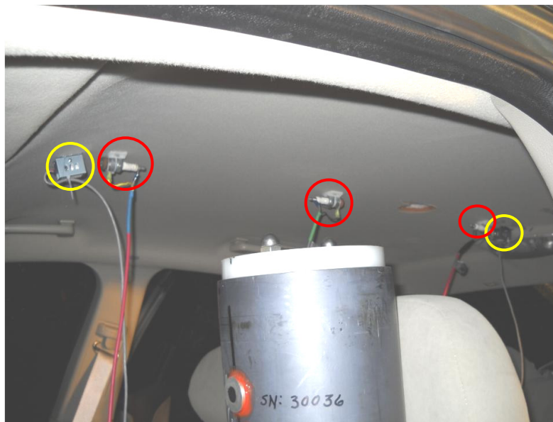
Figure III-7. Typical arrangement of hydrogen sensors (circled in yellow) and spark plugs (circled in red) deployed in ignition tests.
