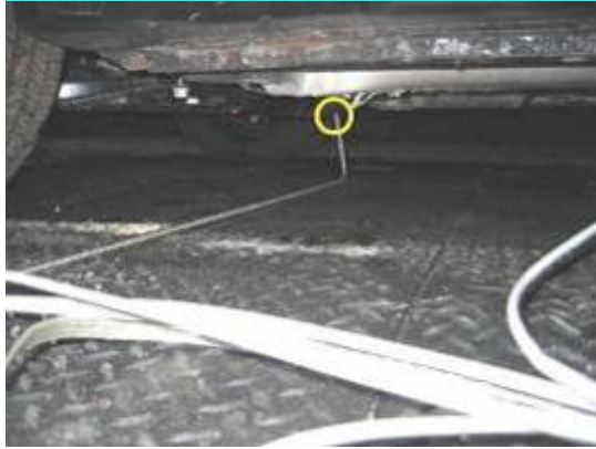
Figure I-13. Hydrogen leak slightly forward at firewall position underneath automobile.
