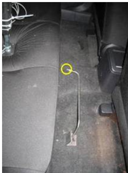
Figure I-8. Hydrogen leak originating from the rear passenger compartment.
