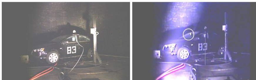
Figure III-41. Timeline of events after ignition (left) and secondary fire (right; circled) in Test 83.
