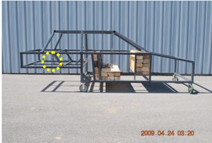
Figure II-11. Hydrogen leak originating in trunk, flow towards the front of the ACS.
