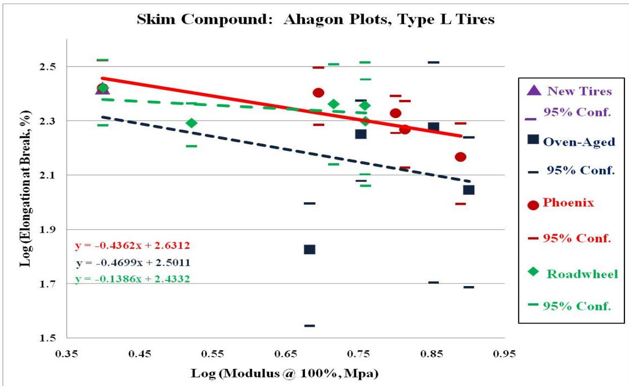
Figure 18. Ahagon Plot of Skim-Coat Compound for Type L Tires
