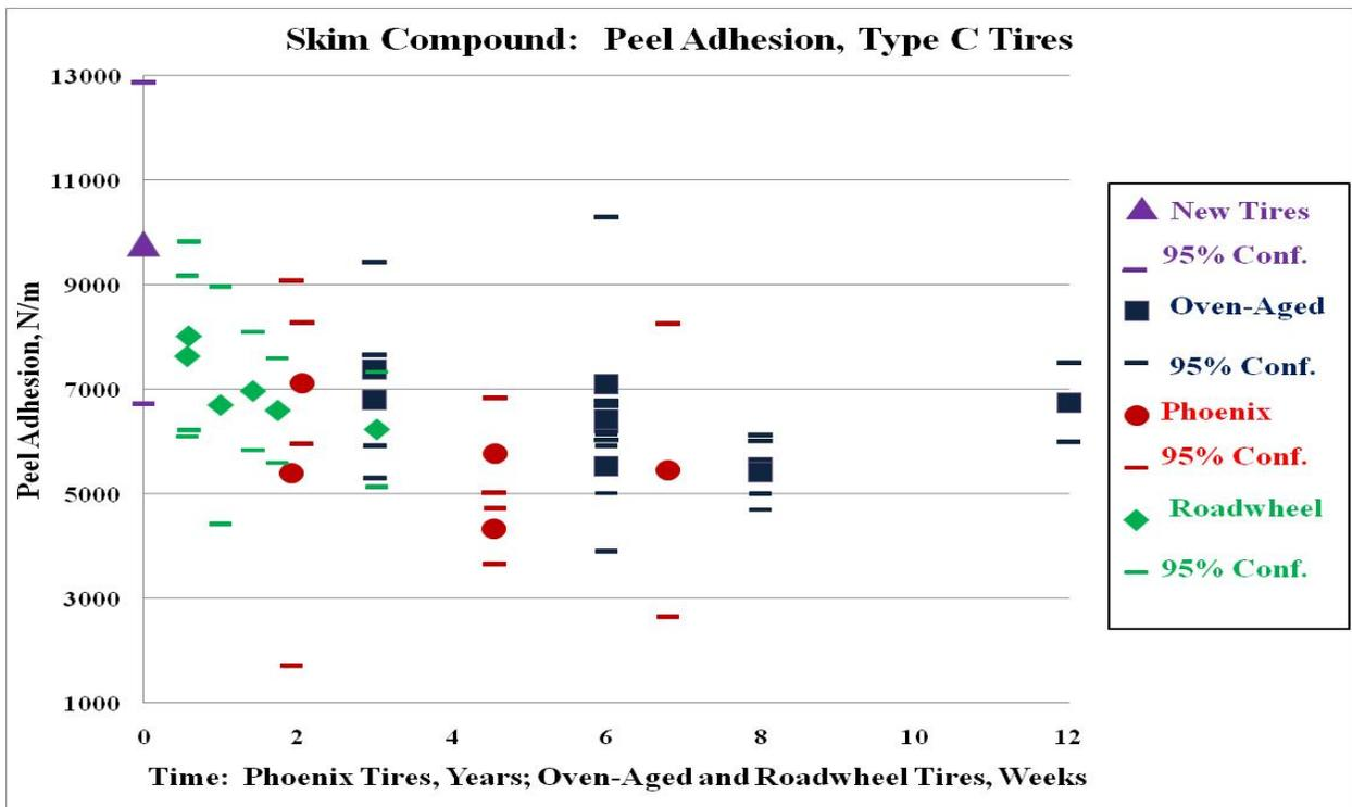
**Figure 32. Peel Adhesion Type C Tire Skim Compound After Oven-Aging, Roadwheel Testing or Service in Phoenix**
