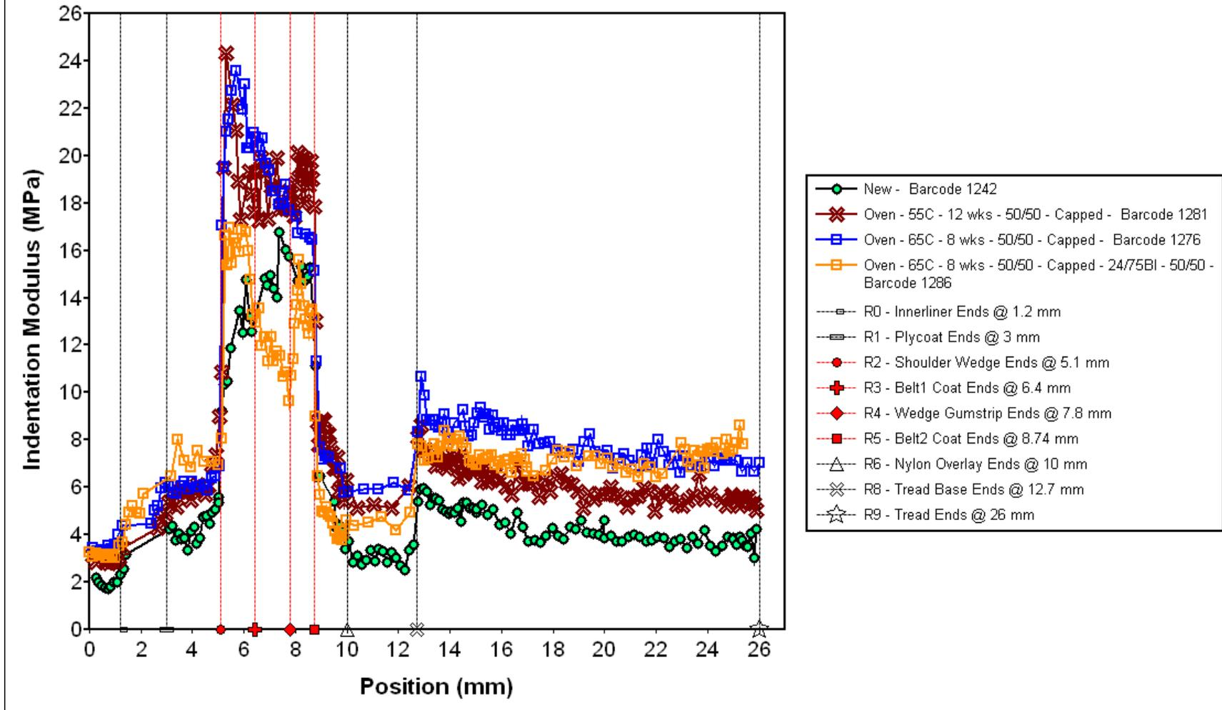
Note: Observe how the belt packages (5.1 mm to 8.74 mm) of the two type H tires that are oven aged without a roadwheel break-in harden relative to the new tire (1242), which is opposite of the trend observed in Phoenix-retrieved type H tires. Then observe how the 24-hour break-in at 75 mph prior to oven aging for tire 1286 produced results similar to the belt-package softening observed in Phoenix-retrieved tires.
