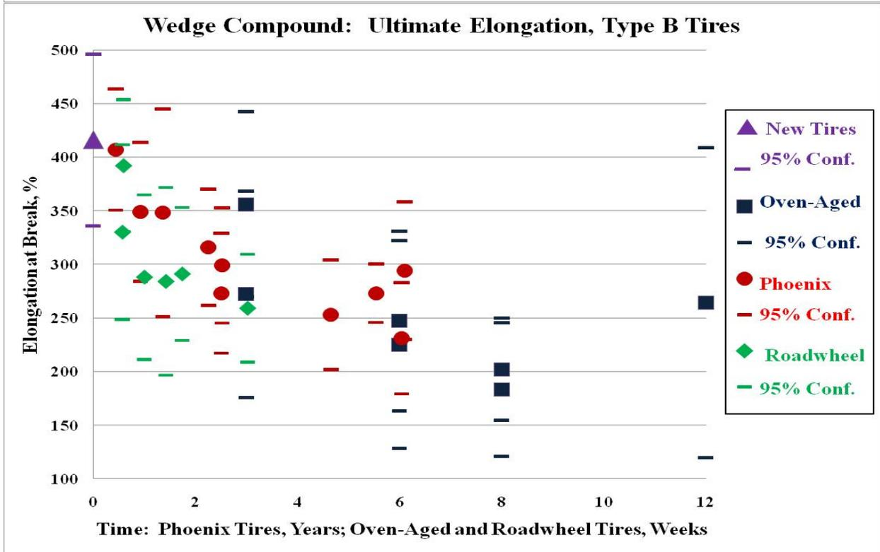
**Figure 19. Modulus @ 100% Strain and Ultimate Elongation for Wedge Compound of Type B Tires**
