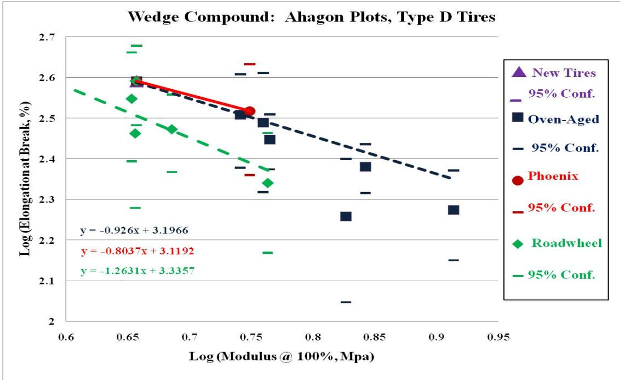
Figure 27. Ahagon Plot of Skim-Coat Compound for Type D Tires
