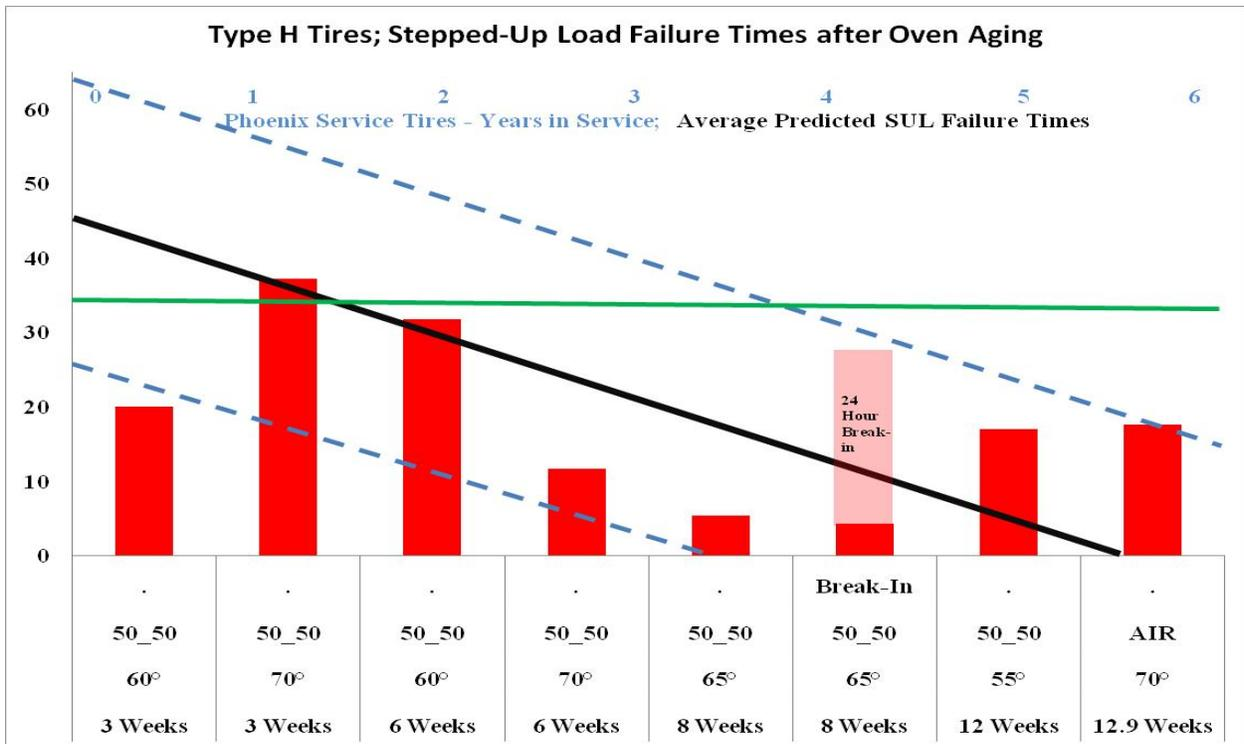
Figure 50. Stepped-up Load Test Failure Times: Oven-Aged Type H Tires Compared to Predicted Values for Tires With 1 to 6 Years of Service in Phoenix
