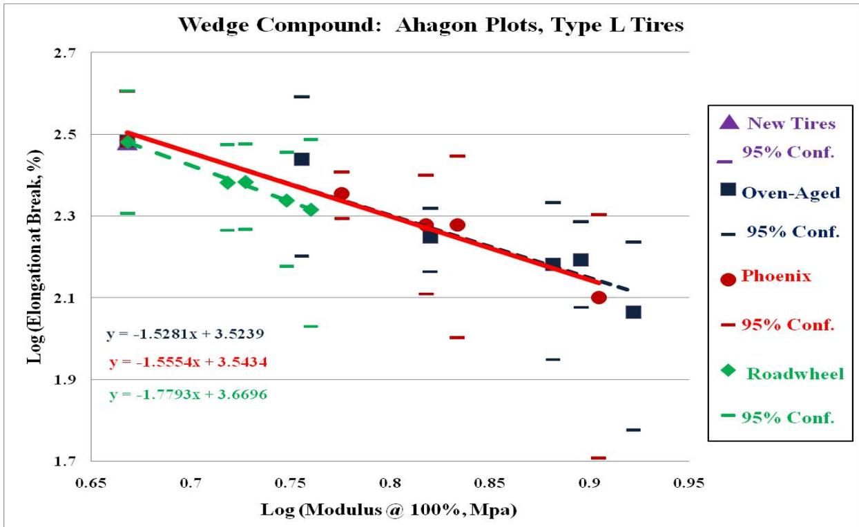
Figure 30. Ahagon Plot of Skim-Coat Compound for Type L Tires
