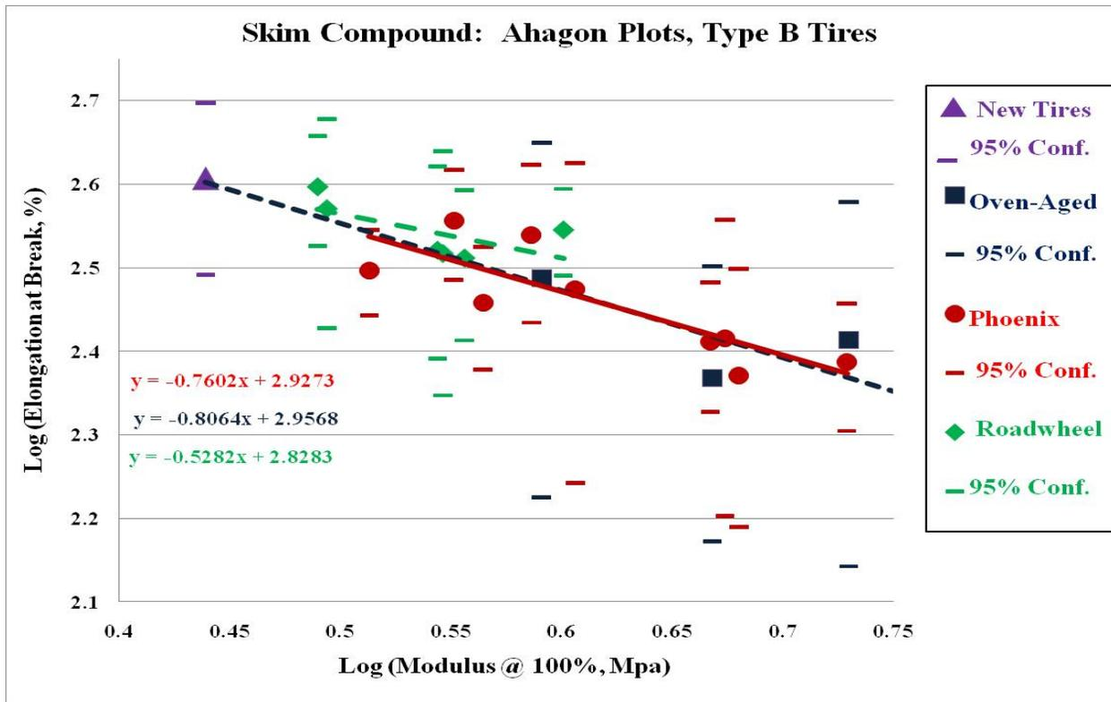
Figure 13. Ahagon Plot of Skim-Coat Compound for Type B Tires
