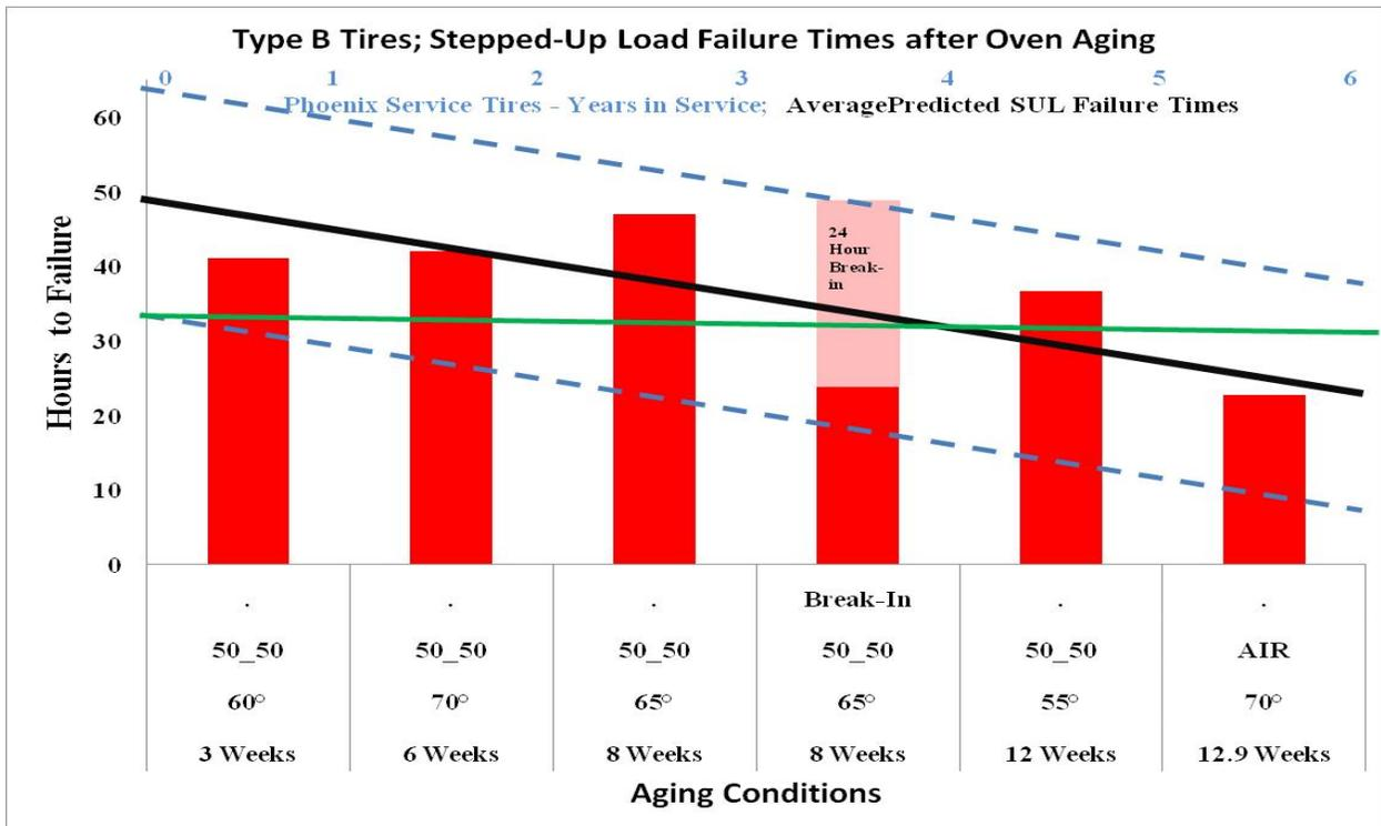
Figure 46. Stepped-up Load Test Failure Times: Oven-Aged Type B Tires Compared to Predicted Values for Tires With 1 to 6 Years of Service in Phoenix
