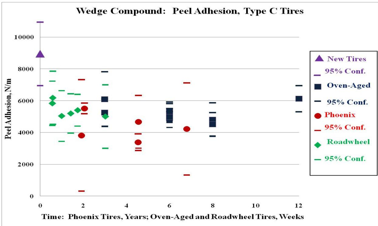
Figure 38. Peel Adhesion Type C Tire Wedge Compound After Oven-Aging, Roadwheel Testing or Service in Phoenix
