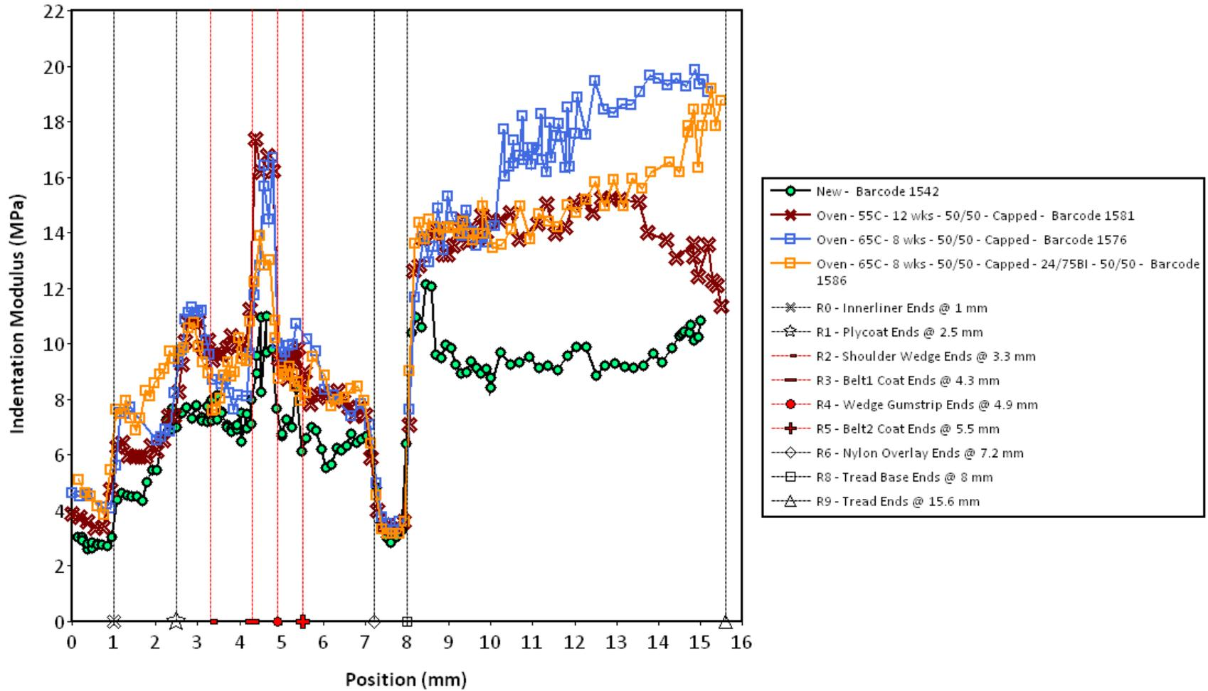
Note: Observe how the 24-hour break-in at 75 mph for tire 1586 produced less belt package hardening than 1576 at the same oven conditions with no break-in.
