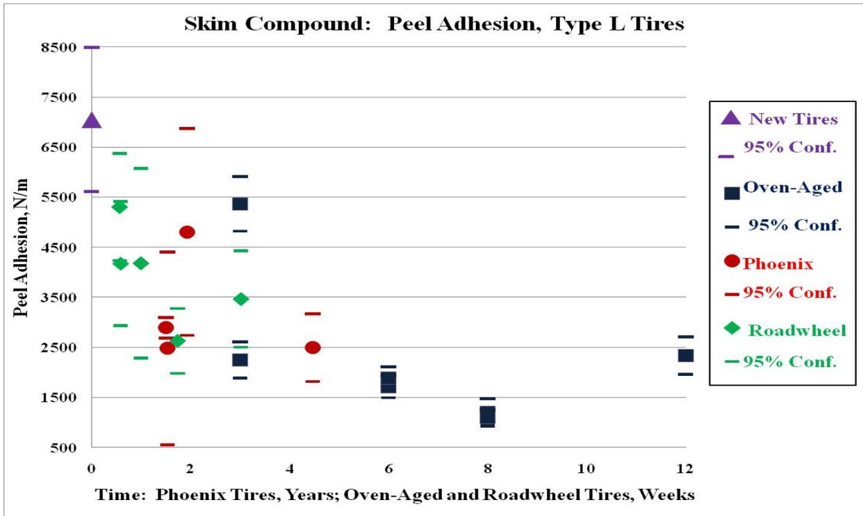
**Figure 36. Peel Adhesion Type L Tire Skim Compound After Oven-Aging, Roadwheel Testing or Service in Phoenix**
