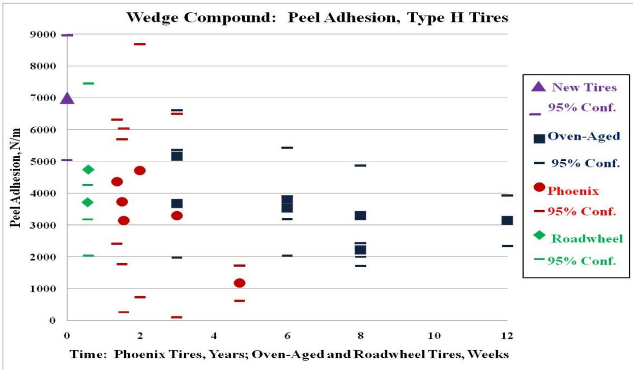
Figure 41. Peel Adhesion Type H Tire Wedge Compound After Oven-Aging, Roadwheel Testing or Service in Phoenix
