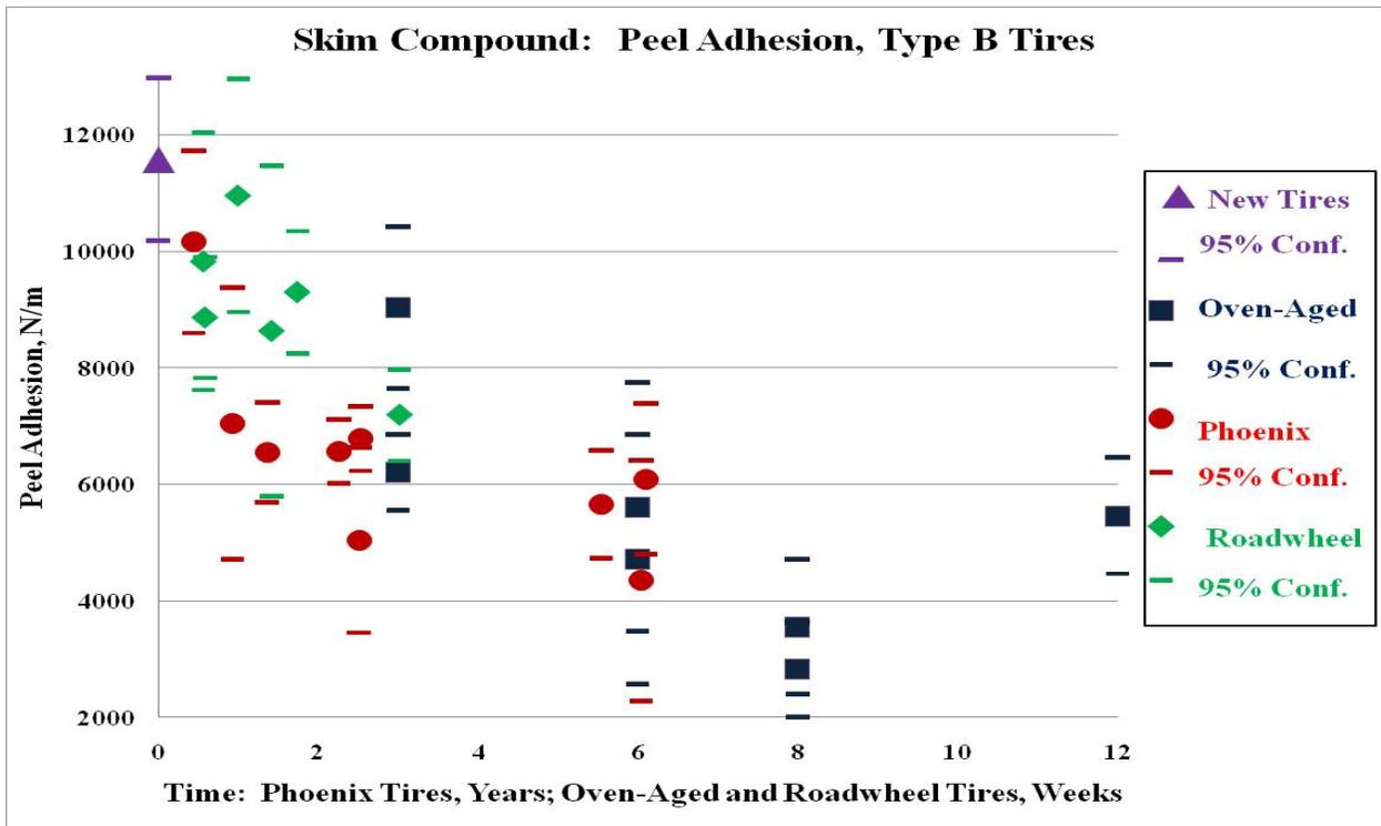
**Figure 31. Peel Adhesion Type B Tire Skim Compound After Oven-Aging, Roadwheel Testing or Service in Phoenix**
