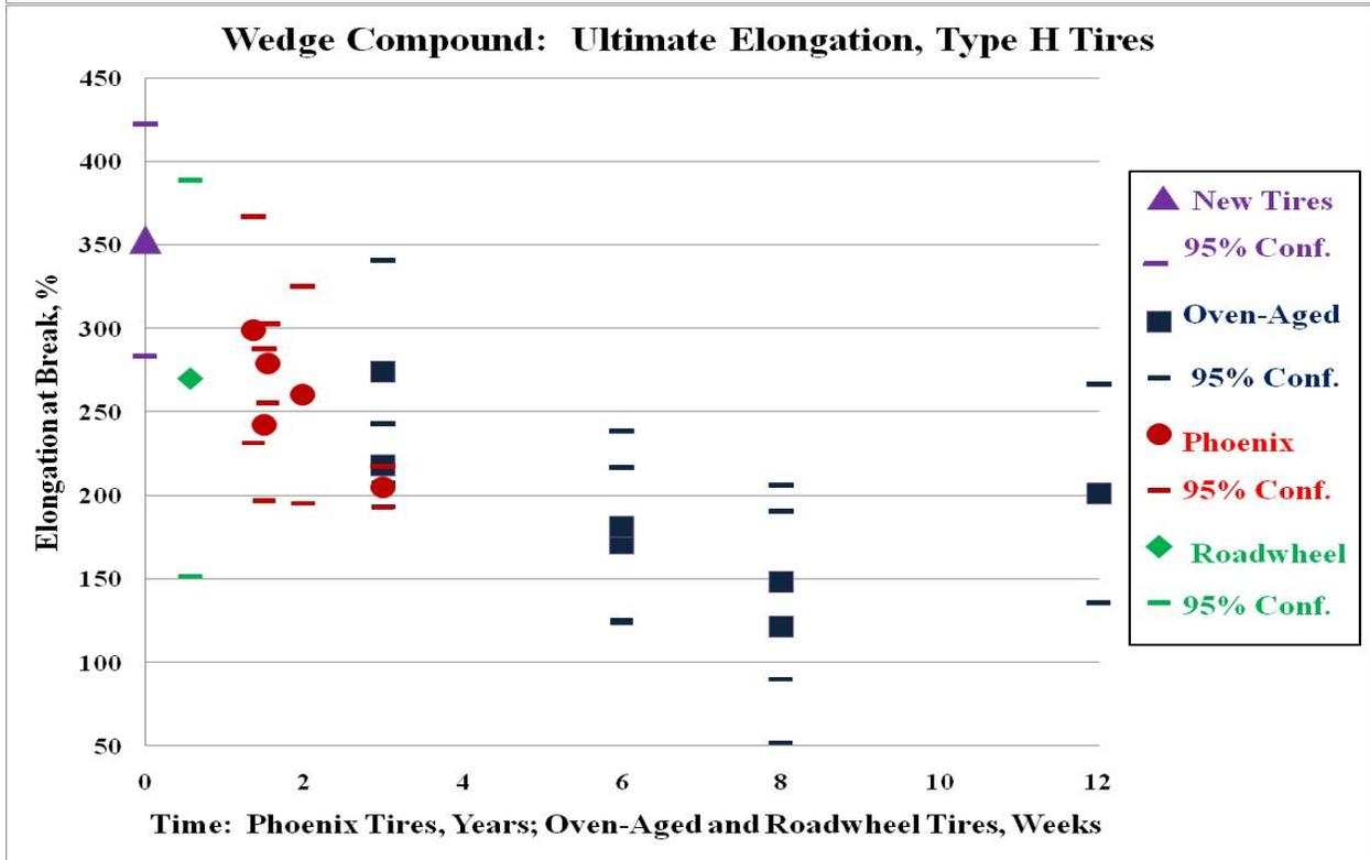
**Figure 23. Modulus @ 100% Strain and Ultimate Elongation for Wedge Compound of Type H Tires**
