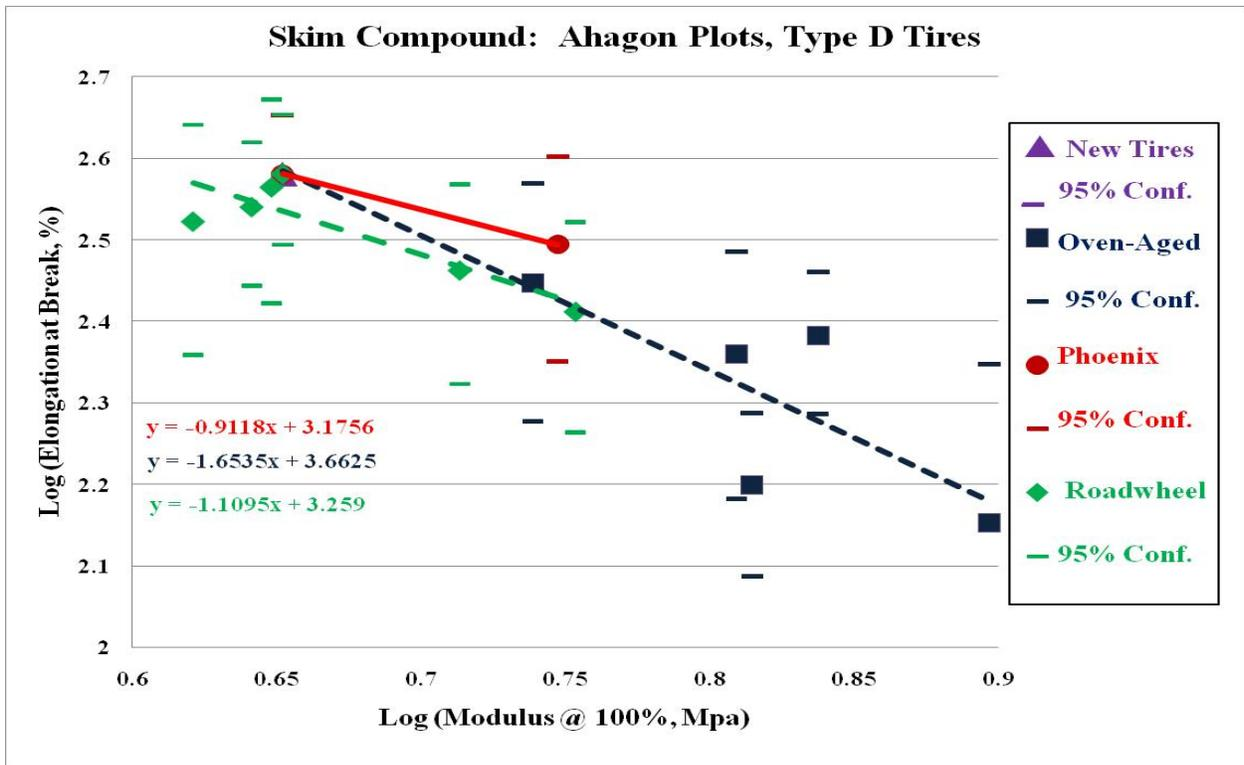
Figure 15. Ahagon Plot of Skim-Coat Compound for Type D Tires
