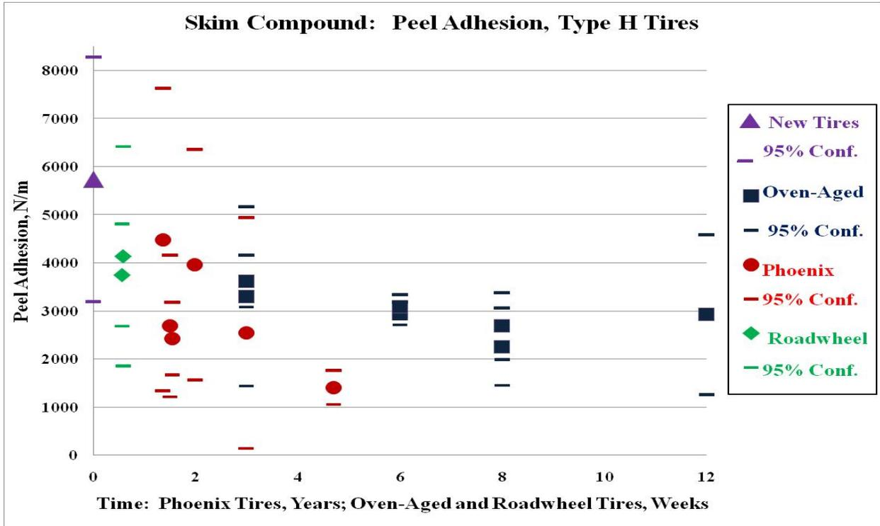
**Figure 35. Peel Adhesion Type H Tire Skim Compound After Oven-Aging, Roadwheel Testing or Service in Phoenix**
