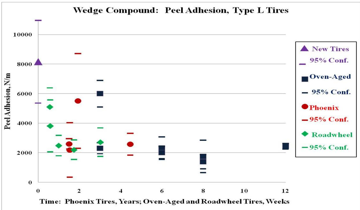
Figure 42. Peel Adhesion Type L Tire Wedge Compound After Oven-Aging, Roadwheel Testing or Service in Phoenix
