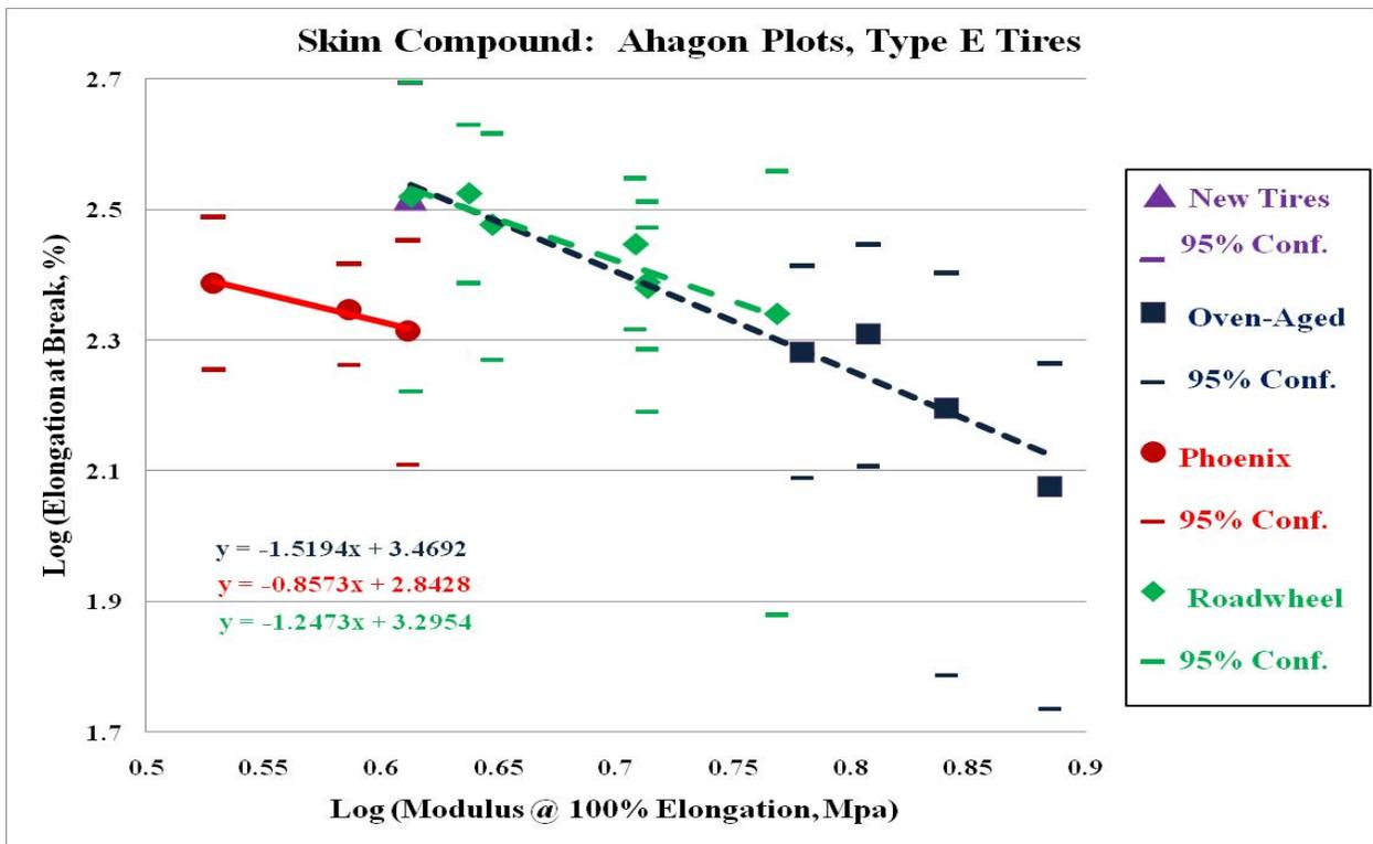
Figure 16. Ahagon Plot of Skim-Coat Compound for Type E Tires
