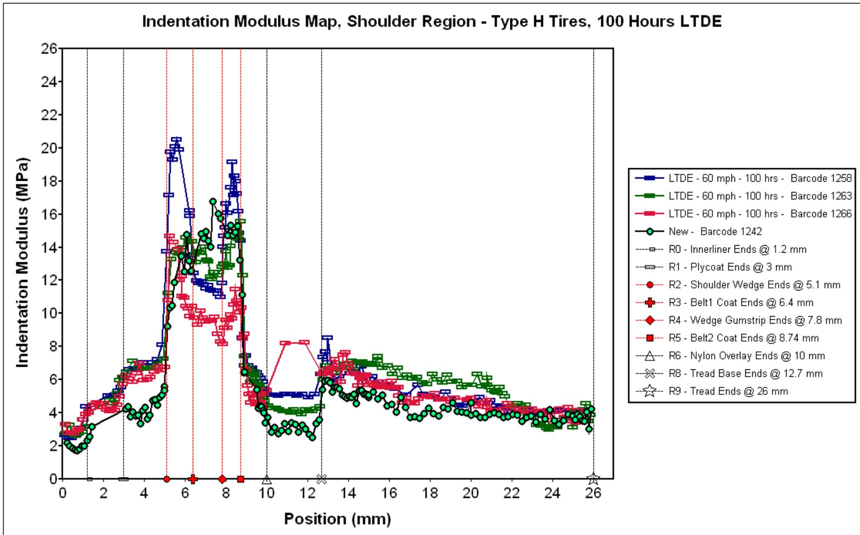
Note: Roadwheel testing of new H tires again produced belt-package softening similar to that observed in Phoenix-retrieved type H tires.
