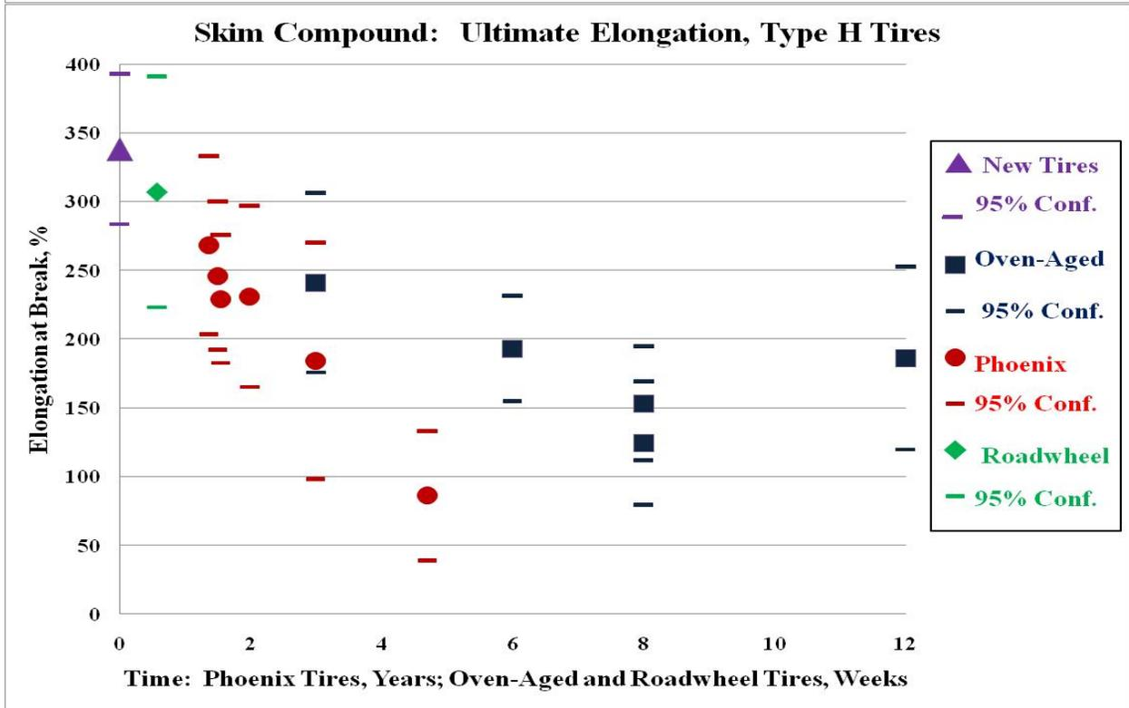
**Figure 11. Modulus @ 100% Strain and Ultimate Elongation for Skim-Coat Compound of Type H Tires**
