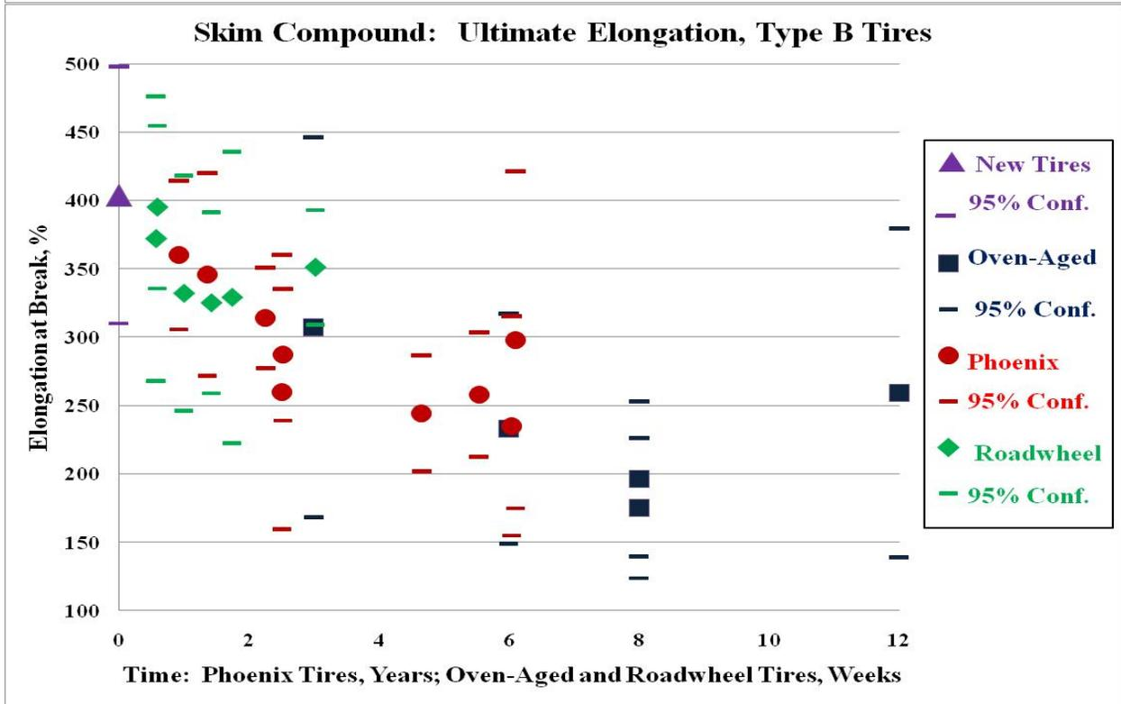
**Figure 7. Modulus @ 100% Strain and Ultimate Elongation for Skim-Coat Compound of Type B Tires**
