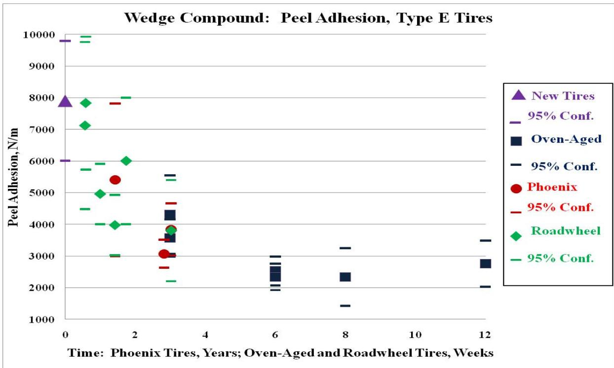
Figure 40. Peel Adhesion Type E Tire Wedge Compound After Oven-Aging, Roadwheel Testing or Service in Phoenix
