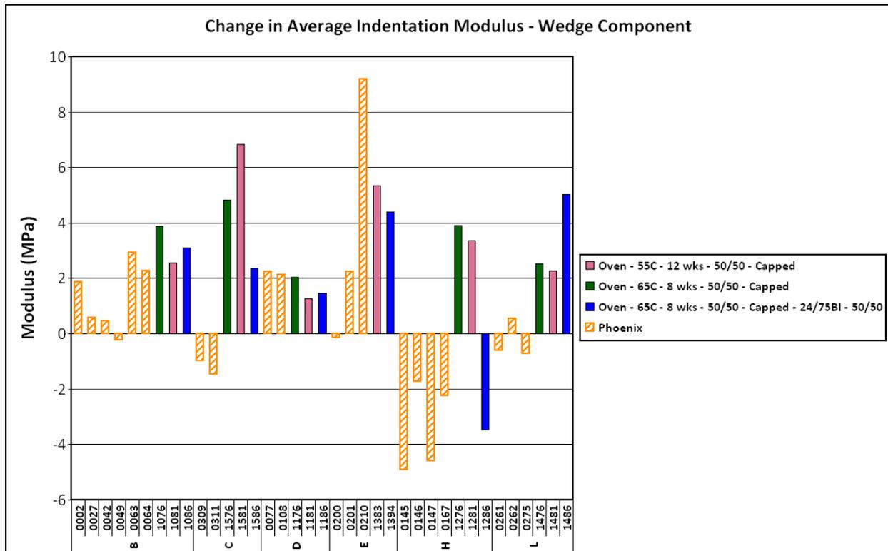
**Figure 5. Changes in Indentation Modulus for Oven-Aged and Phoenix Service Tires**
