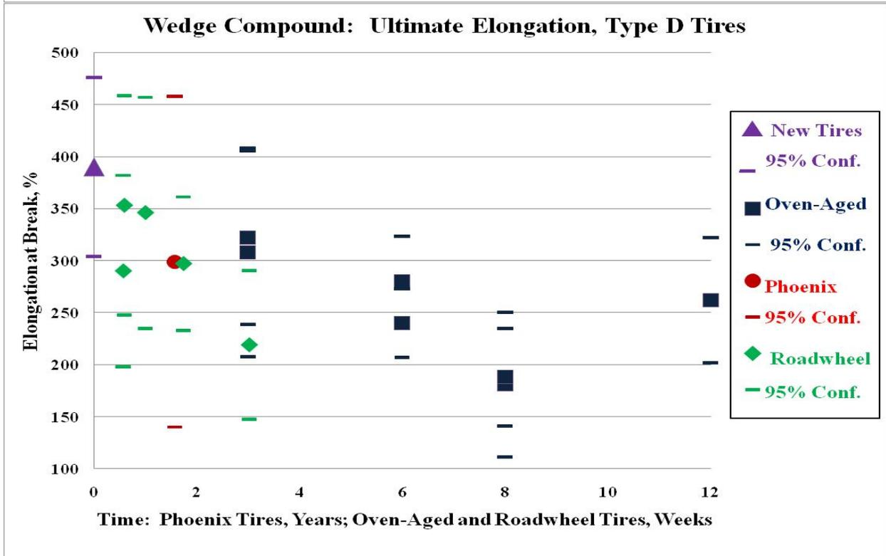
**Figure 21. Modulus @ 100% Strain and Ultimate Elongation for Wedge Compound of Type D Tires**
