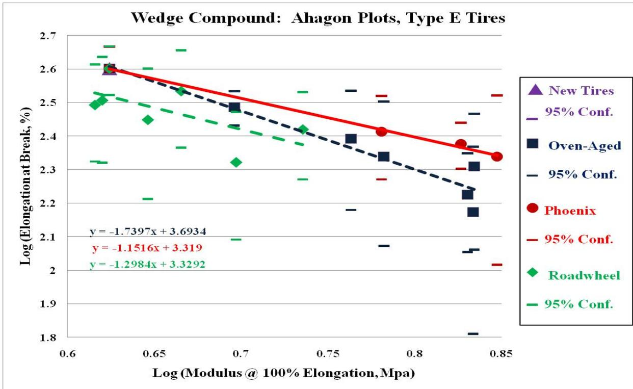
Figure 28. Ahagon Plot of Skim-Coat Compound for Type E Tires
