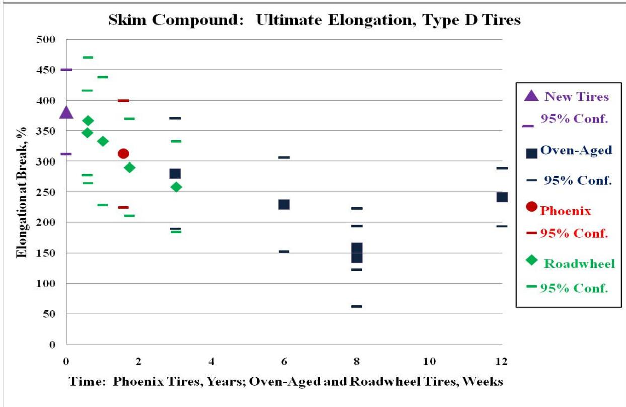
**Figure 9. Modulus @ 100% Strain and Ultimate Elongation for Skim-Coat Compound of Type D Tires**
