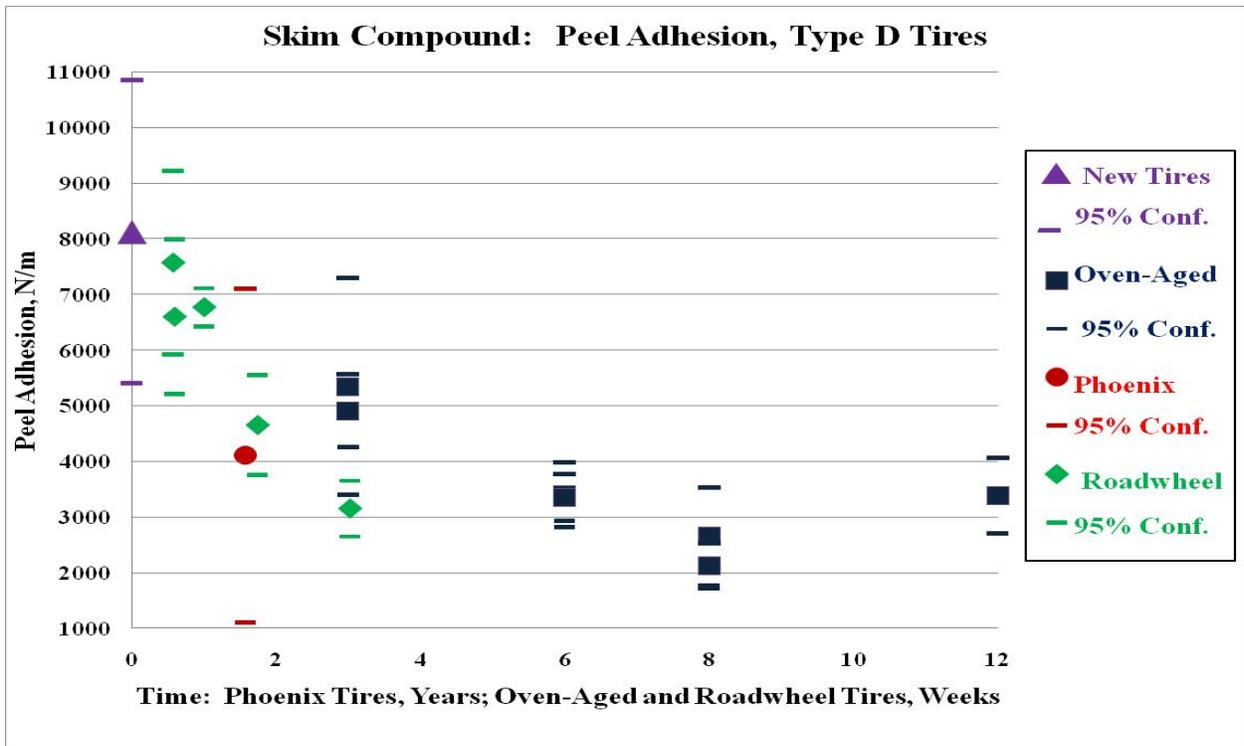
Figure 33. Peel Adhesion Type D Tire Skim Compound After Oven-Aging, Roadwheel Testing or Service in Phoenix
