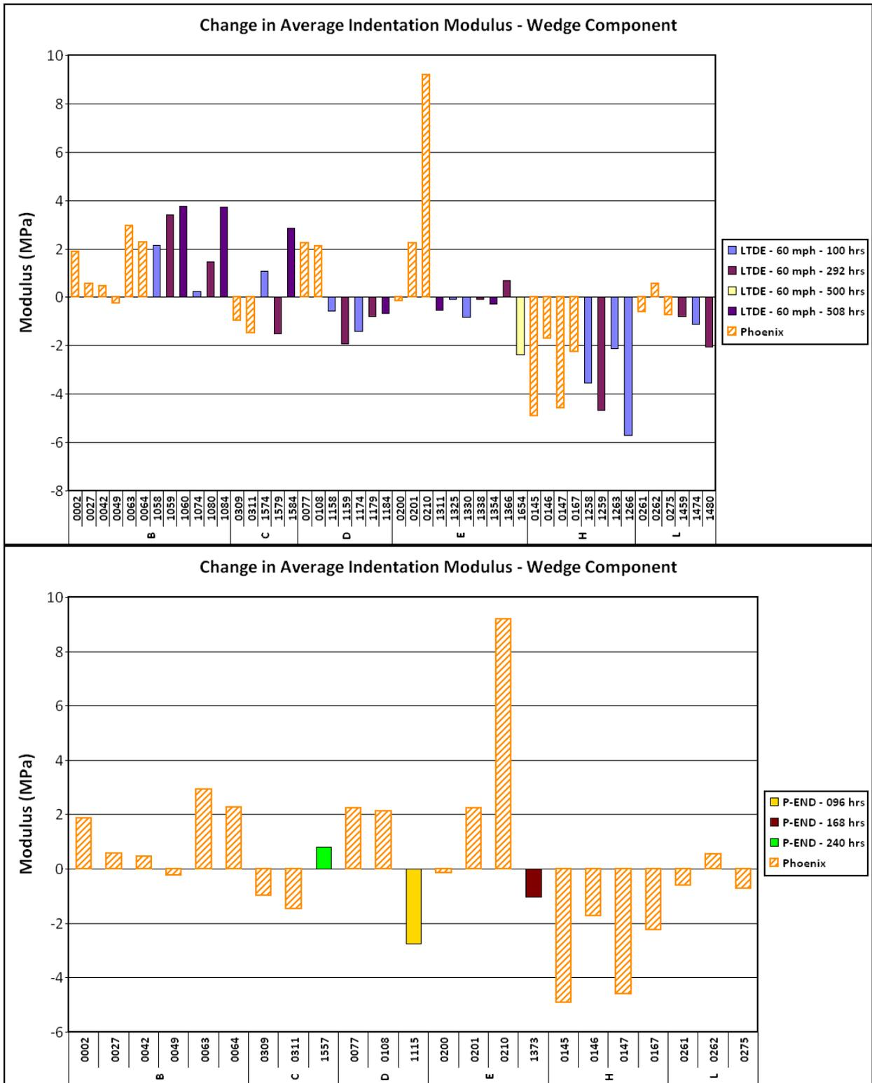
Figure 4. Changes in Indentation Modulus for Roadwheel Tests and Phoenix Service Tires
