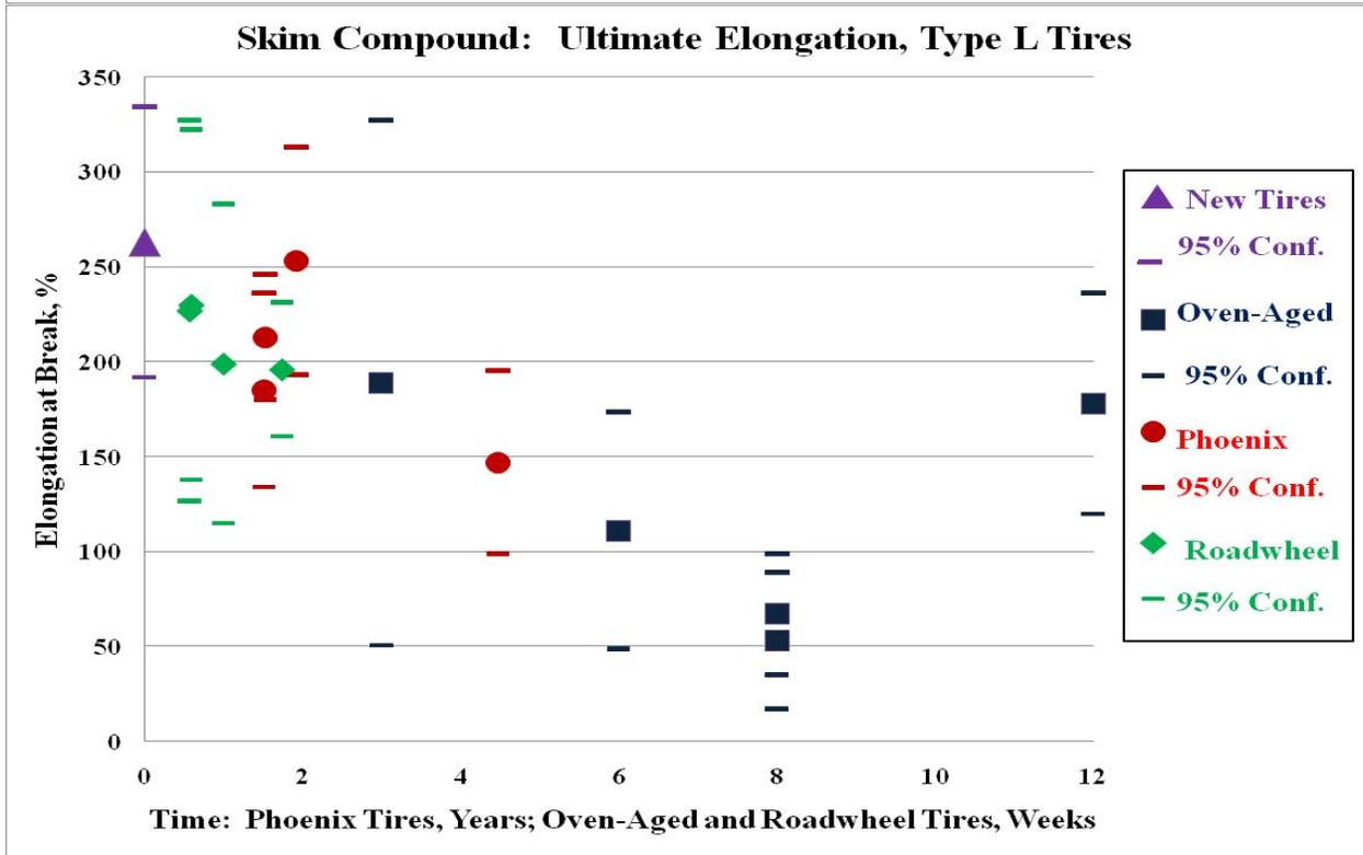
**Figure 12. Modulus @ 100% Strain and Ultimate Elongation for Skim-Coat Compound of Type L Tires**
