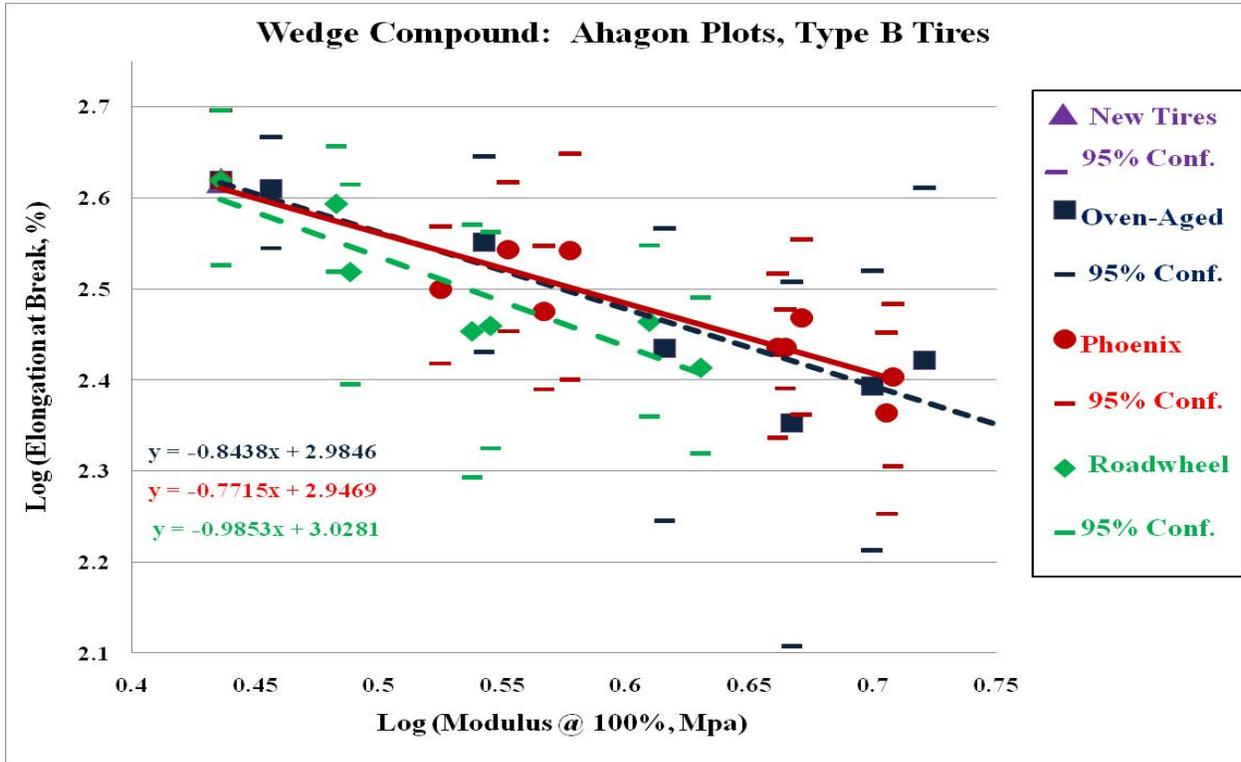
Figure 25. Ahagon Plot of Skim-Coat Compound for Type B Tires
