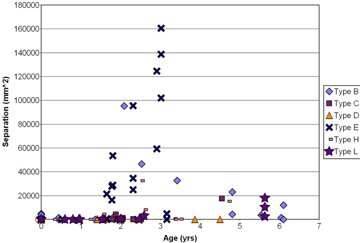
**Figure 43. Bead-to-Bead Shearography Separation @ 50 mbar Vacuum Versus Age, New, and Phoenix On-Road Tires (45 New Tires, 106 Phoenix Tires)**
