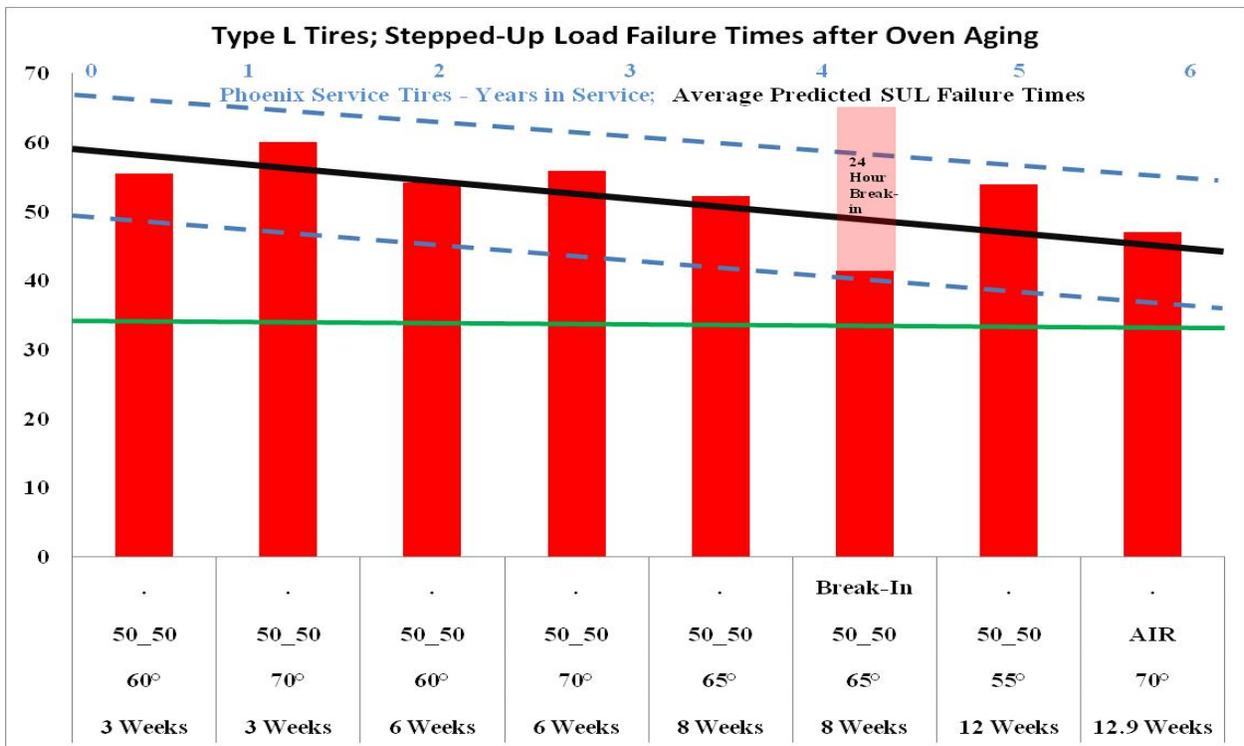
Figure 51. Stepped-up Load Test Failure Times: Oven-Aged Type L Tires Compared to Predicted Values for Tires With 1 to 6 Years of Service in Phoenix
