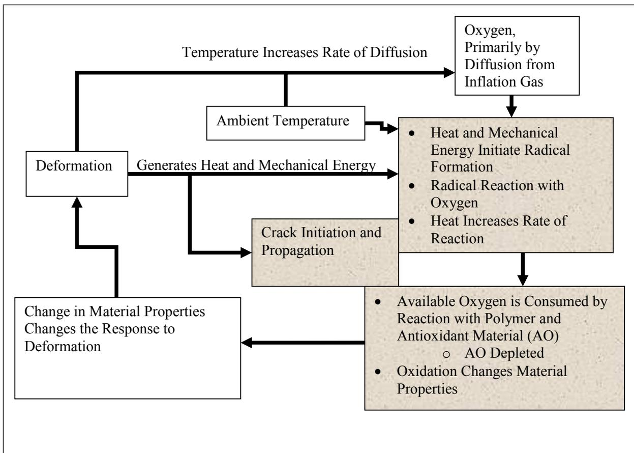
**Figure 1. Simplified Illustration of Rubber Degradation by Mechanical Energy, Heat Energy, and Reaction With Oxygen**
