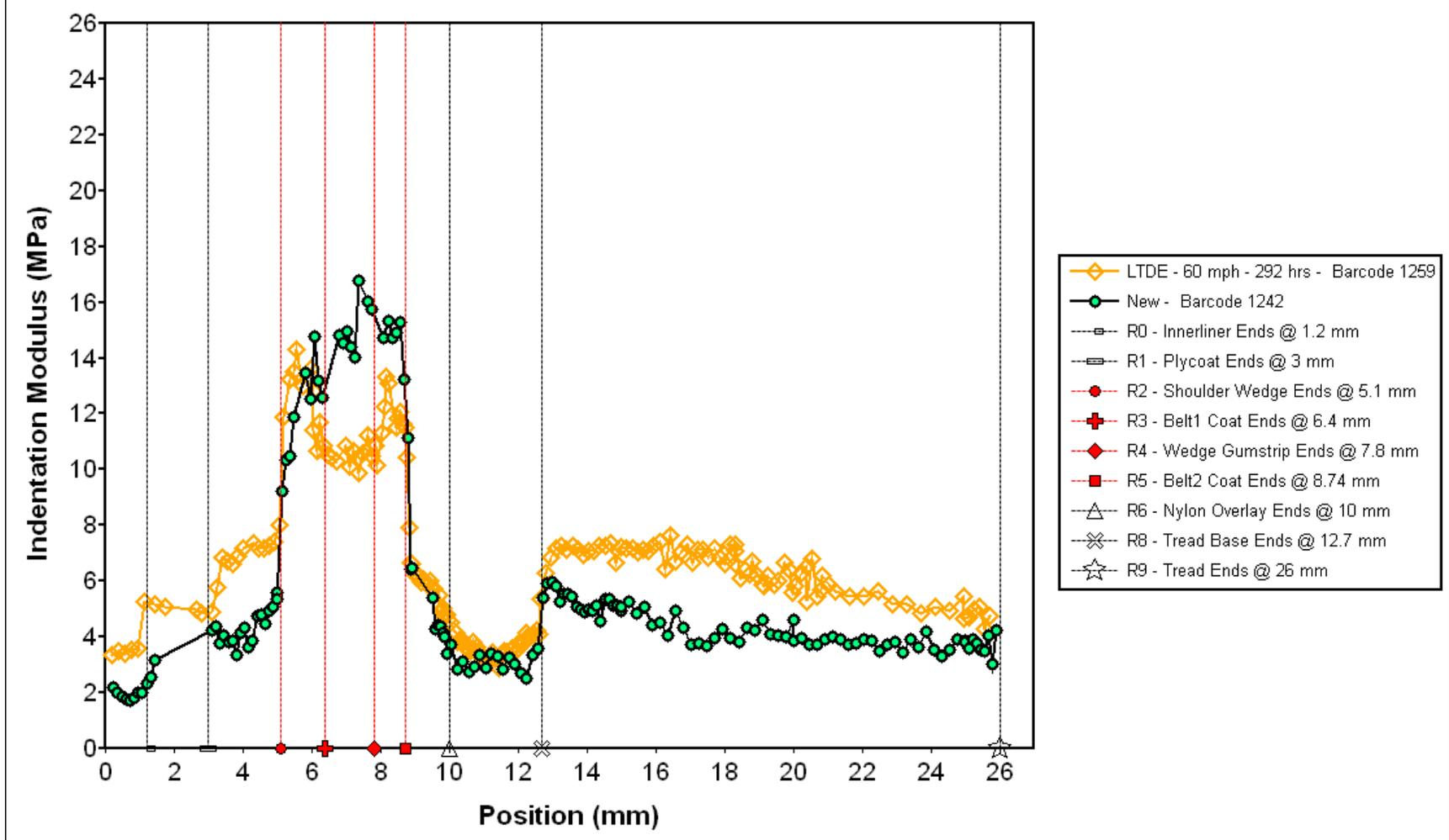
Note: Roadwheel testing of new H tires again produced belt-package softening similar to that observed in Phoenix-retrieved type H tires.
