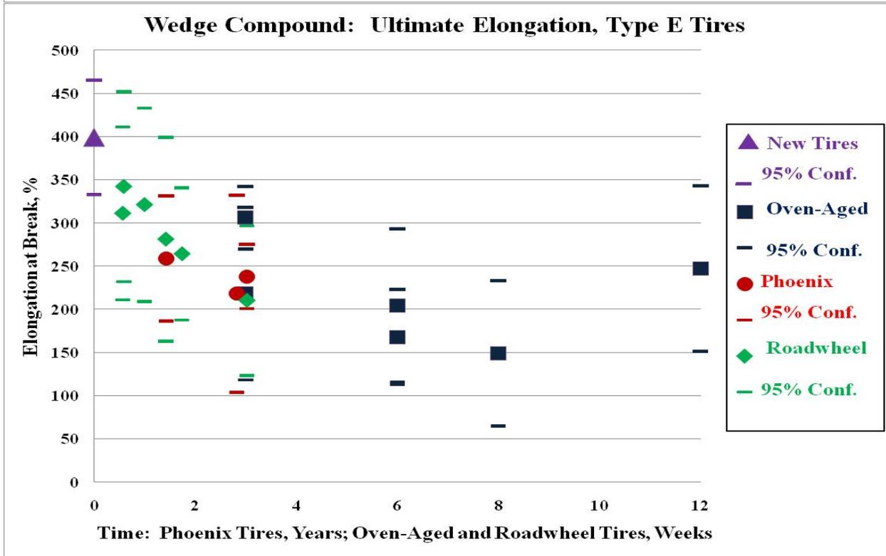
**Figure 22. Modulus @ 100% Strain and Ultimate Elongation for Wedge Compound of Type E Tires**
