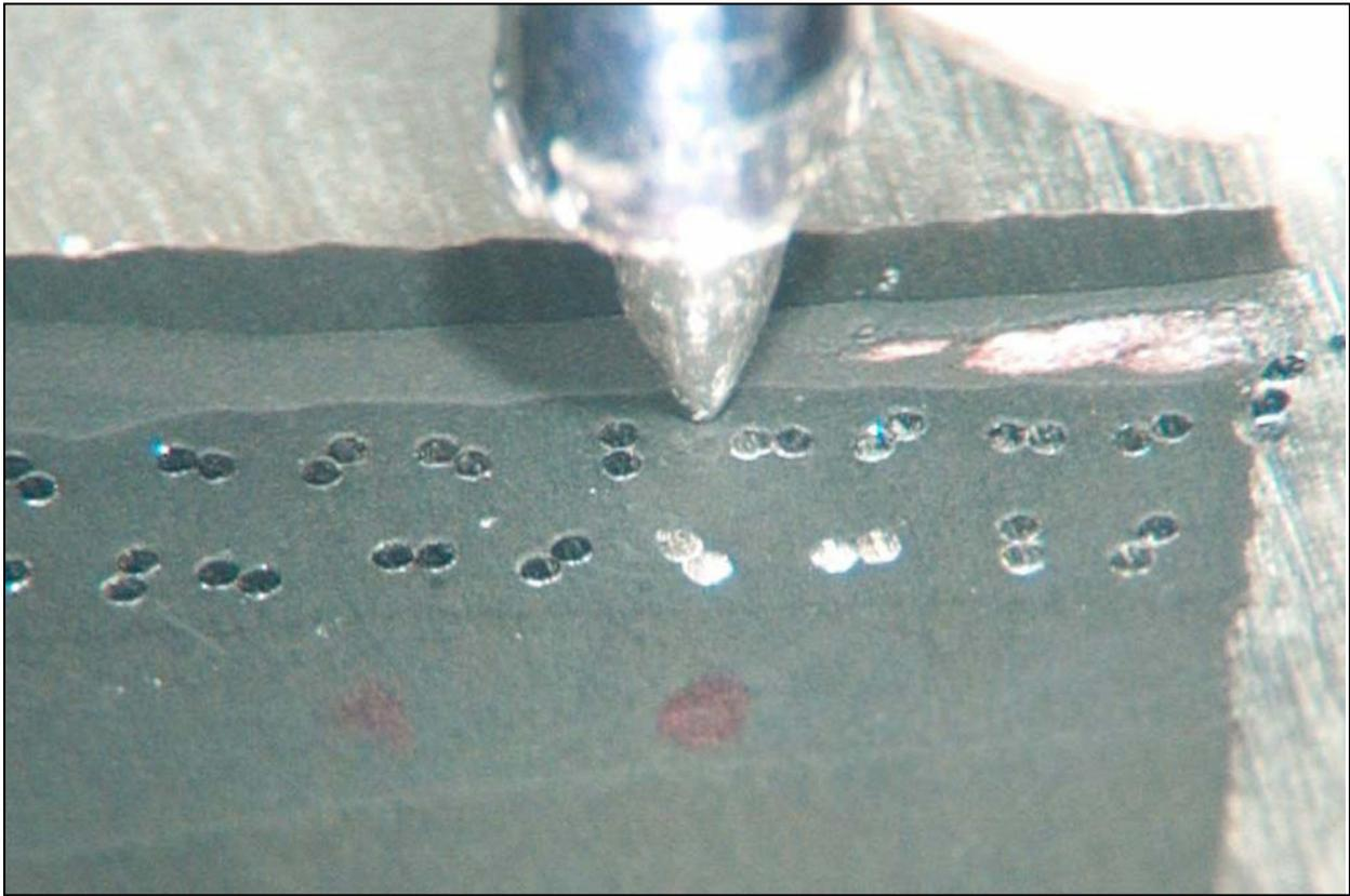
**Figure 3. Example Micro-Indentation Modulus**
