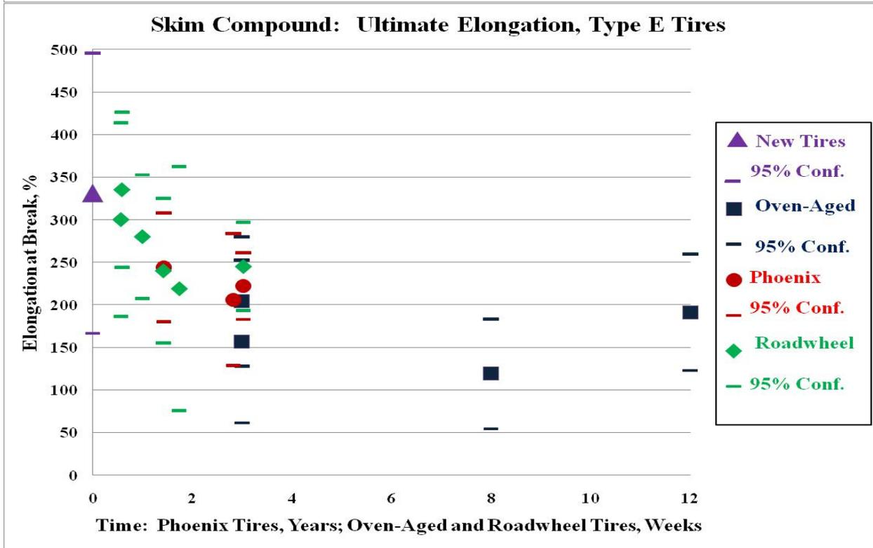
**Figure 10. Modulus @ 100% Strain and Ultimate Elongation for Skim-Coat Compound of Type E Tires**
