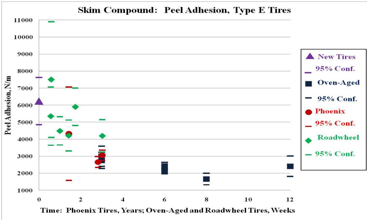
Figure 34. Peel Adhesion Type E Tire Skim Compound After Oven-Aging, Roadwheel Testing or Service in Phoenix
