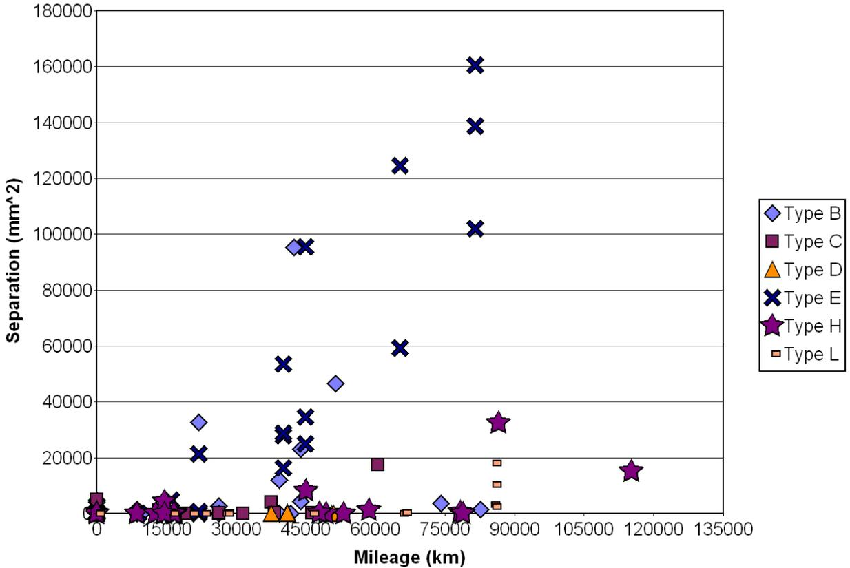
**Figure 44. Bead-to-Bead Shearography Separation @ 50 mbar Vacuum Versus Mileage, New, and Phoenix On-Road Tires (45 New Tires, 106 Phoenix Tires)**
