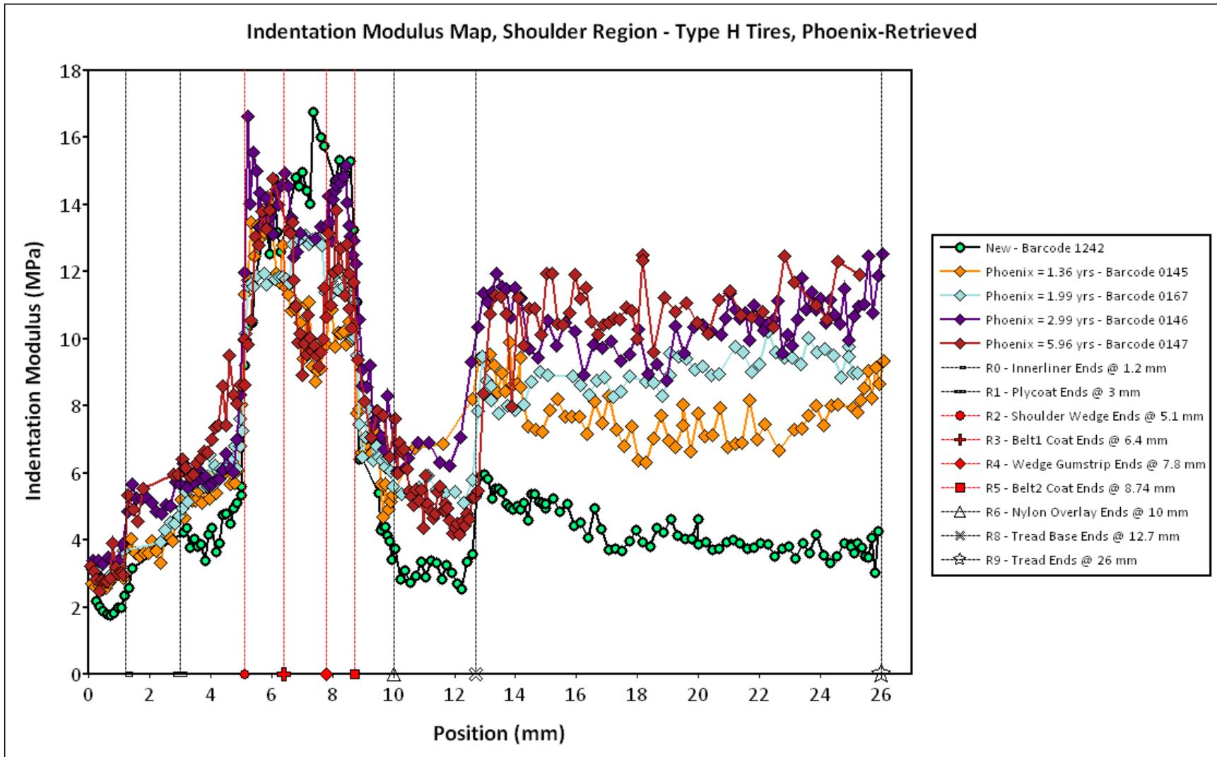
Note: Observe how the belt packages (5.1 mm to 8.74 mm) of the four type H tires retrieved from service in Phoenix soften relative to the new tire (1242).
