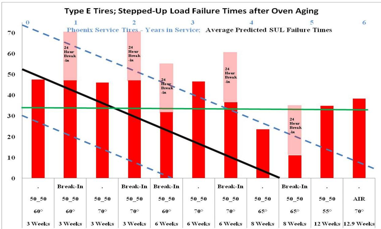
Figure 49. Stepped-up Load Test Failure Times: Oven-Aged Type E Tires Compared to Predicted Values for Tires With 1 to 6 Years of Service in Phoenix
