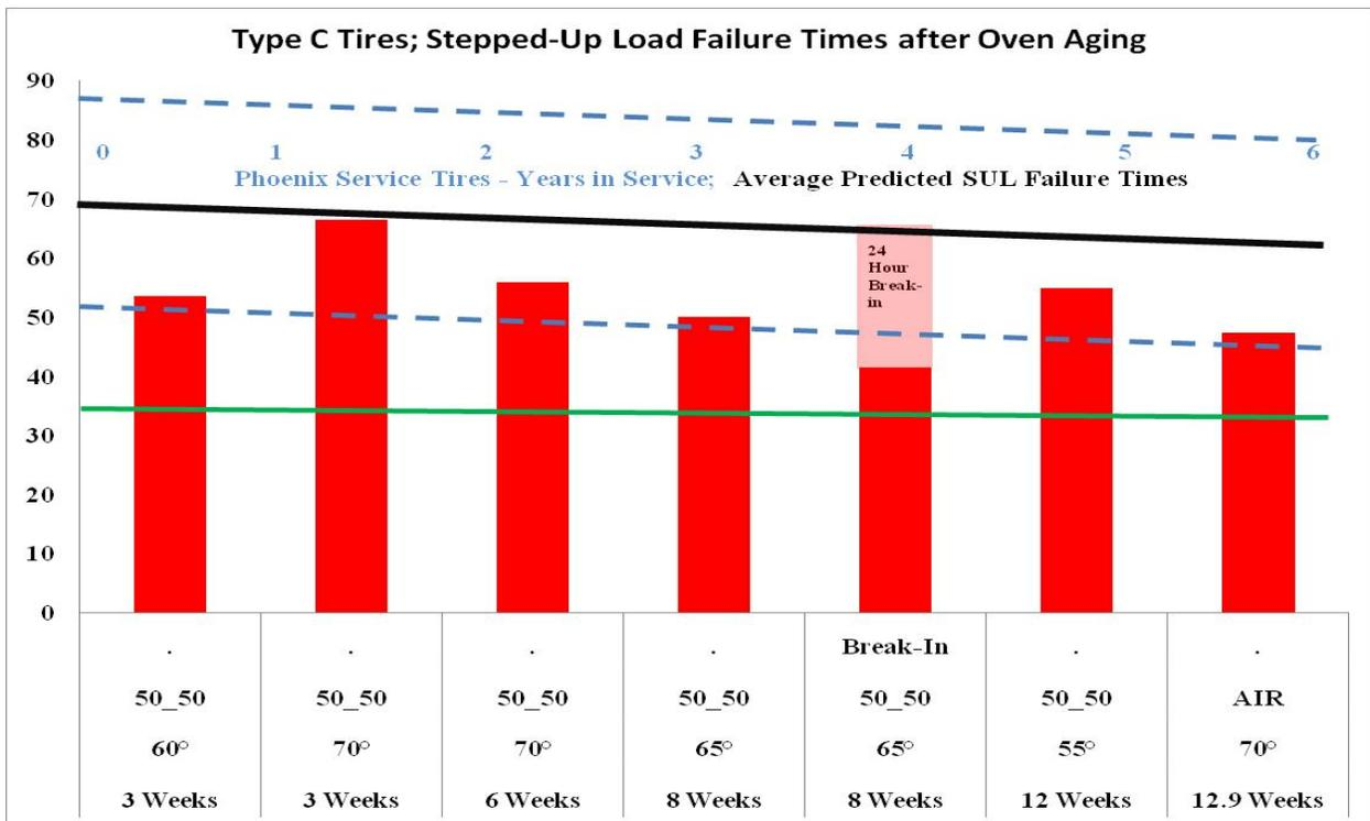
Figure 47. Stepped-up Load Test Failure Times: Oven-Aged Type C Tires Compared to Predicted Values for Tires With 1 to 6 Years of Service in Phoenix
