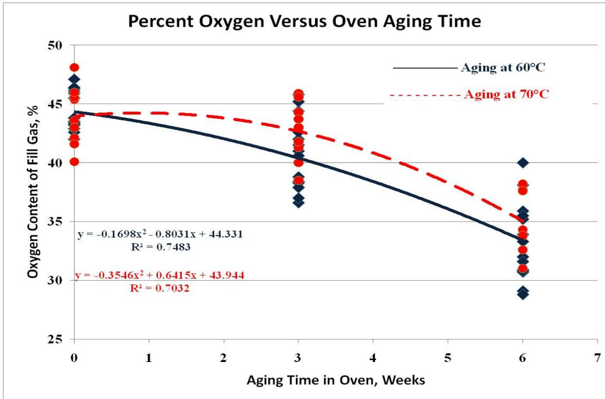
**Figure 45. Percent Oxygen Content of the Fill Gas Versus Oven-Aging Time**
