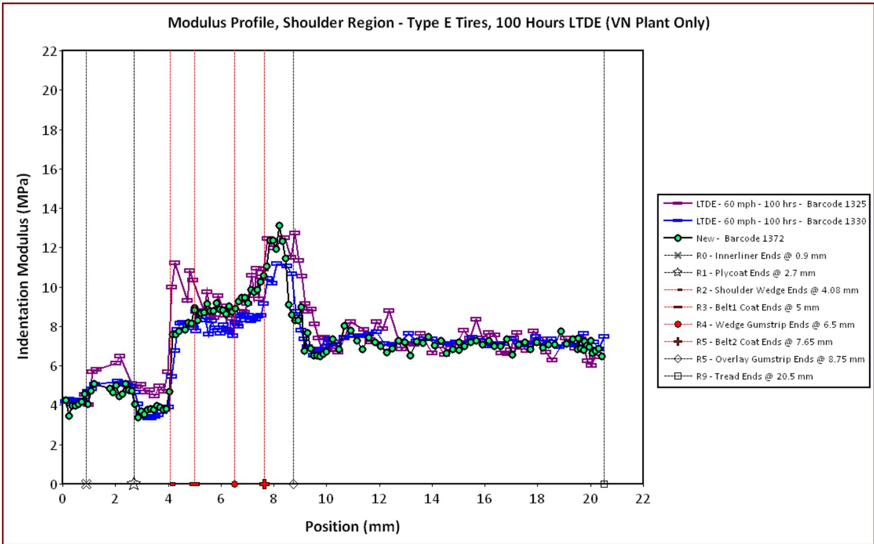
Note how LTDE targets the belt1 coat and wedge in this and subsequent figures.
