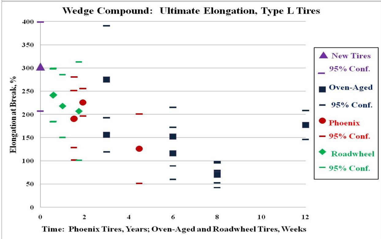
**Figure 24. Modulus @ 100% Strain and Ultimate Elongation for Wedge Compound of Type L Tires**
