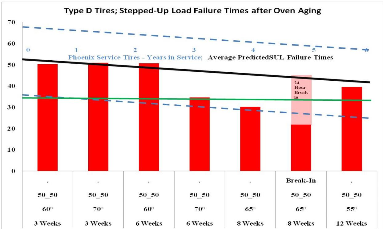
Figure 48. Stepped-up Load Test Failure Times: Oven-Aged Type D Tires Compared to Predicted Values for Tires With 1 to 6 Years of Service in Phoenix
