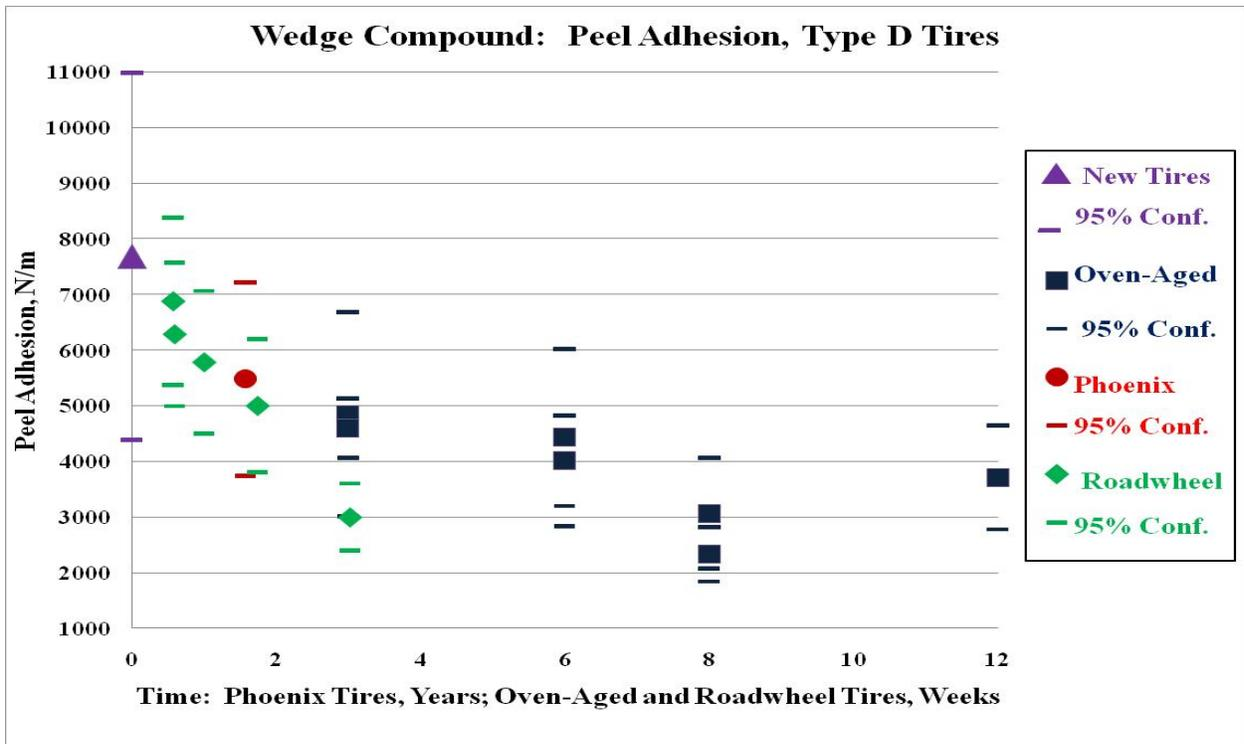
Figure 39. Peel Adhesion Type D Tire Wedge Compound After Oven-Aging, Roadwheel Testing or Service in Phoenix
