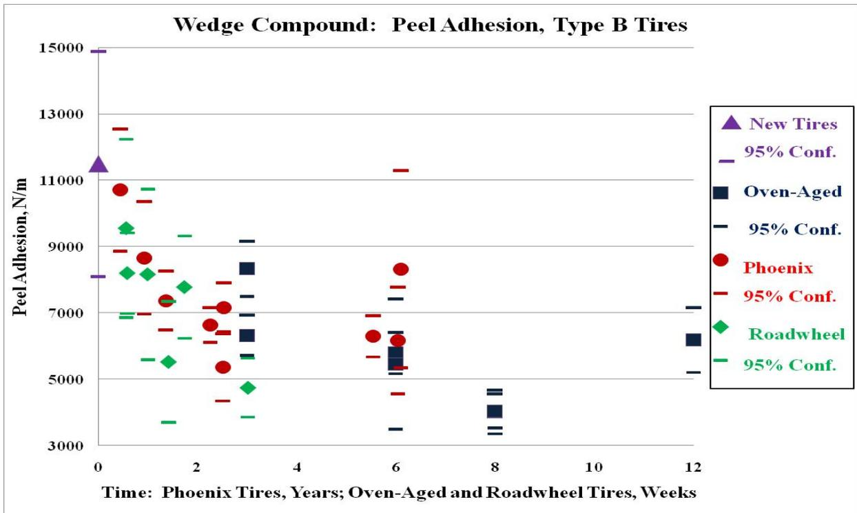
Figure 37. Peel Adhesion Type B Tire Wedge Compound After Oven-Aging, Roadwheel Testing or Service in Phoenix
