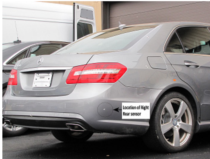
Figure 3-8 Mercedes BSM Sensor Proximity
