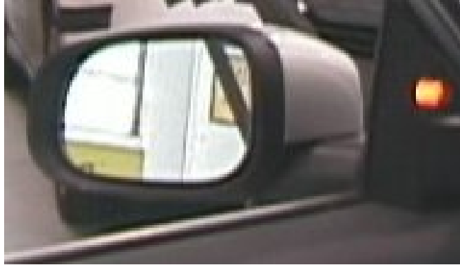
Figure 3-3 Photograph of Volvo Left Side “Lighted” Alert Indicator on Inside of Front Door Frame
