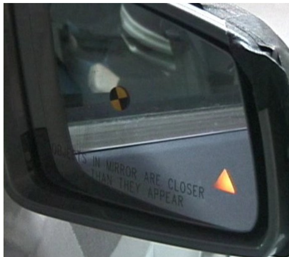
Figure 3-10 Photograph of the Warning Indicator Integrated Into the Right Mirror of the Mercedes
