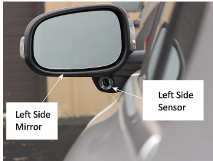
Figure 3-1 Volvo Left BSM Sensor (Camera) Mounted Beneath Mirror (Viewed From Behind the Vehicle)
