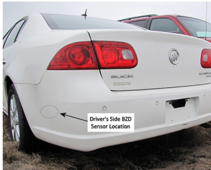
Figure 3-4 Buick BSM Sensor Proximity
