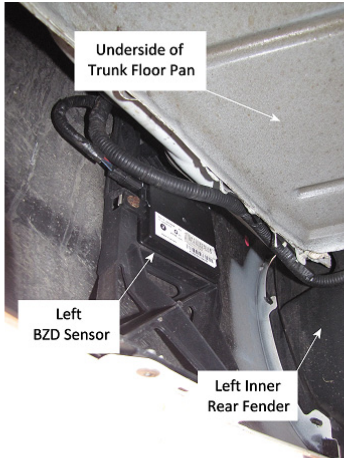
Figure 3-5 Buick Left BSM Sensor Behind Rear Bumper Wrap-Around
