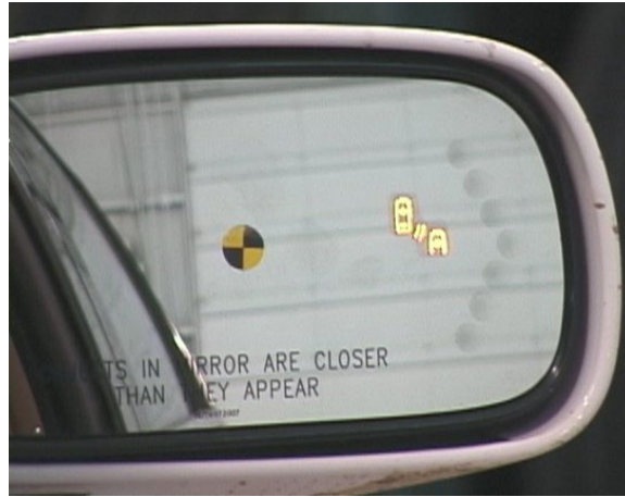
Figure 3-7 Photographic Image of the Buick Lucerne Warning Icon on the Right Side Mirror
