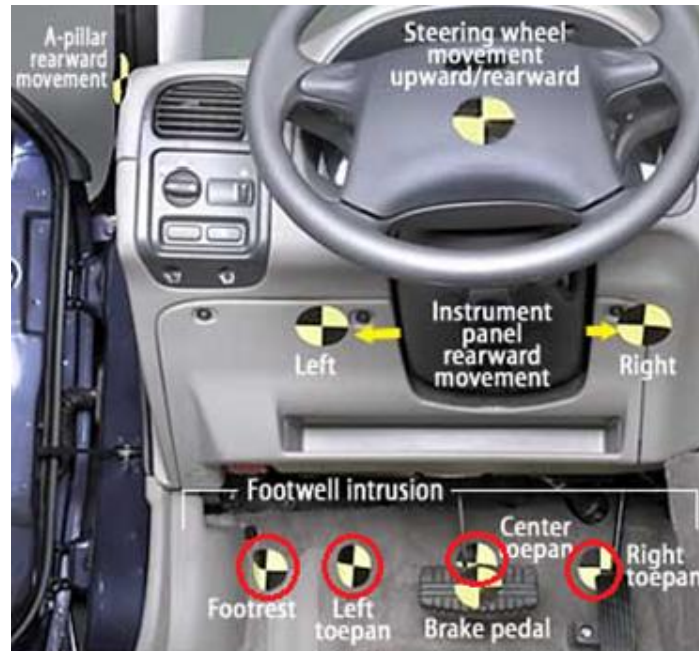
Figure 4-3. Locations for Intrusion Measurements in the IIHS Offset Configuration
