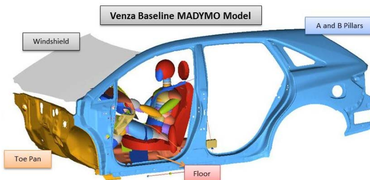
Figure 3-15. Venza MADYMO Model With Imported FE Parts
