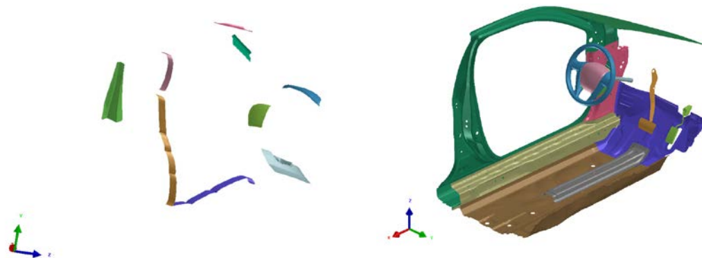
Figure 3-13. Digitized Parts (left) and FE Model Parts (right) That Were Used to Position the MADYMO Model
