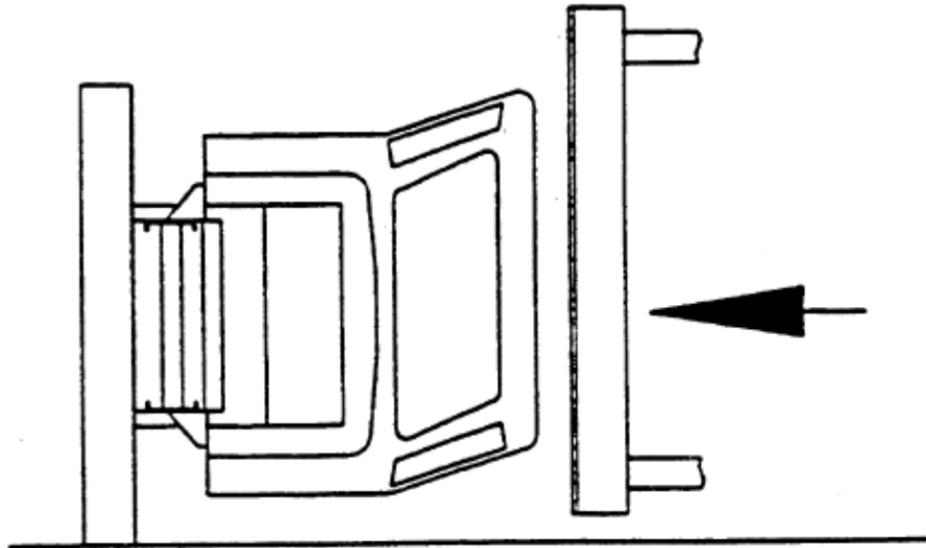
**Figure 6 Quasi-Static Roof Load Configuration**
