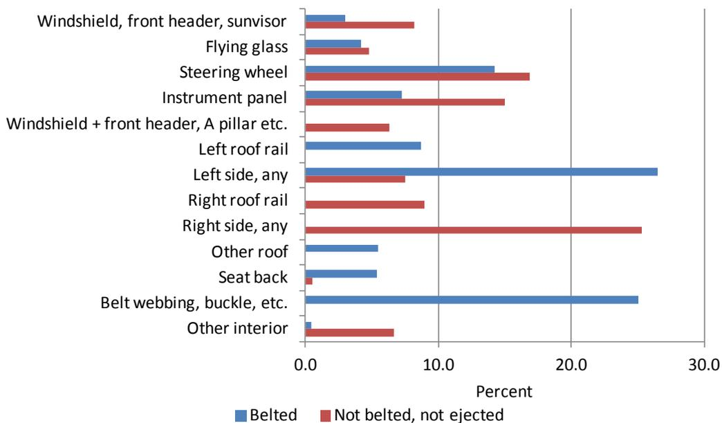
**Figure 37 Tractor-semitrailer and Straight Trucks, Cab Interior Contact for Driver Injuries, Rollover**
