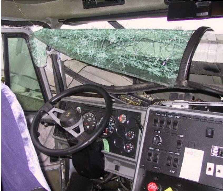
**Figure 29 Hood Intrusion in Frontal Collision**
