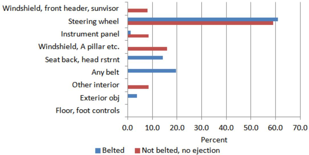
**Figure 40 Source of Injury in Frontal Impacts, AIS2+ Injuries Only, by Seat Belt Use, LTCCS**
