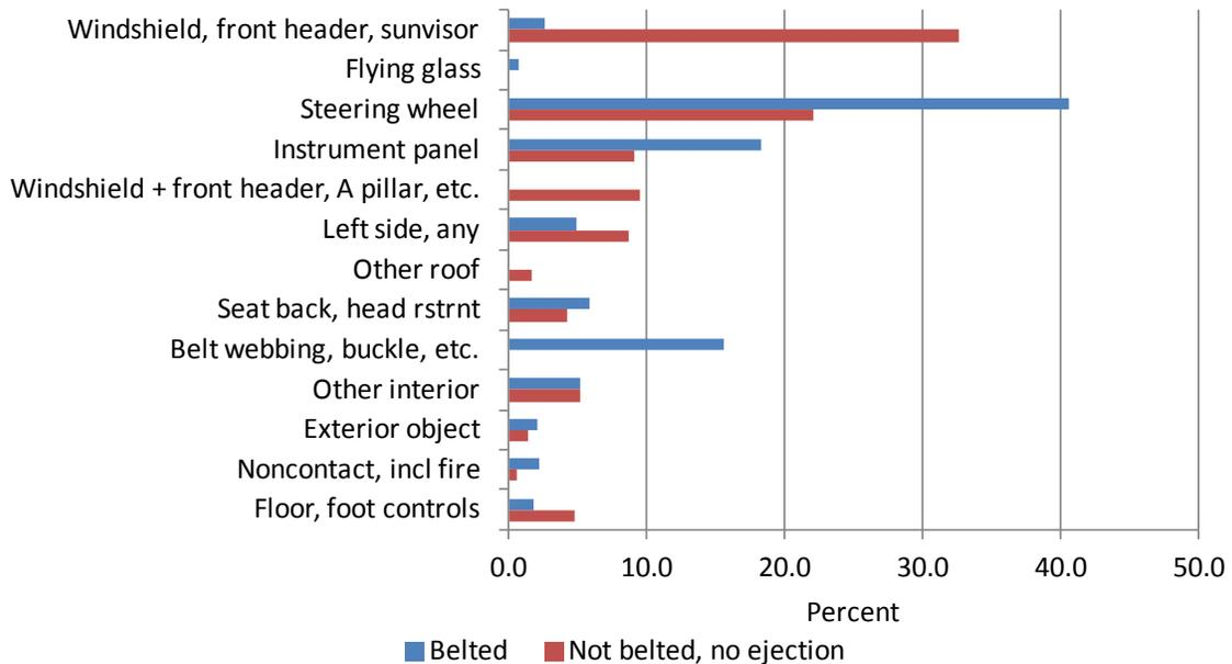
**Figure 39 Source of Injury in Frontal Impacts, by Seat Belt Use, LTCCS Data**
