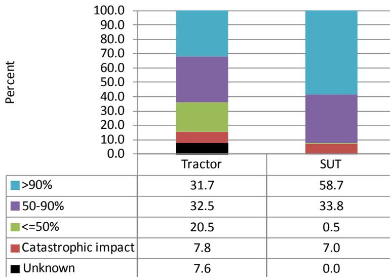
**Figure 18 Cab space remaining by truck type, rollover crashes**
