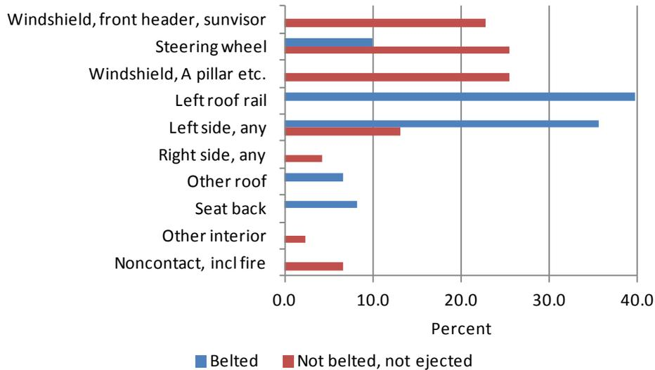
**Figure 38 Tractor-semitrailer and SUTs, Cab Interior Contact for AIS 2+ Injuries, Rollover, LTCCS Data**
