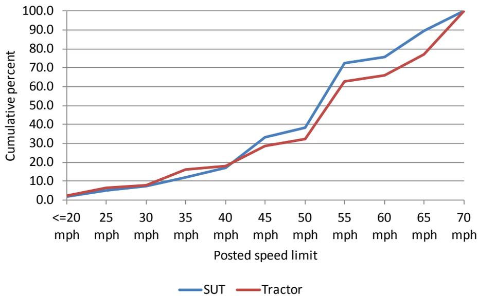
**Figure 13 Cumulative Percentage of Truck Driver Fatal and A Injuries, by Power Unit Type
