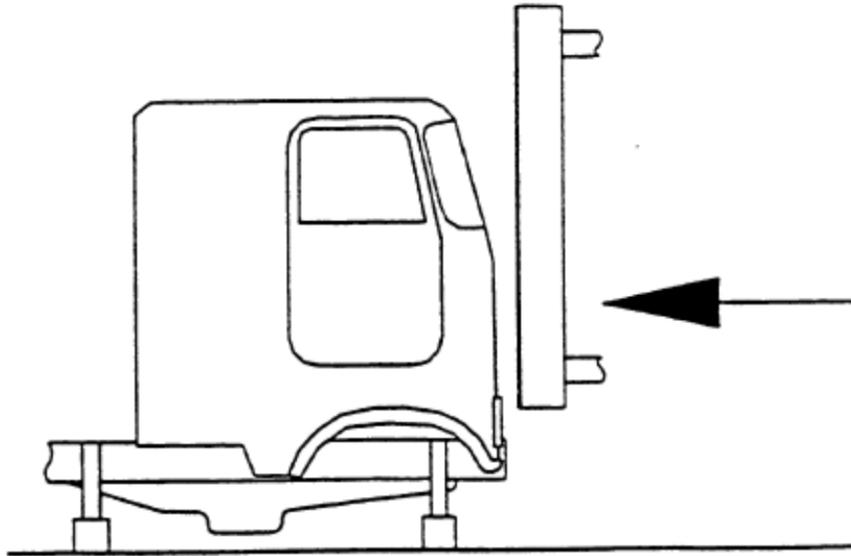
**Figure 3 COE Frontal Strength Test Configuration**
