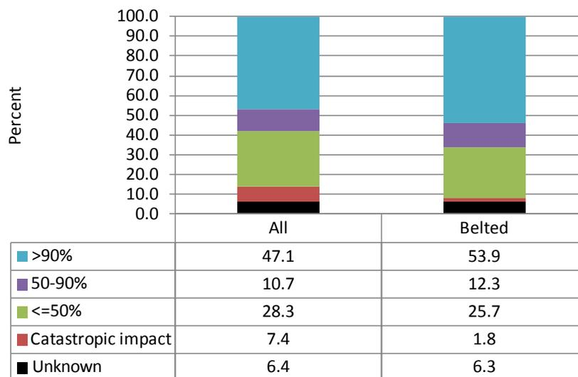
**Figure 27 Cab Space Remaining in Frontal Crashes, All and Belted Drivers Only**
