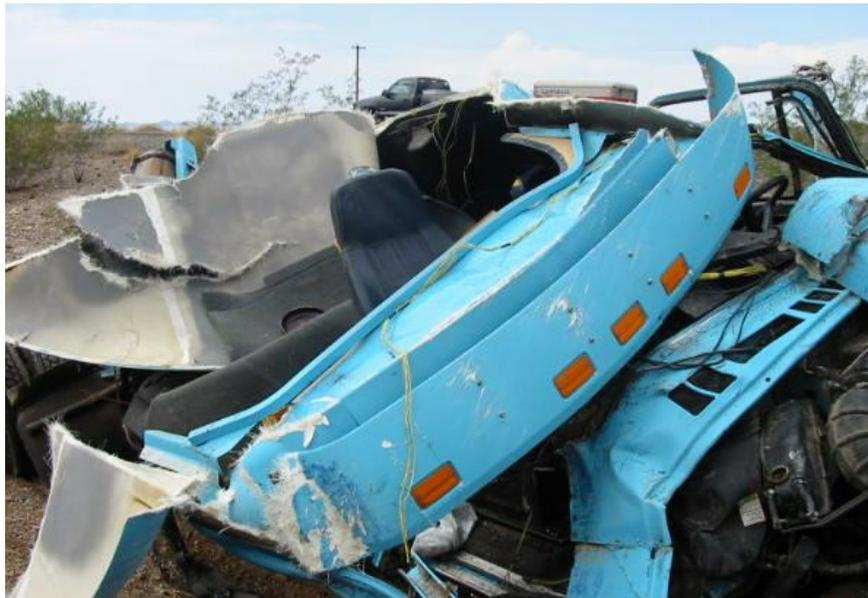
**Figure 16 Truck-tractor rolled 4 quarter turns, destroying the cab**
