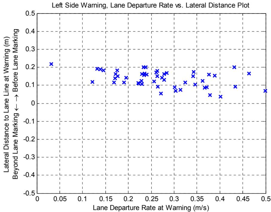
**Figure 3.5 Left-Side Test – Lateral Distance to Lane Line at Warning Versus Lane Departure Rate Plot**
