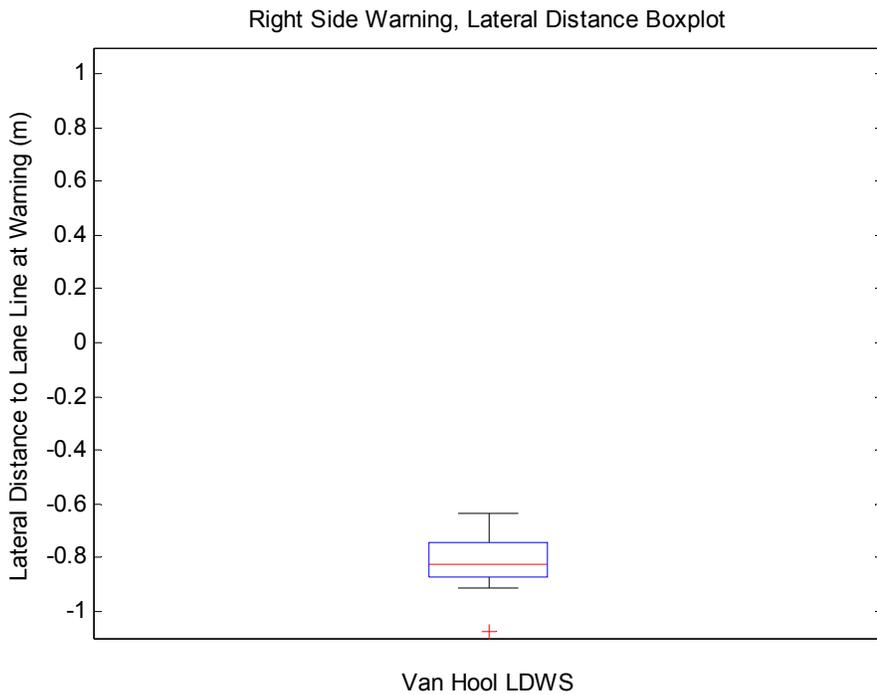
**Figure 3.10 Curved Lane, Right-Side Test – Lateral Distance to the Lane Line at Warning Boxplot**
