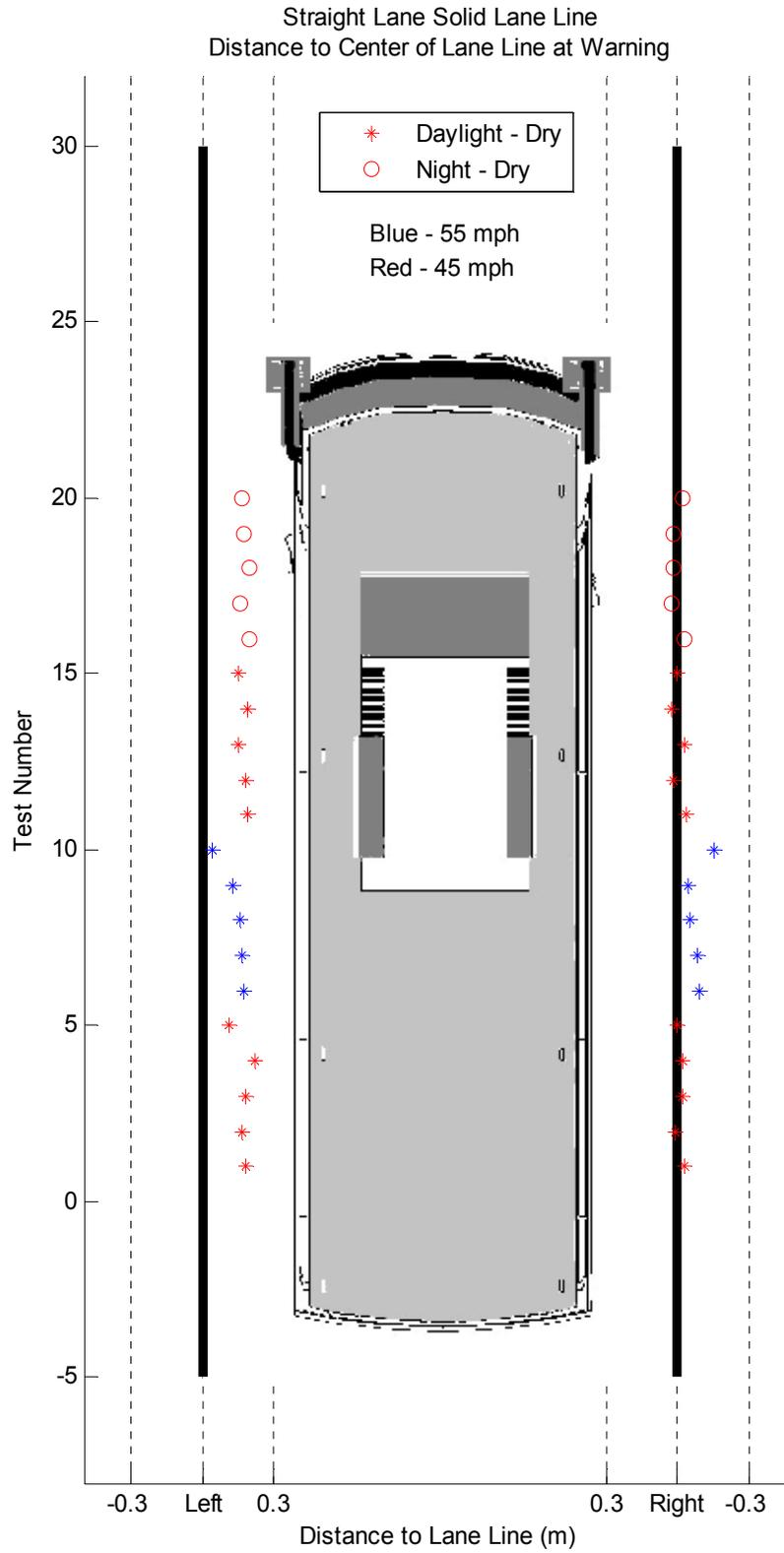
**Figure 3.1 Straight Lane Solid Lane Line – Lateral Distance to Lane Line Distribution at LDW**
