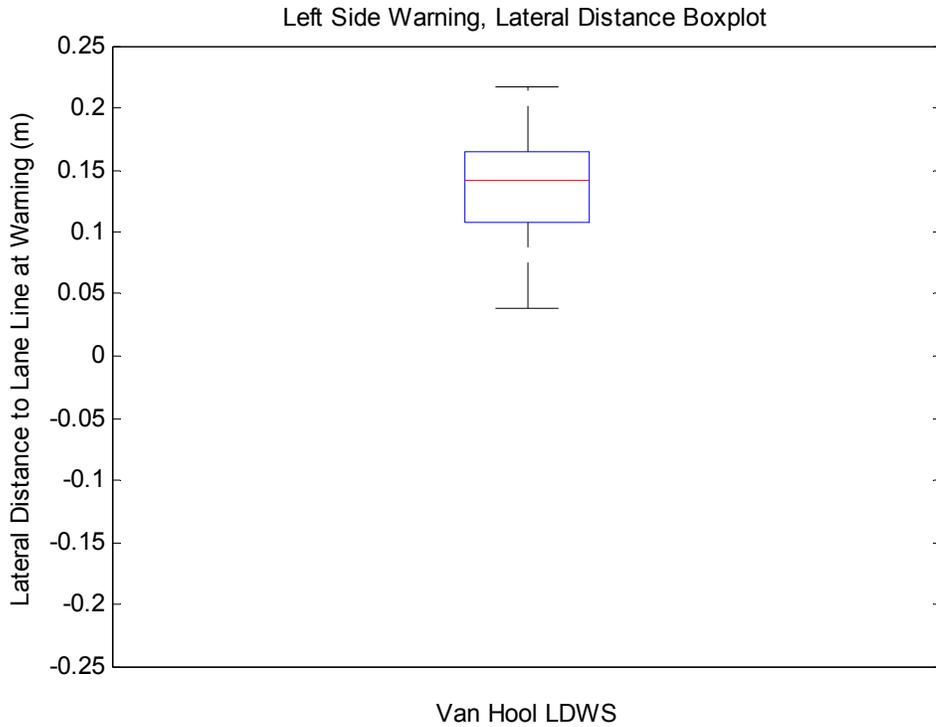
**Figure 3.3** Straight Lane, Left-Side Test – Lateral Distance to Lane Line at Warning-Box Plot
