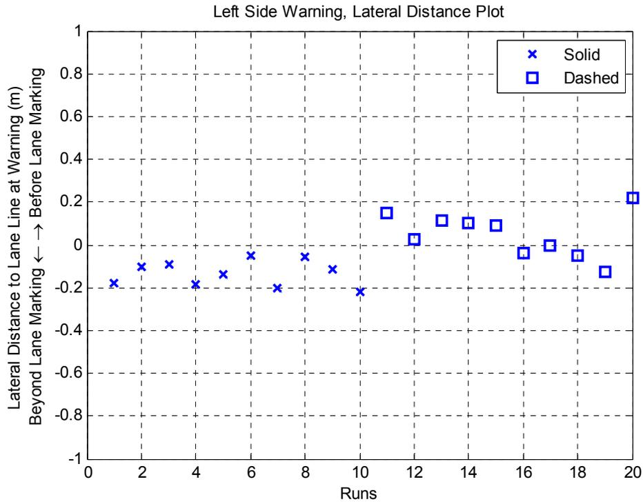
**Figure C.3 Curved Lane, Left-Side Test – Warning Distribution**
