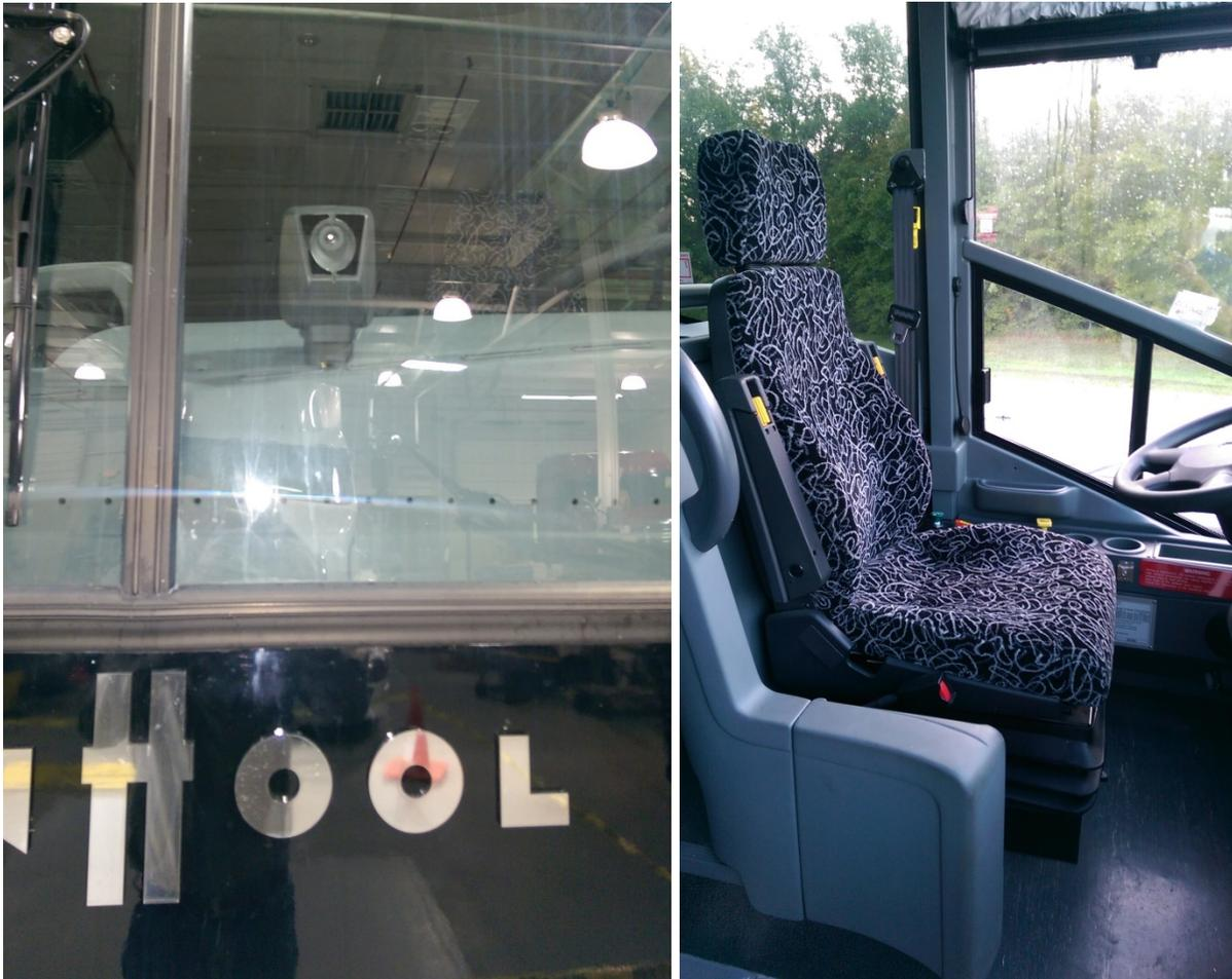
**Figure 2.5 Left: Bendix AutoVue LDW System Video Camera Sensor
