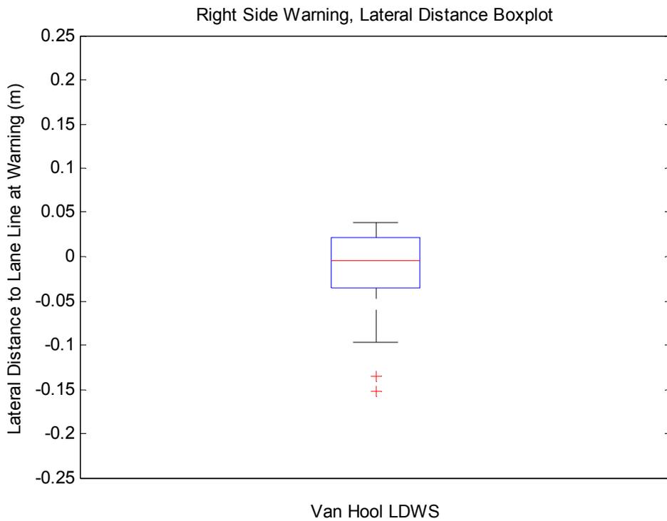
**Figure 3.4** Straight Lane, Right-Side Test – Lateral Distance to Lane Line at Warning-Box Plot
