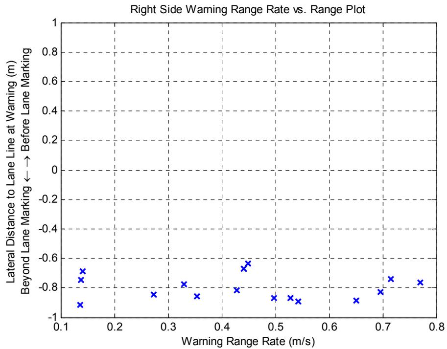
**Figure 3.12 Curved Lane, Right-Side Test – Lateral Distance to Lane Line at Warning Versus Lane Departure Rate Plot**
