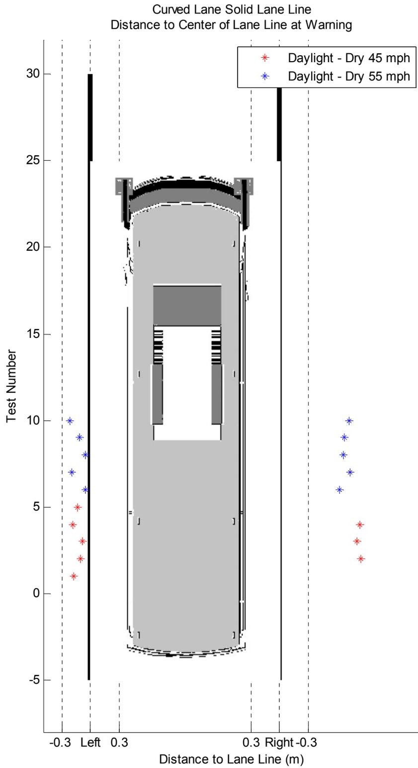
**Figure 3.7 Curved Solid Lane – Warning Distribution**
