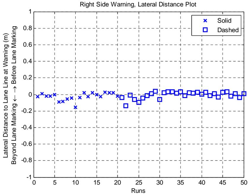
**Figure C.2 Straight Lane, Right-Side Test - Lateral Distance to Lane Line at LDW Distribution**
