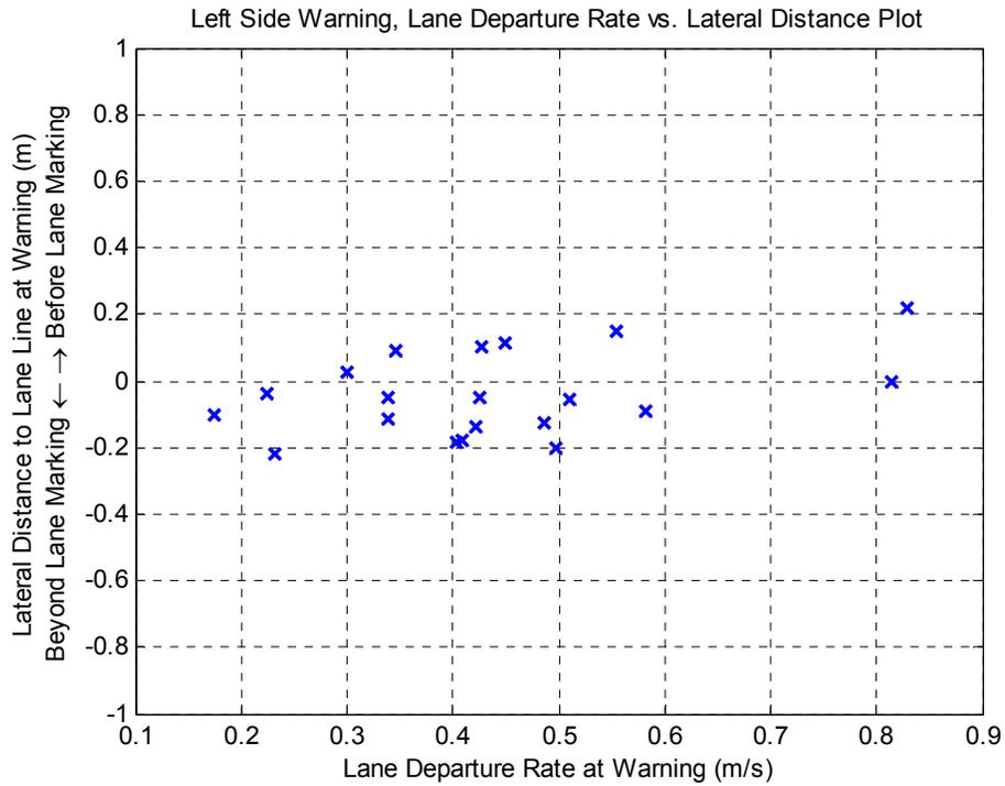
**Figure 3.11 Curved Lane, Left-Side Test – Lateral Distance to Lane Line at Warning Versus Lane Departure Rate Plot**
