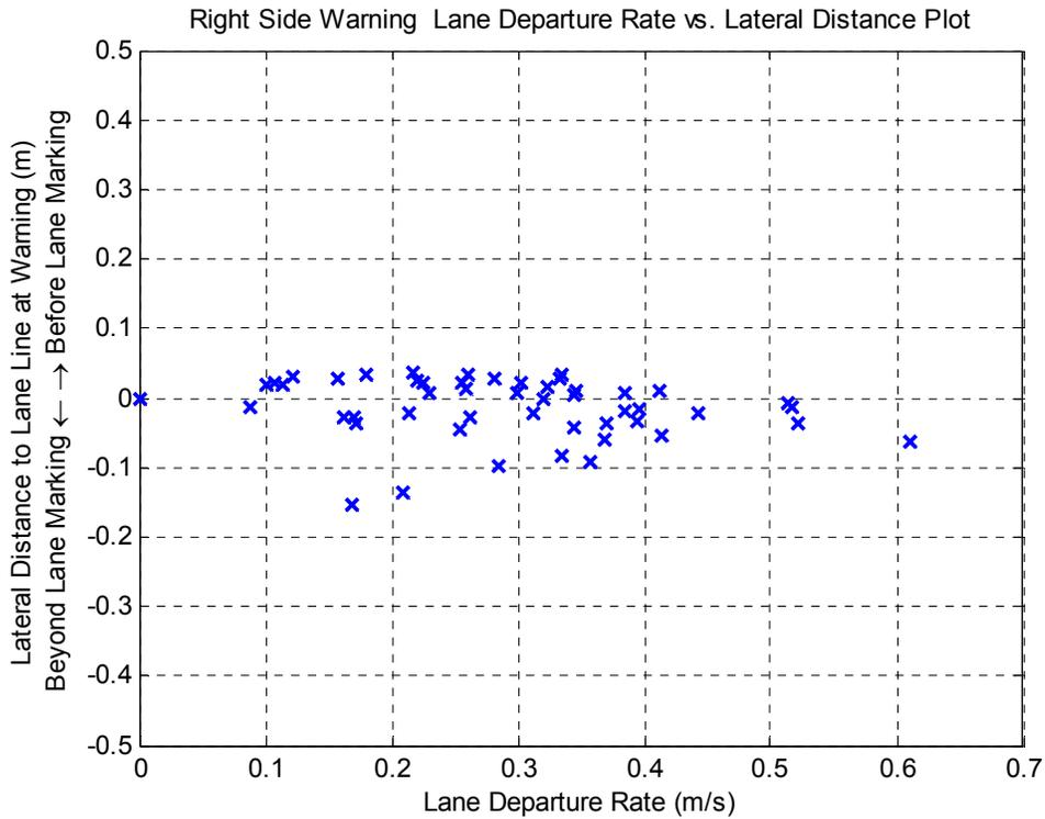
**Figure 3.6 Right-Side Test – Lateral Distance to Lane Line at Warning Versus Lane Departure Rate Plot**
