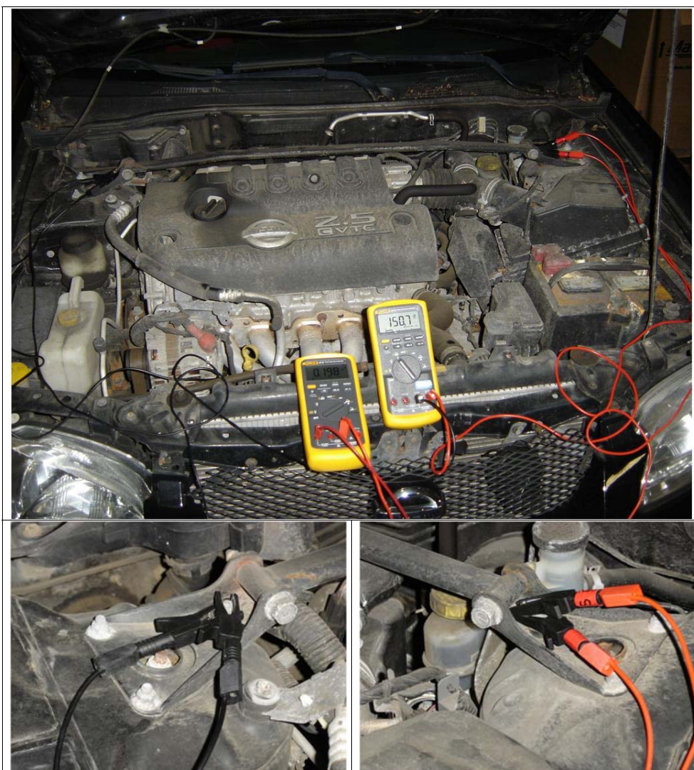
Figure A-4. Pictures of test point locations for the Nissan Sentra circa 2002.
