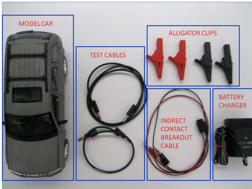
Figure C-1. Demonstration kit car, test cables, test clips and battery charger.
