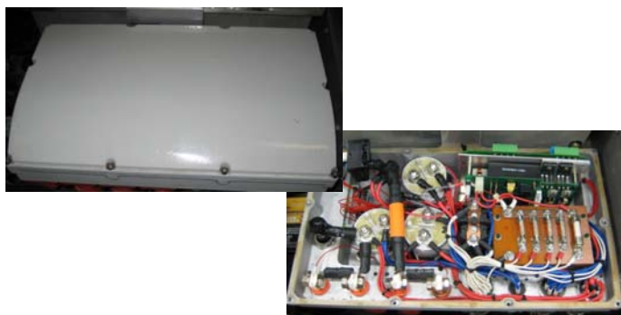
Figure 14. Example of an electrical protective barrier and the electronics components contained within in a prototype fuel cell vehicle.
