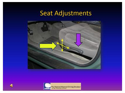
"Once you are seated, please adjust the seat and the steering wheel so you are in a comfortable driving position. Move the power seat lever in the direction that you would like the seat to go. Adjust the angle of the seatback using the long lever."
