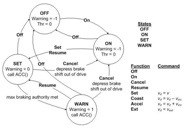
Figure 22: Cruise control state transition diagram
