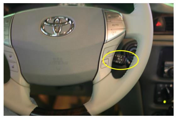
Figure 1: ACC Controls in NADS-1.
