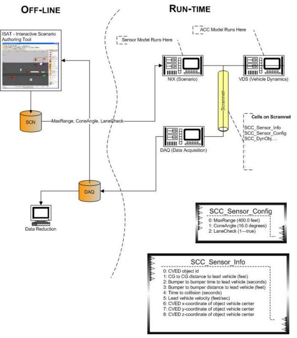
Figure 21: ACC Distributed Model Architecture.
