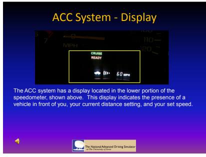
"The ACC system has a display located in the lower portion of the speedometer, shown above. This display indicates the presence of a vehicle in front of you, your current distance setting, and your set speed."
