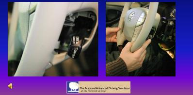
"The ACC system you will use today will be familiar, but not identical, to the ACC in your personal vehicle. The controls for the ACC system are shown below. To turn on the ACC system, press the "ON - OFF" button."
