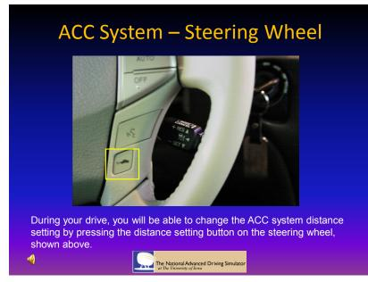
"During your drive, you will be able to change the ACC system distance setting by pressing the distance setting button on the steering wheel, shown above."
