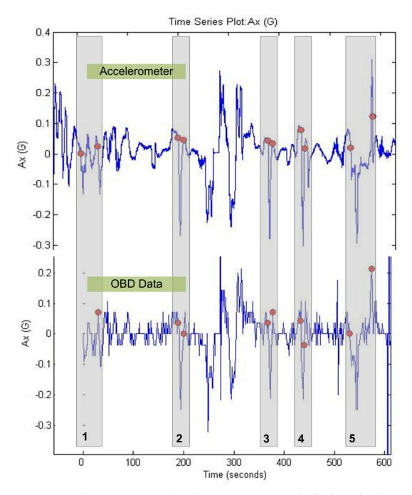
Figure 19: OBD and Accelerometer Data: Longitudinal Acceleration
