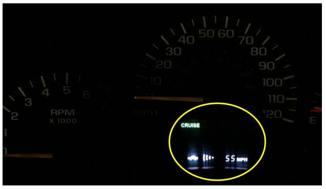
Figure 2: ACC Display in NADS-1.
