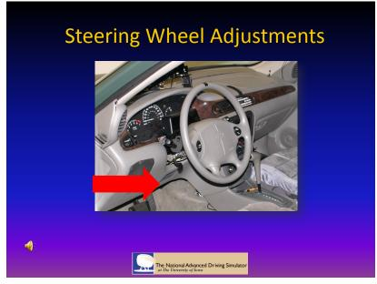
"Adjust the steering wheel so you are comfortable, however, you must be able to view the speedometer by glancing downward rather than by moving your head. (pause) The lever is located above your left knee. It will help the eye tracking process if you adjust the wheel as low as possible while still considering your comfort."
