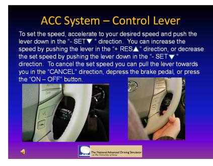
"To set the speed, accelerate to your desired speed and push the lever down in the "- SET down " direction. You can increase the speed by pushing the lever in the "+ RES up " direction, or decrease the set speed by pushing the lever down in the "- SET down " direction. To cancel the set speed you can pull the lever towards you in the "CANCEL" direction, depress the brake pedal, or press the "ON – OFF" button."
