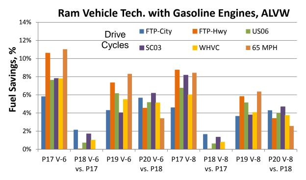
FIGURE 2.24 RAM VEHICLE TECHNOLOGY PACKAGE RESULTS WITH THE BASELINE GASOLINE ENGINES. P18 IS COMPARED TO P17, AND P20 TO P19
