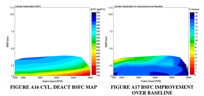
For loads greater than four bar BMEP, the engine turns on all eight cylinders with EGR. The combined maps can be seen below in Figures A 66 and A67.
