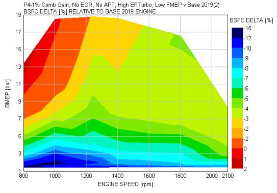
FIGURE B1.5B BSFC IMPROVEMENT MAP OF COMBO PACKAGE 4 ENGINE VS. THE 2019 BASELINE
