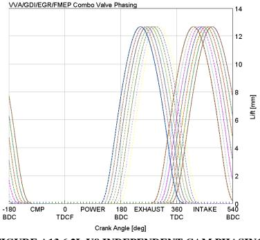
FIGURE A13 6.2L V8 INDEPENDENT CAM PHASING
