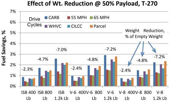
FIGURE 3.8 EFFECT OF EMPTY WEIGHT REDUCTION ON T270
