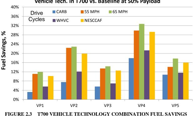
Vehicle Tech. in T700 vs. Baseline at 50% Payload
