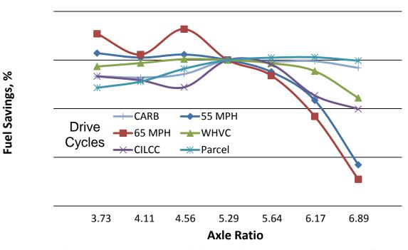
T270 Axle Ratio Sweep w/ ISB, 50% Payload
