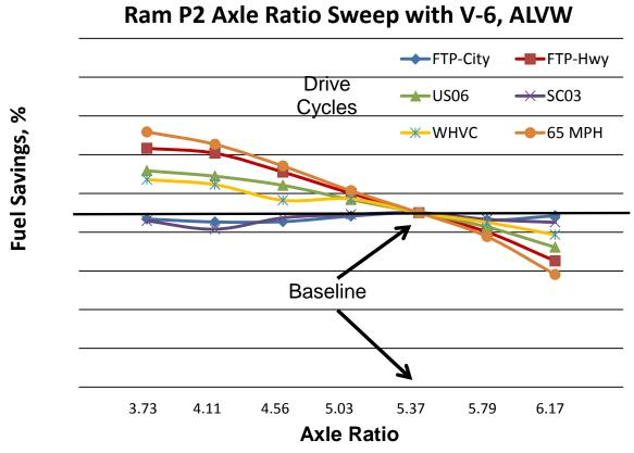
FIGURE 3.17 AXLE RATIO SWEEP ON RAM PICKUP WITH V-6 GASOLINE
