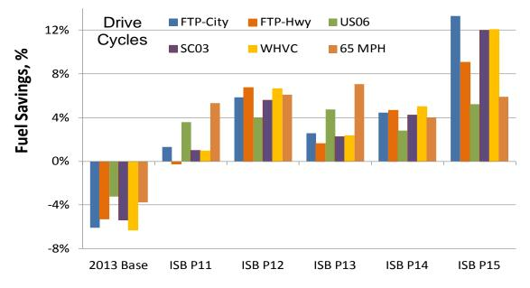
FIGURE 2.19 DIESEL TECHNOLOGY COMBINATIONS IN THE RAM PICKUP
