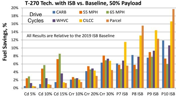
FIGURE 2.17 T270 VEHICLE TECHNOLOGY COMBINATION FUEL SAVINGS RESULTS WITH THE 2019 BASELINE ISB ENGINE. ALL RESULTS ARE RELATIVE TO THE 2019 ISB BASELINE
