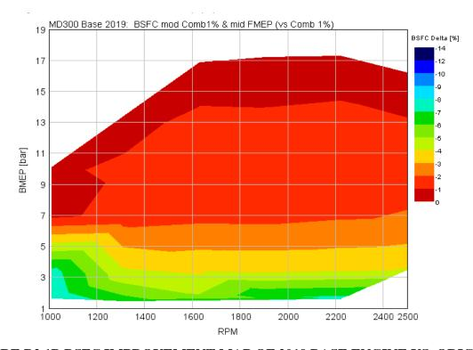
FIGURE B2.1B BSFC IMPROVEMENT MAP OF 2019 BASE ENGINE VS. ORIGINAL MEDIUM DUTY ISB
