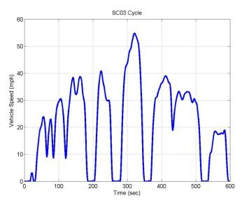
FIGURE C13 SC03 AIR CONDITIONER DRIVE CYCLE
