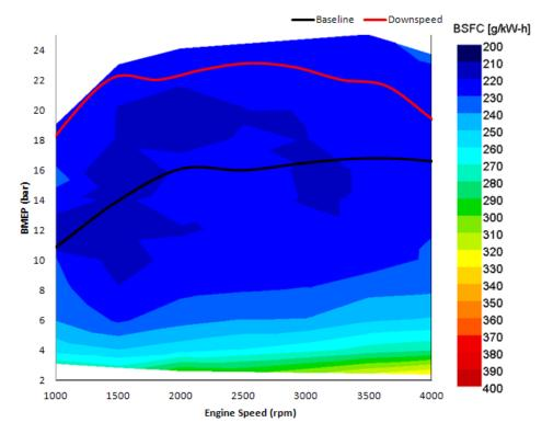
FIGURE A3 BMEP COMPARISON OF STANDARD AND DOWN SPEED TORQUE CURVES
