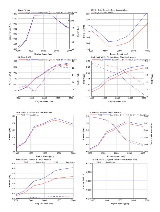
FIGURE B3.3C PACKAGE 12 FULL LOAD PERFORMANCE COMPARISON
