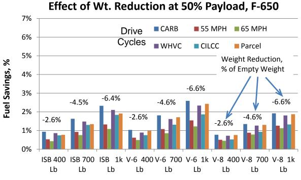
FIGURE 3.7 EFFECT OF EMPTY WEIGHT REDUCTION ON F-650
