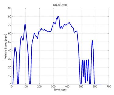
FIGURE C12 US06 AGGRESSIVE LIGHT DUTY DRIVE CYCLE
