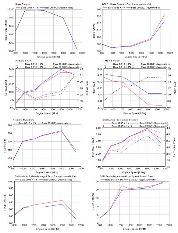
FIGURE B1.1D 2019 BASE ENGINE COMPARISON WITH ORIGINAL DD15 (BOTH FEATURING IMPROVED COMBUSTION)
