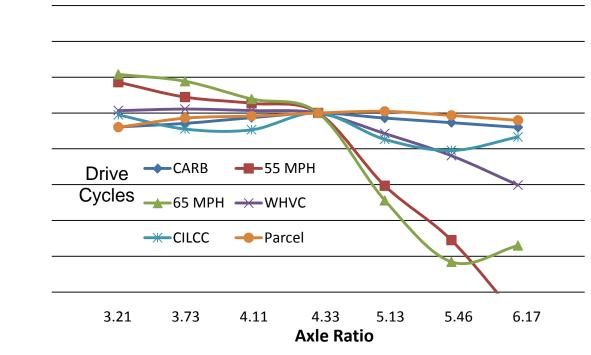
F-650 Axle Ratio Sweep w/ ISB, 50% Payload
