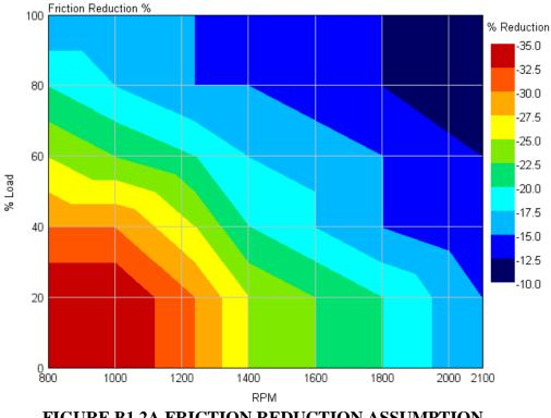
FIGURE B1.2A FRICTION REDUCTION ASSUMPTION
