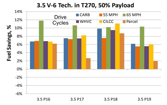
FIGURE 2.12 FUEL SAVING PERFORMANCE OF ISB TECHNOLOGY PACKAGES IN THE T270 TRUCK
