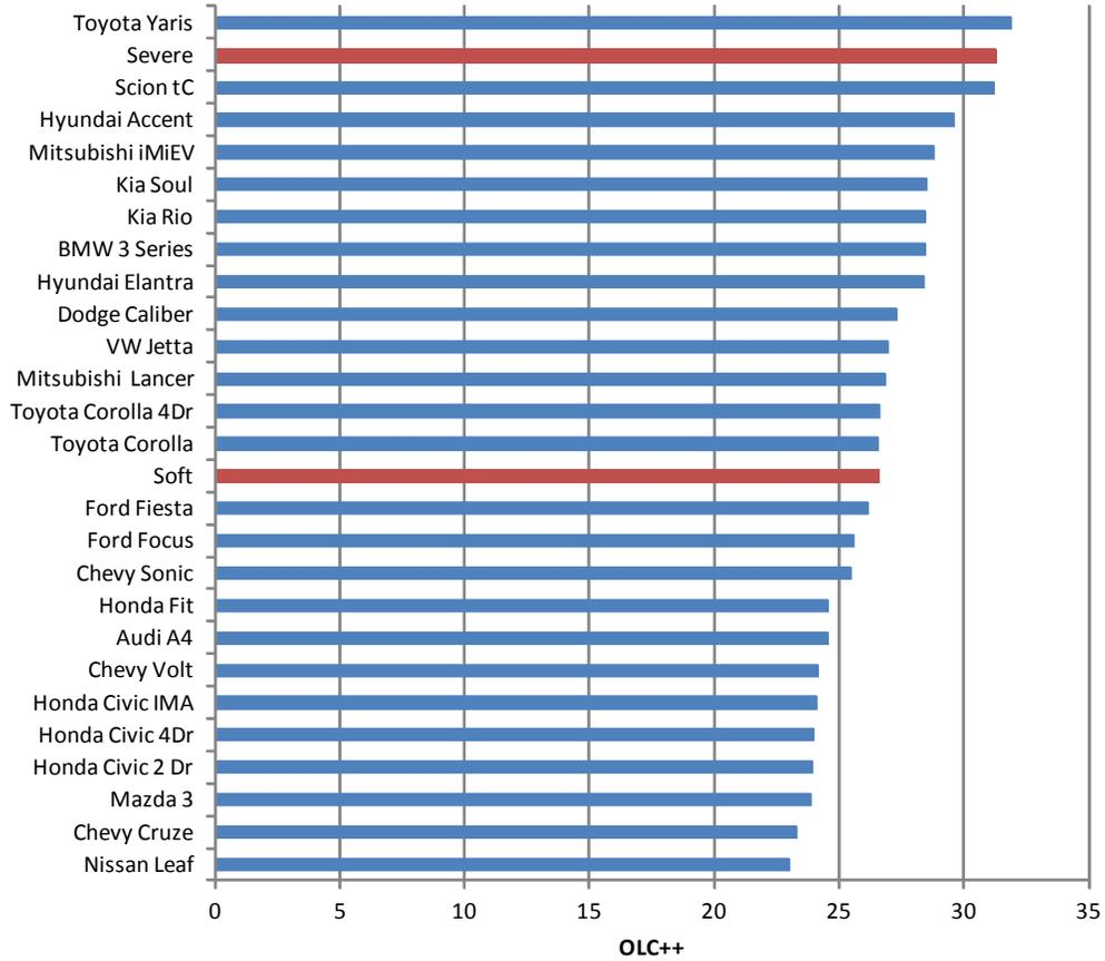
Figure 5: NCAP pulse severity ranking based on 25 small cars
