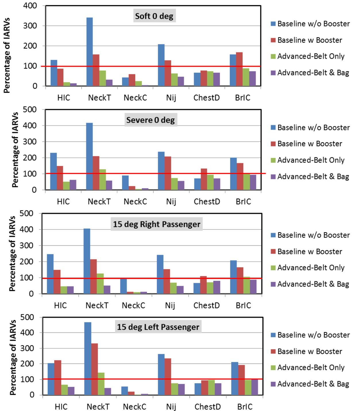
Figure 28: 6YO ATD injury measures with four restraints at four crash conditions
