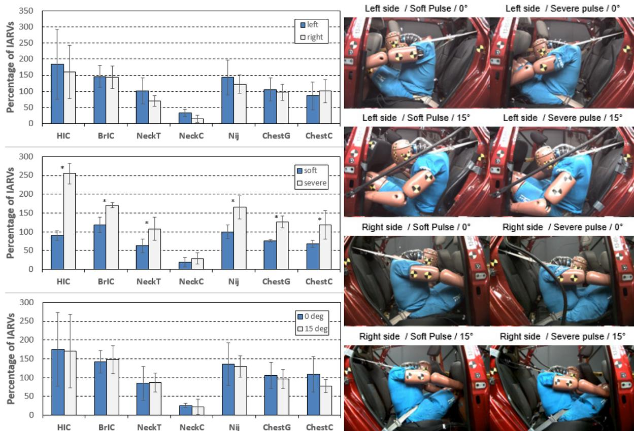
Figure 7: 95th ATD injury measures and kinematics at maximum head excursion
