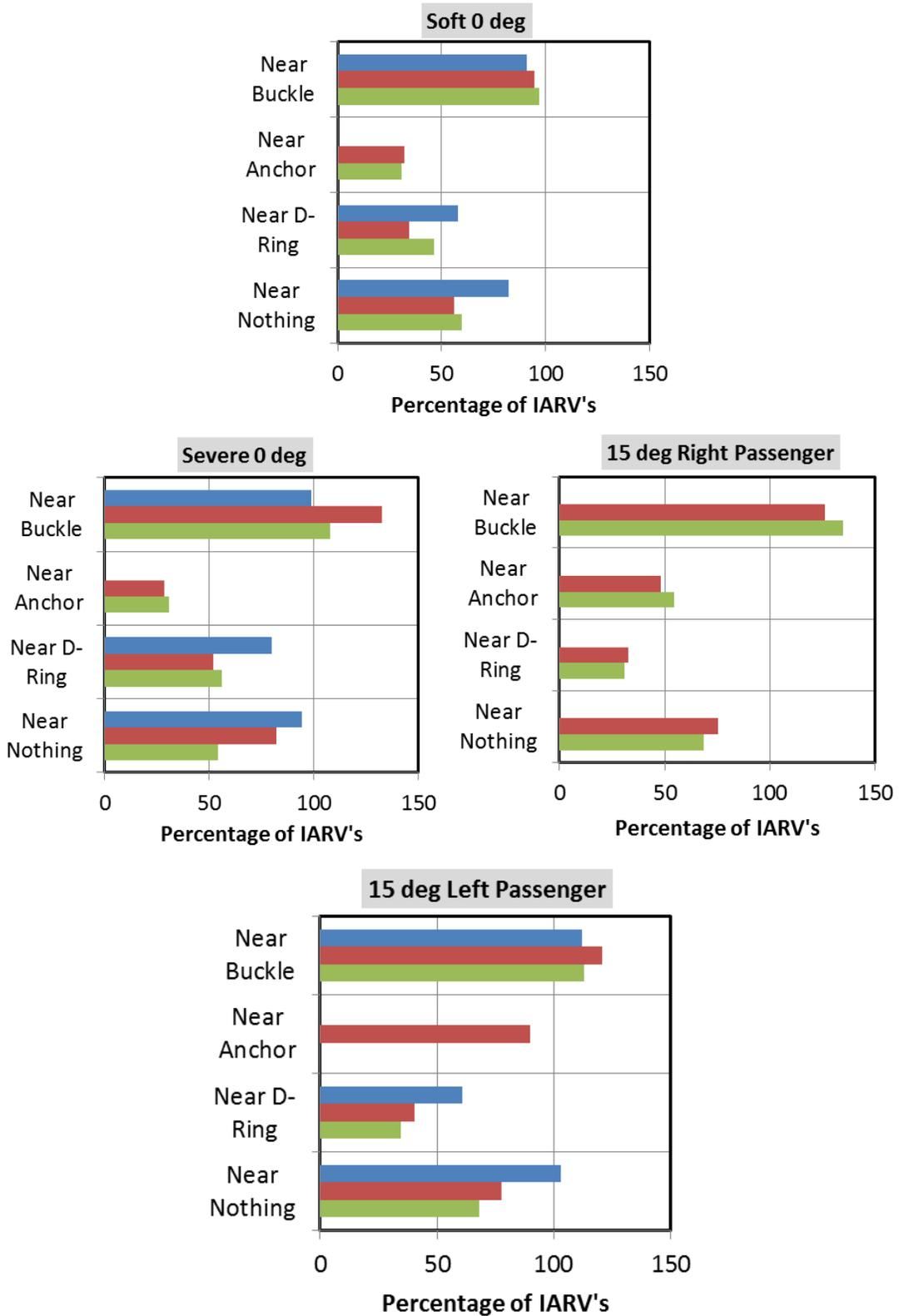
Figure 33: THOR 50th chest deflections at four locations with three restraints at four crash conditions
