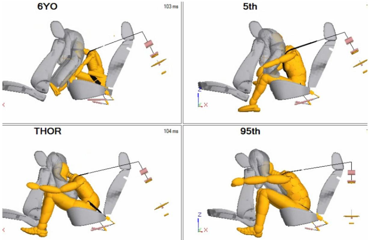
Figure 25: Driver side ATD kinematics with an advanced belt system (3-point belt with 9.0 mm torsion bar, retractor and anchor pretensioners) and a SCaRAB under severe crash pulse at 0 deg crash angle
