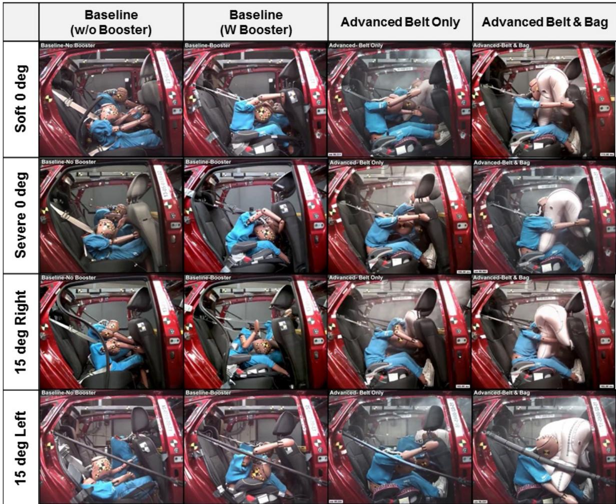
Figure 27: 6YO ATD kinematics with four restraints at four crash conditions
