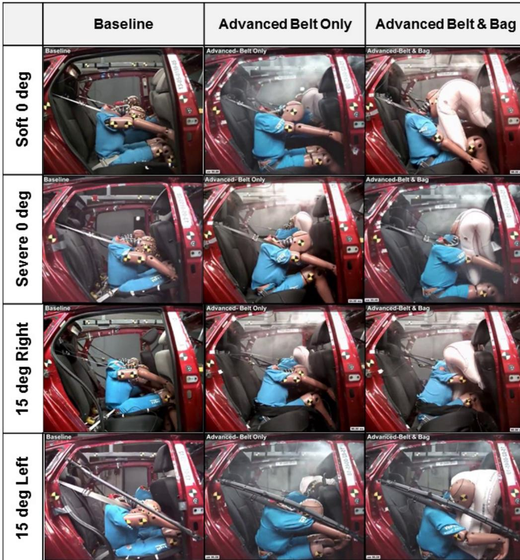
Figure 29: 5th ATD kinematics with three restraints at four crash conditions
