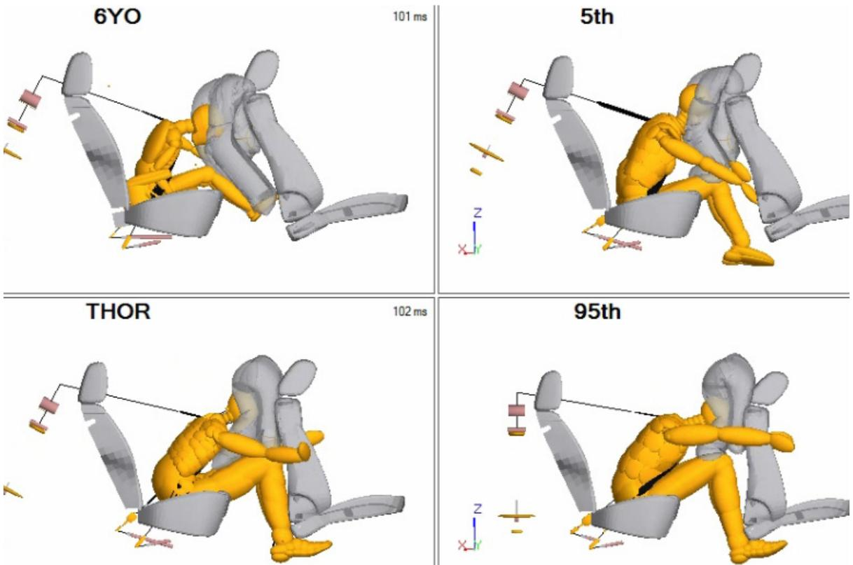
Figure 26: Passenger side ATD kinematics with an advanced belt system (3-point belt with 9.0 mm torsion bar, retractor and anchor pretensioners) and a SCaRAB under severe crash pulse at 0 deg crash angle
