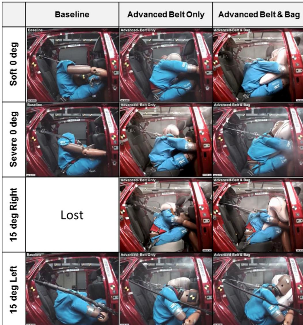
Figure 31: THOR 50th kinematics with three restraints at four crash conditions
