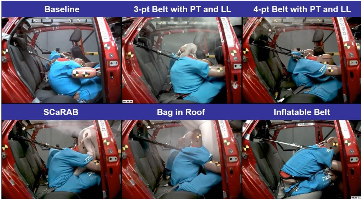
Figure 20: THOR 50th kinematics with different restraint systems
