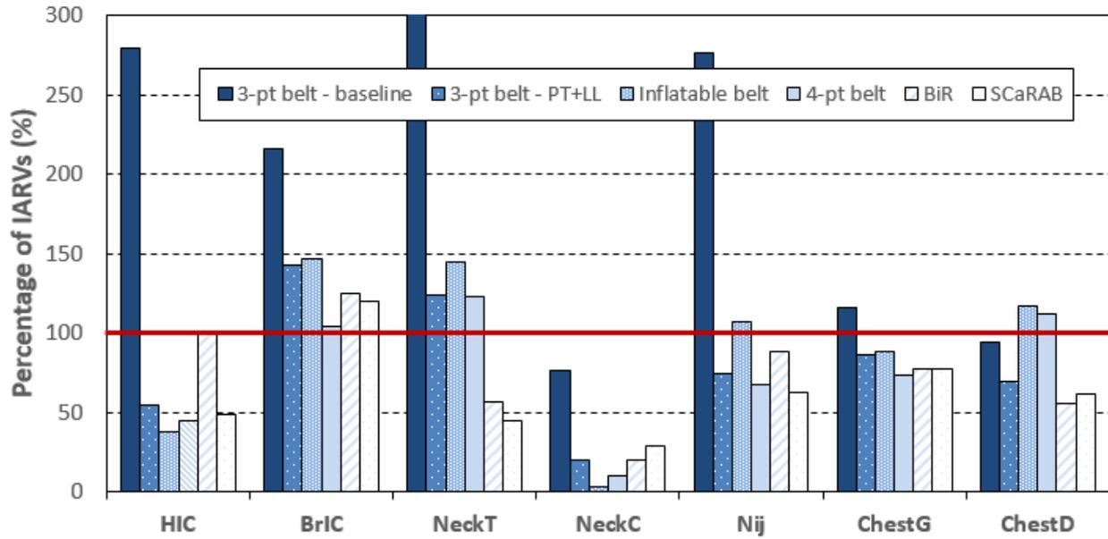
Figure 17: Injury measures for the 6YO ATD with different restraint systems
