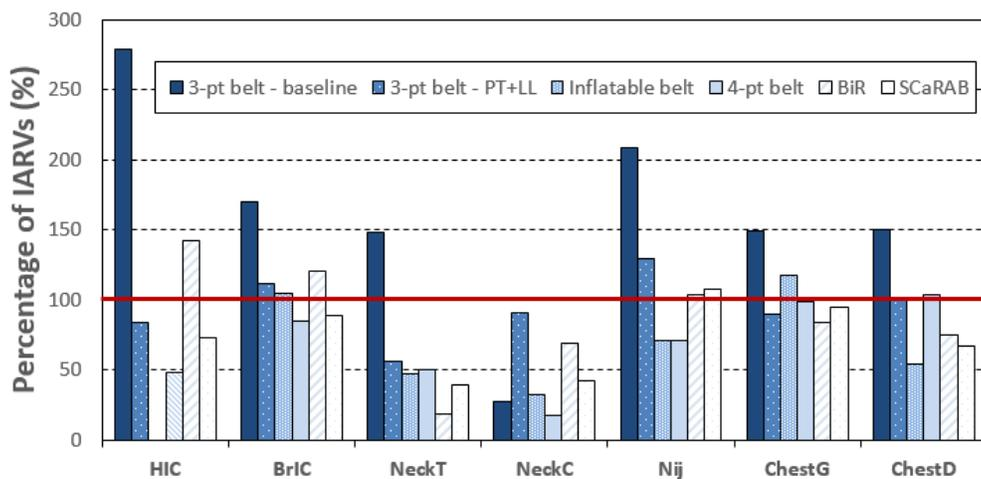
Figure 21: Injury measures for the 95th ATD with different restraint systems
