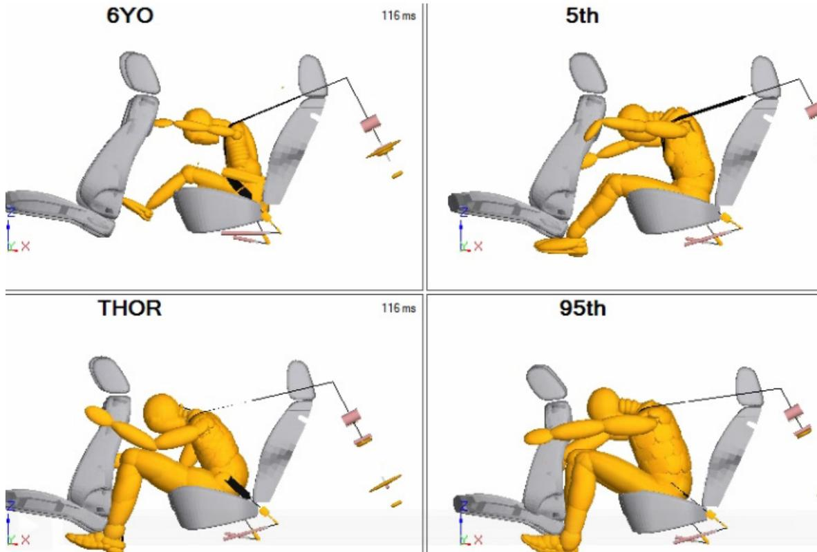
Figure 24: ATD kinematics with the belt-only design 122 (3-point belt with 9.0 mm torsion bar, DLT, and retractor and buckle pretensioners) under soft crash pulse at 0 deg crash angle
