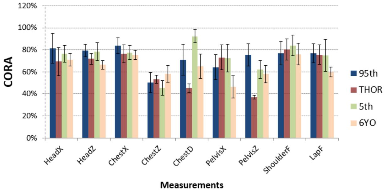
Figure 13: Summary of the CORA scores for the model validation against baseline tests
