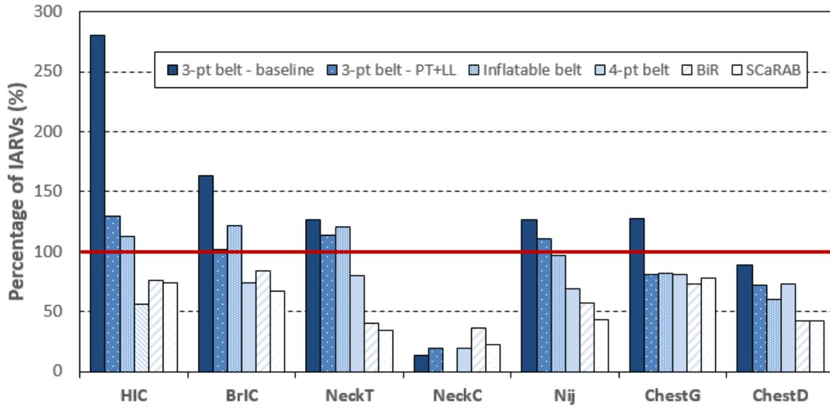
Figure 15: Injury measures for the 5th ATD with different restraint systems
