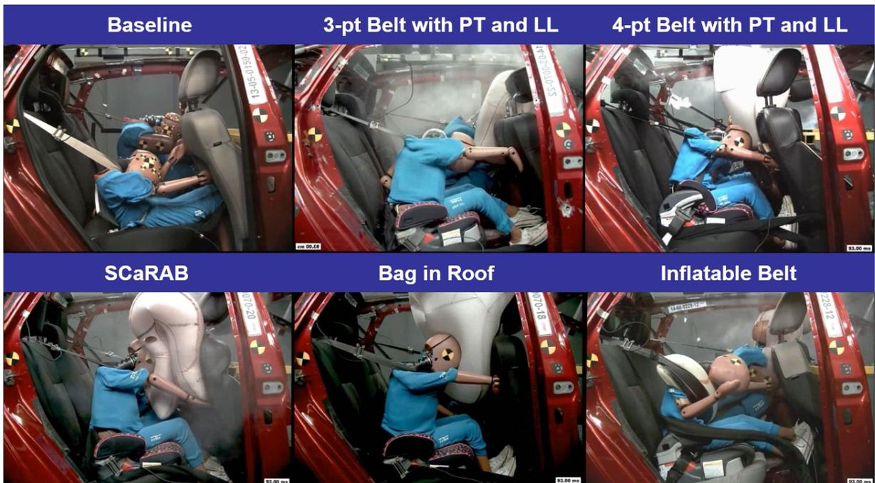
Figure 18: 6YO ATD kinematics with different restraint systems
