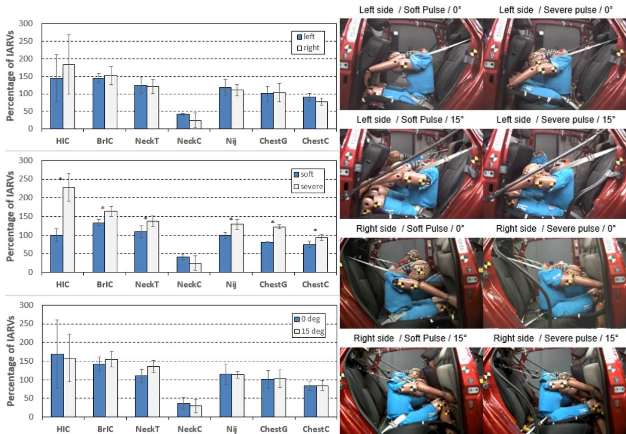
Figure 9: 5th ATD injury measures and kinematics at maximum head excursion
