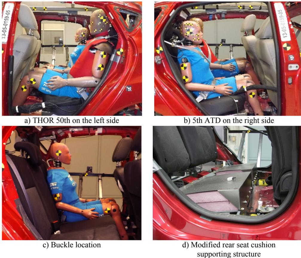
Figure 3: Belt position relative to the ATDs and modified rear seat cushion supporting structure
