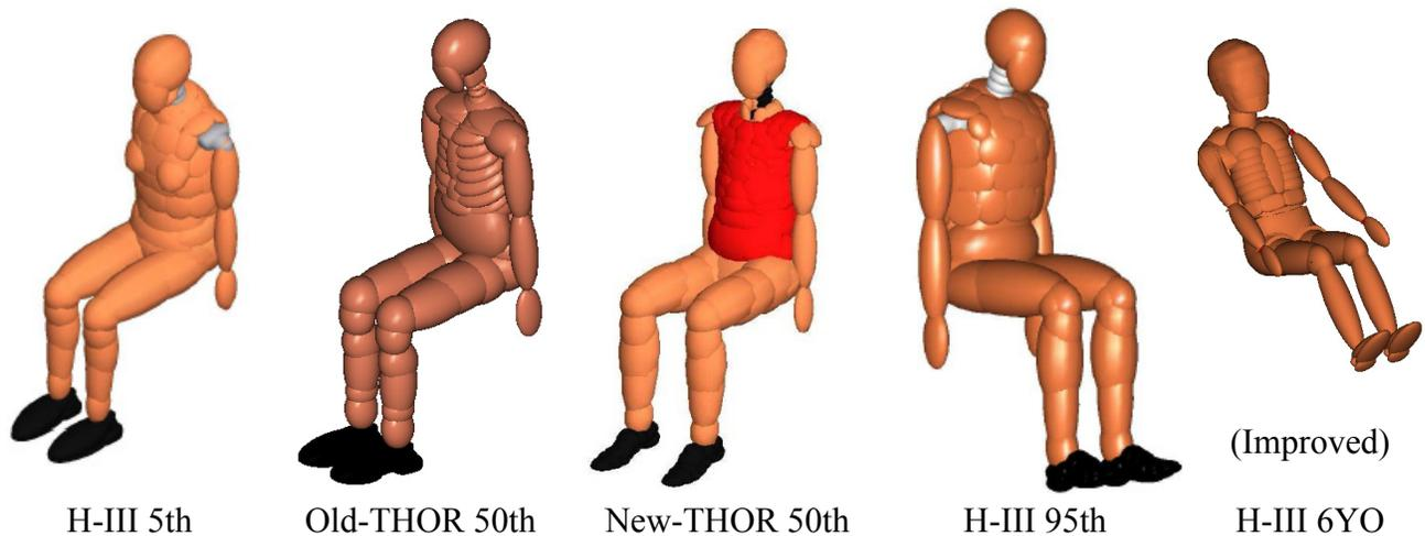
Figure 11: ATD models used in this study
