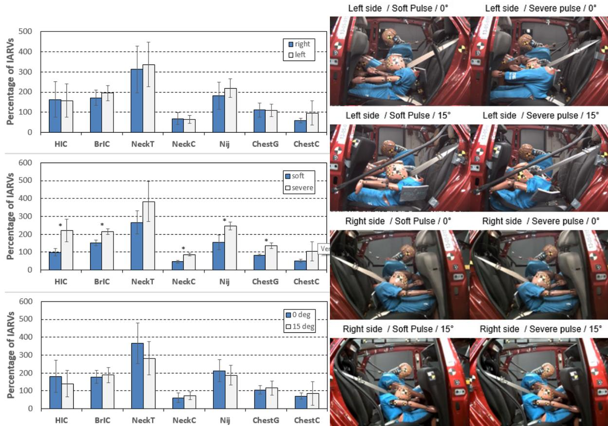
Figure 10: 6YO ATD injury measures and kinematics at maximum head excursion
