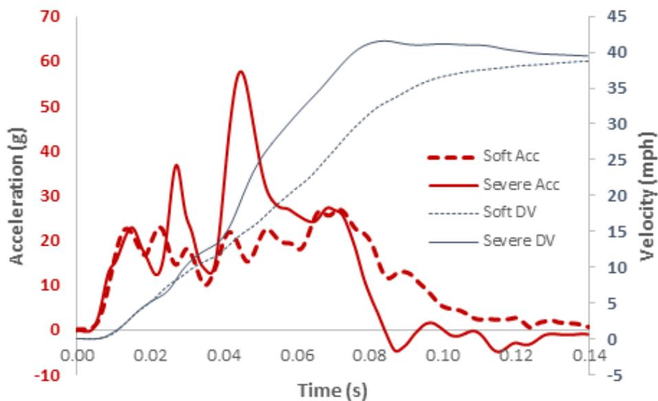
Figure 4: Soft and severe crash pulses based on NCAP tests
