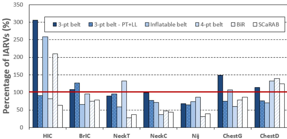
Figure 19: Injury measures for the THOR 50th with different restraint systems
