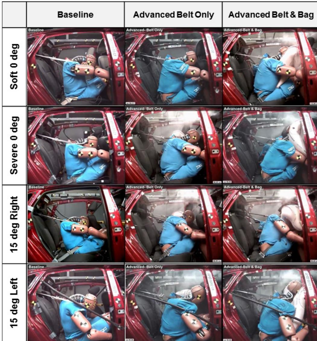
Figure 34: 95th ATD kinematics with three restraints at four crash conditions
