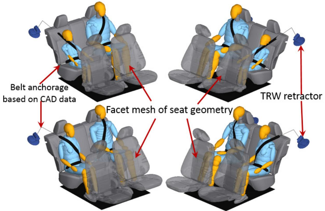
Figure 12: Four sets of models developed for model validation against baseline tests
