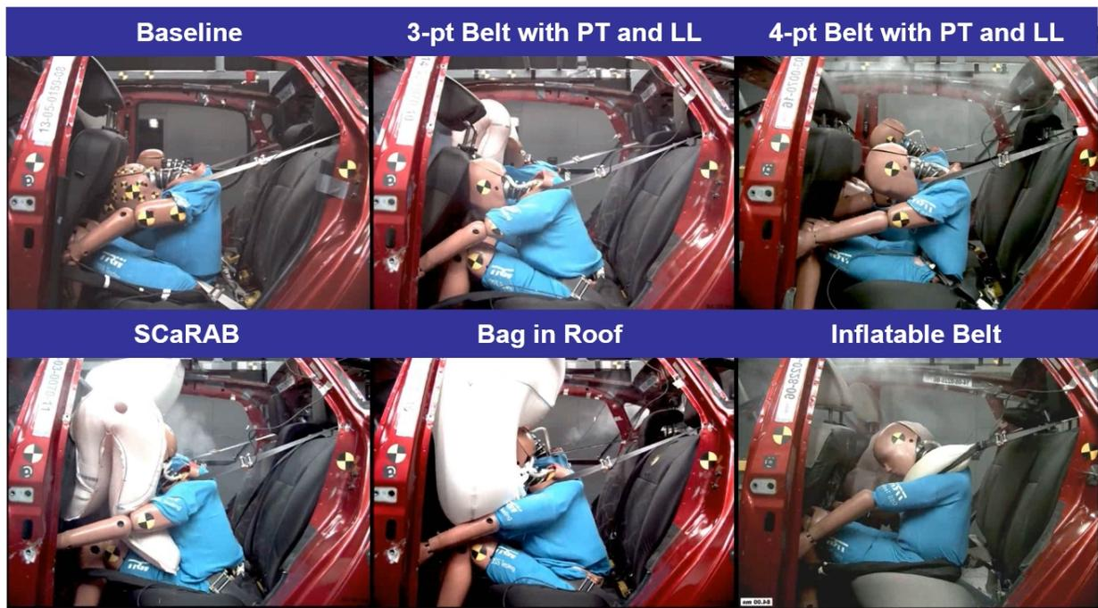
Figure 16: 5th ATD kinematics with different restraint systems
