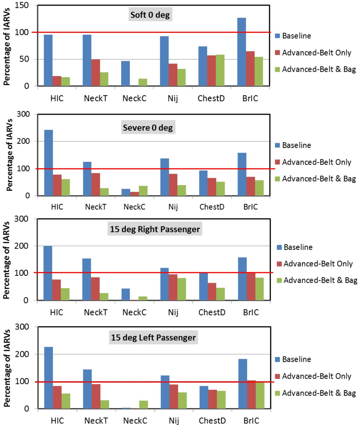
Figure 30: 5th ATD injury measures with three restraints at four crash conditions
