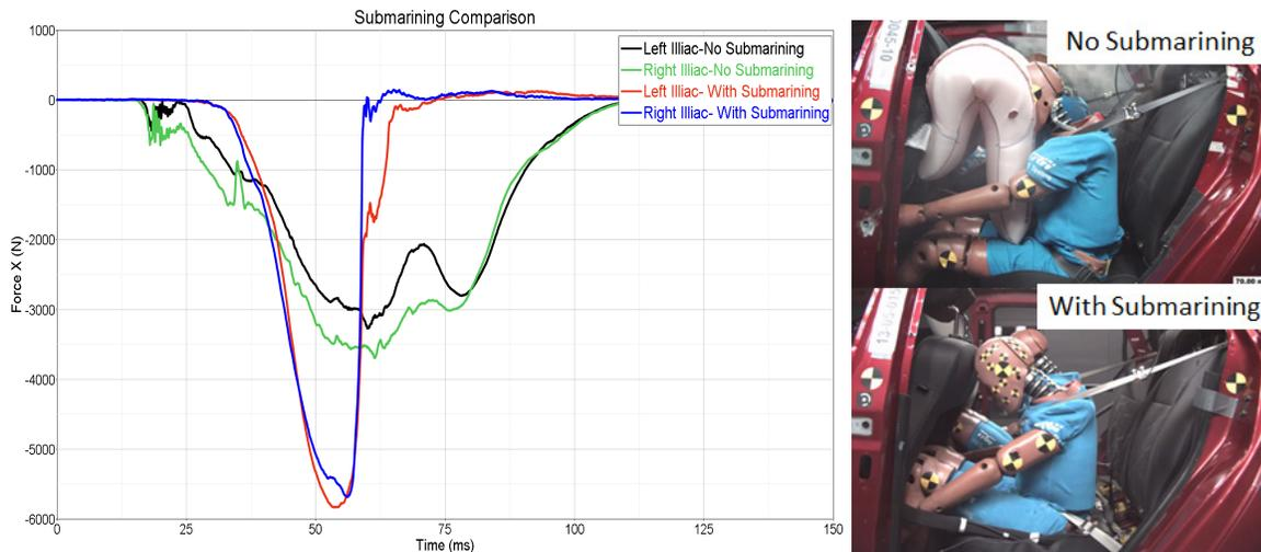
Figure 6: Examples of iliac loads and ATD kinematics with and without submarining
