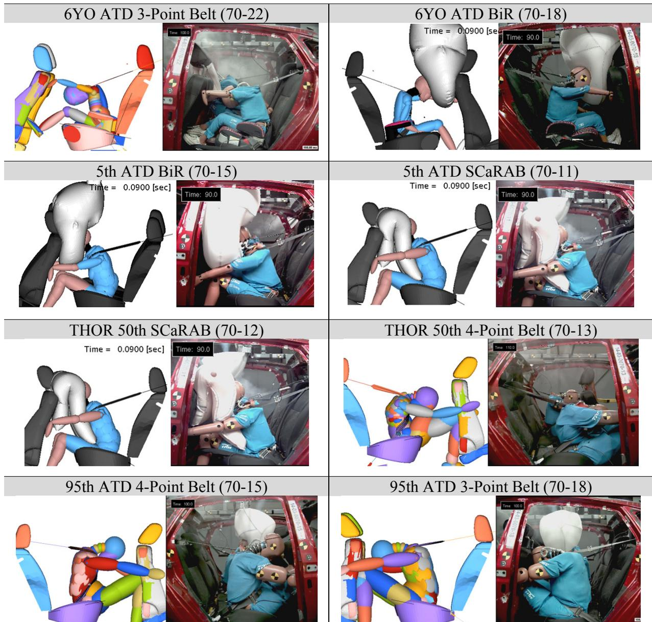
Figure 23: Comparison of ATD kinematics between the tests and simulations with advanced restraints
