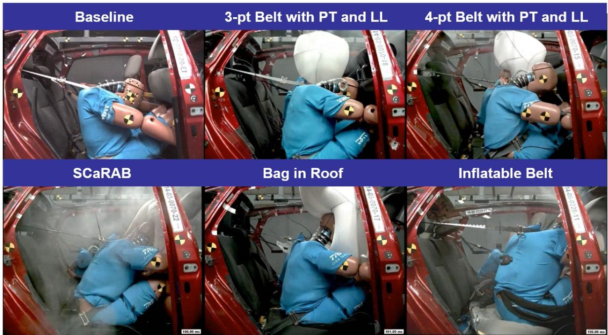
Figure 22: 95th ATD kinematics with different restraint systems
