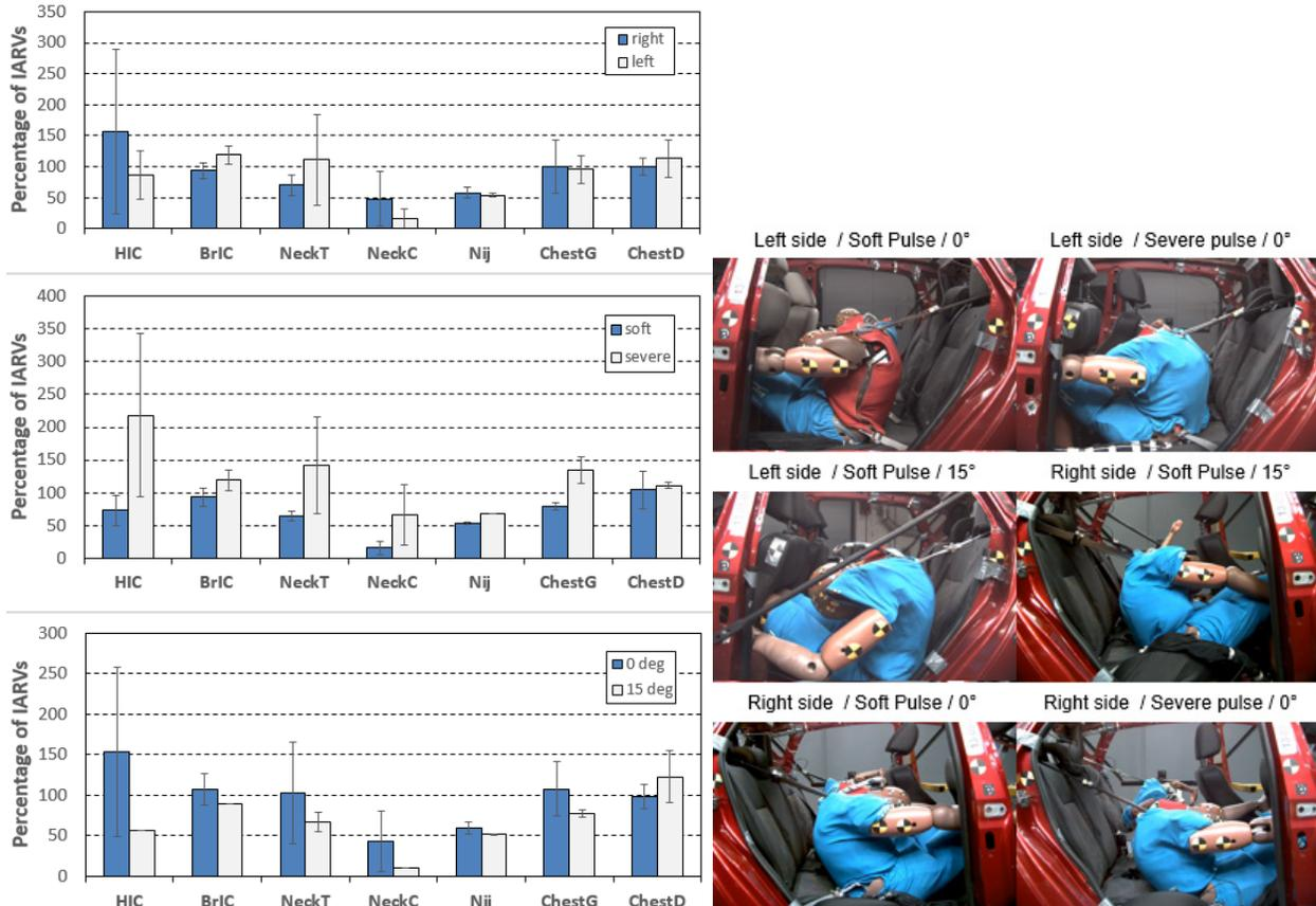
Figure 8: THOR 50th injury measures and kinematics at maximum head excursion (110ms for soft pulse, and 92ms for severe pulse) (T-test was not conducted due to small sample size)
