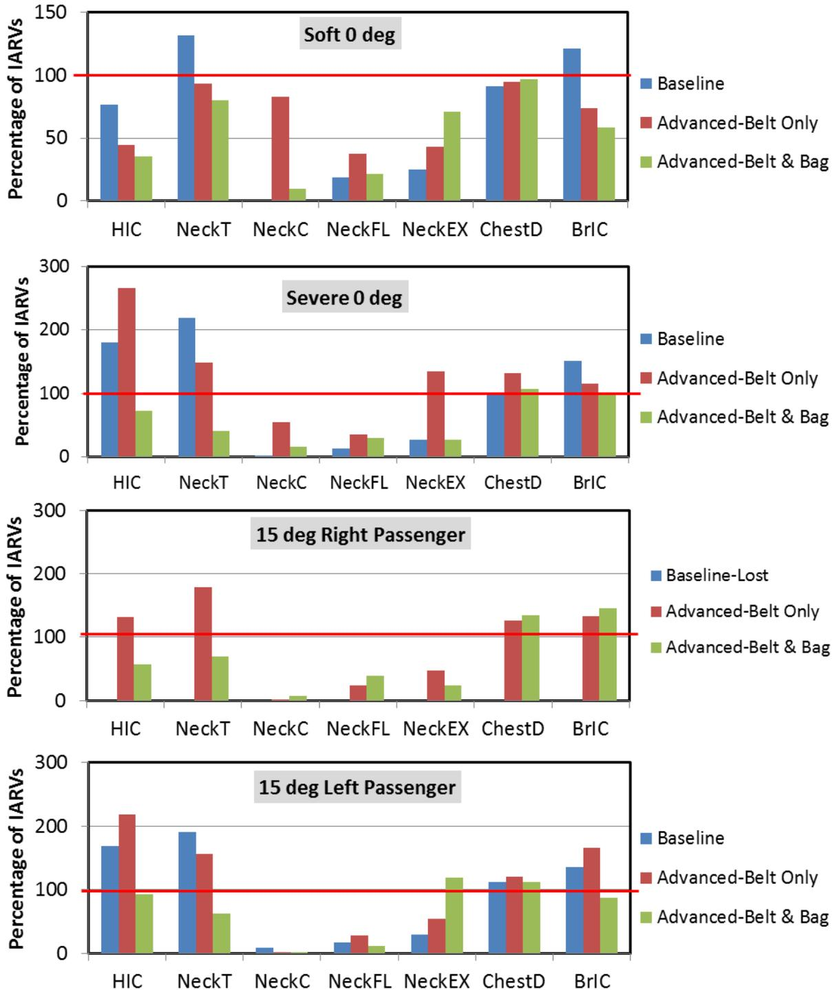
Figure 32: THOR 50th injury measures with three restraints at four crash conditions
