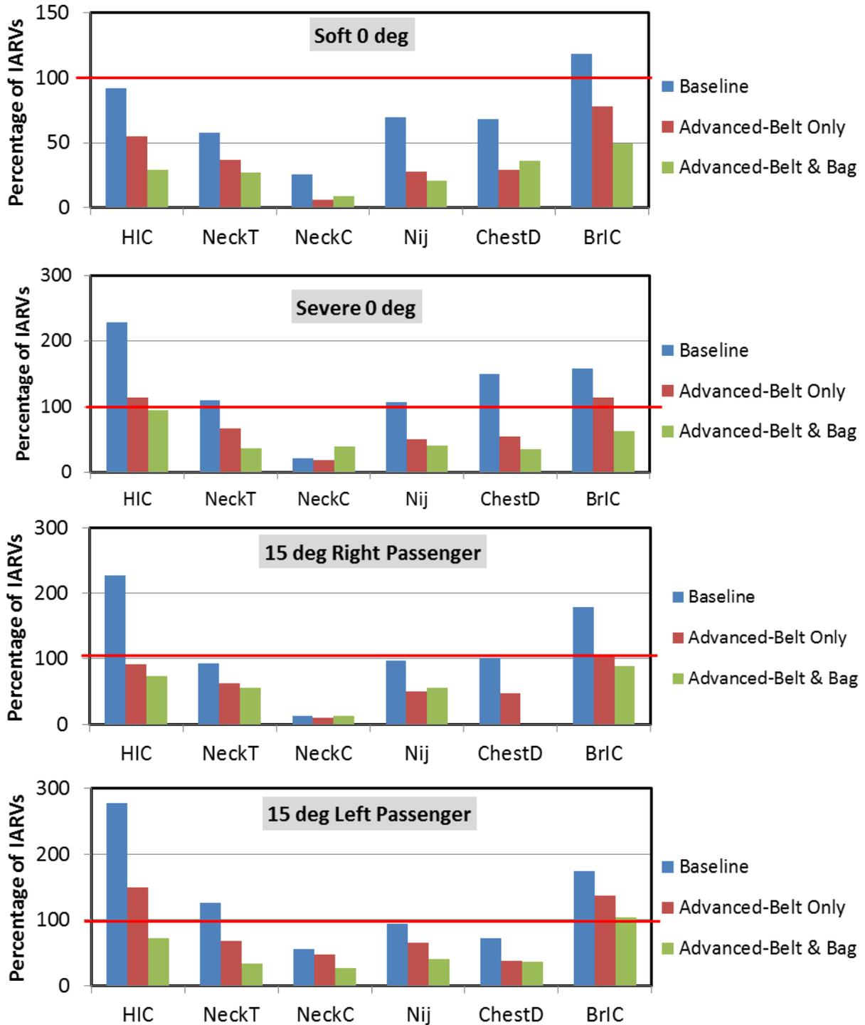
Figure 35: 95th ATD injury measures with three restraints at four crash conditions
