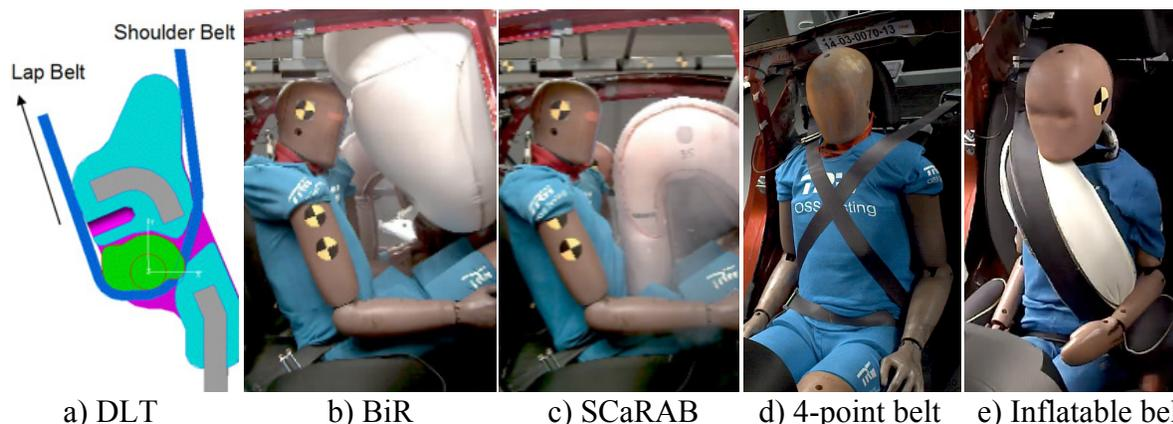
Figure 14: Different advanced restraint systems evaluated in this study
