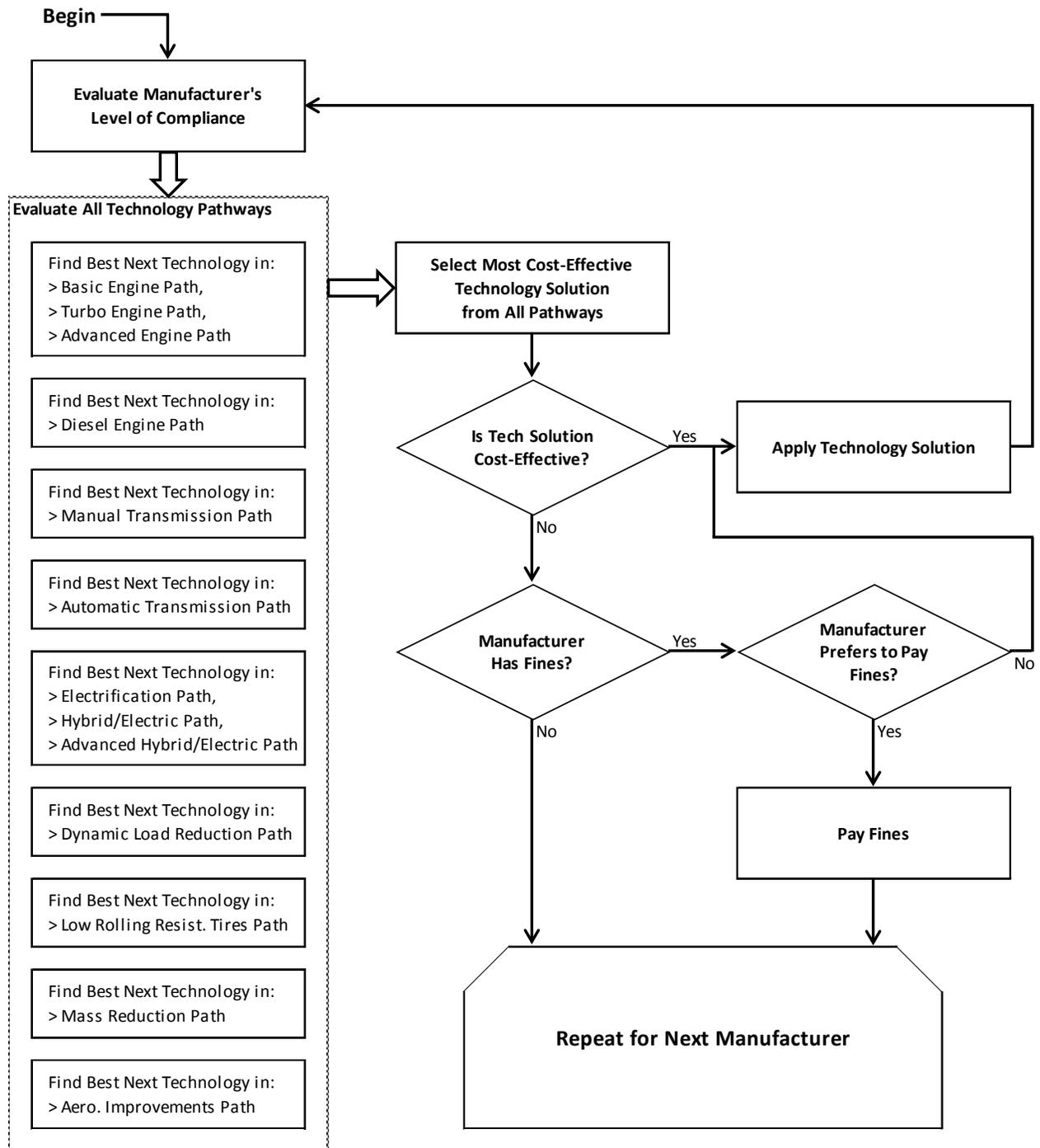
**Figure 7. Compliance Simulation Algorithm**
