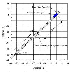
Figure 4. Behavior of Car A near the collision point.
