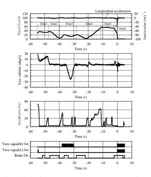
Figure 2. Accident data collected by Recorder-A.
