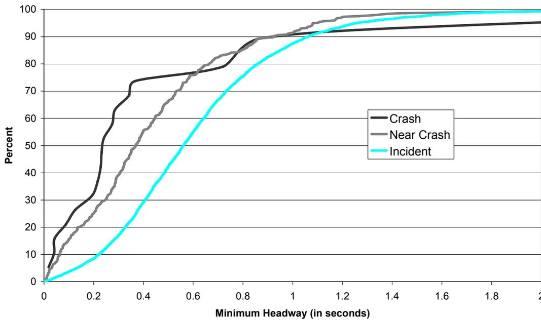
**Figure 19. Distribution of Minimum Headways by Severity Level (3 s before closest headway).**
