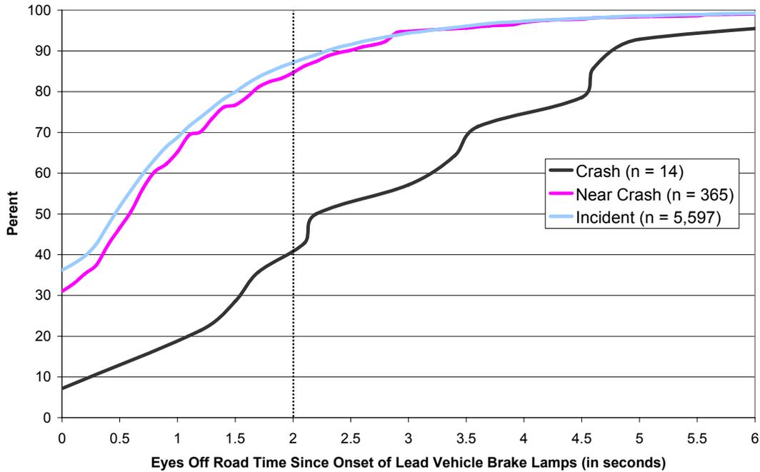
Figure 10. Distribution of Driver EOR Times (in Seconds) Since Onset of Lead-Vehicle Brake Lamps. Only Includes Conflict With Lead Vehicle Cases
