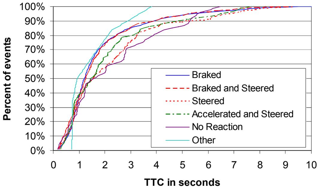
**Figure 27. Distribution of FV-driver responses based on minimum TTC to lead vehicle.**
