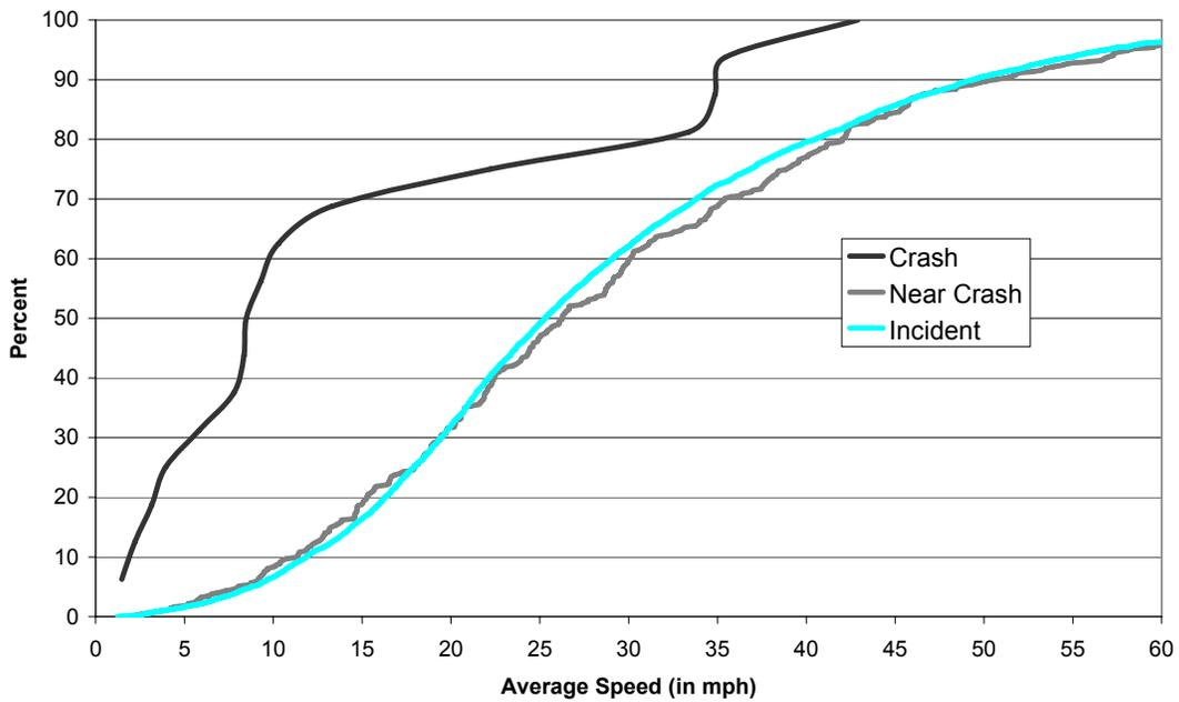
**Figure 17. Distribution of Average Speed by Severity Level (3 s before closest headway).**
