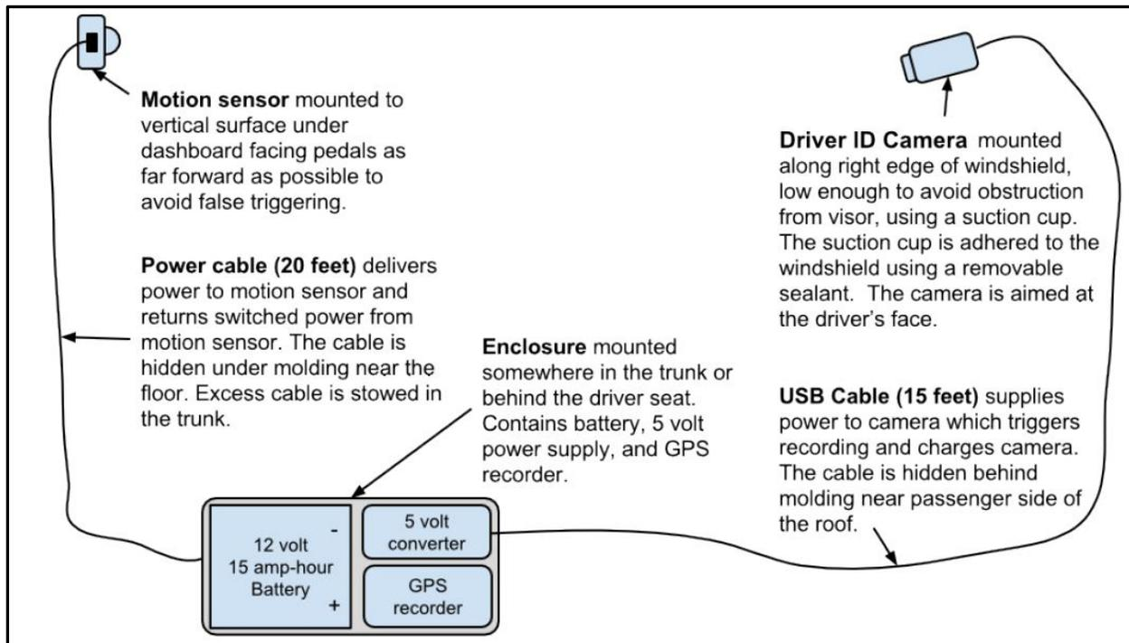
Figure 3. Vehicle Instrumentation.
