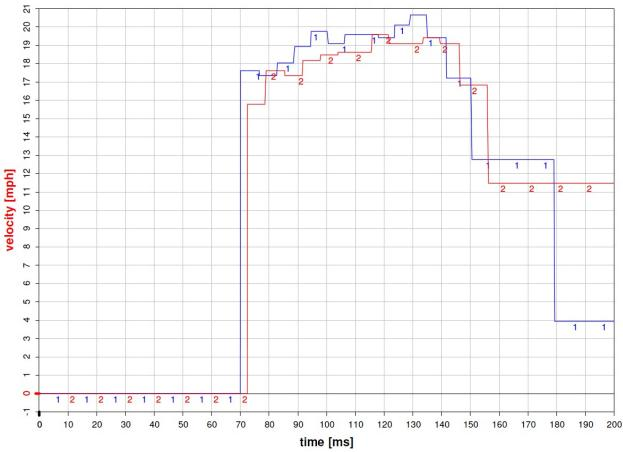
Figure 18: Velocity of the secondary carriage for two 19.0 mph tests as measured by a multi-pass proximity sensor
