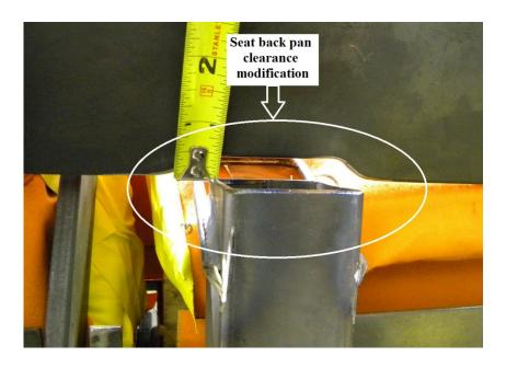
Figure 7: Modification to the seat back pan
