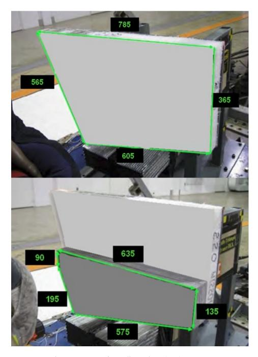
Figure B2: Door foam dimensions (mm)  $\pm$  6 mm
