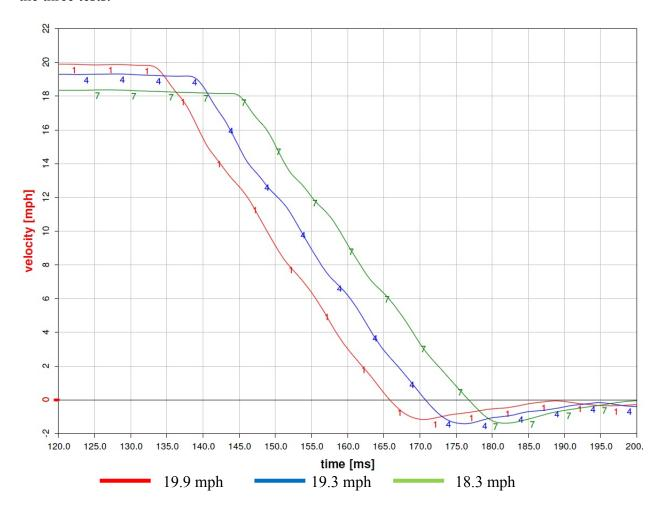
Figure 23: Relative velocity time histories for side impact tests conducted at varying speeds (tests conducted with the 225 lb secondary carriage)
