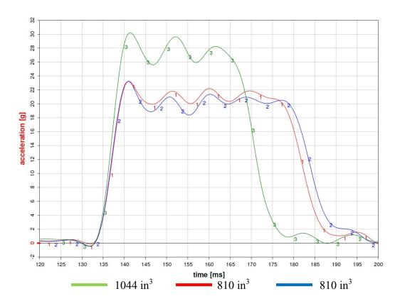
Figure 29: Acceleration of the secondary carriage for varied aluminum honeycomb volume
