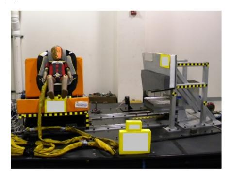
Figure B1: Front view of side impact fixture attached to the deceleration sled
