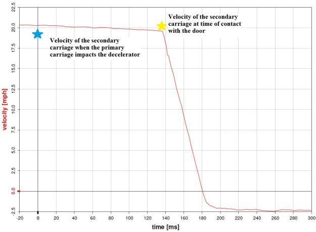
Figure 17: Velocity of the secondary carriage during a "typical" test
