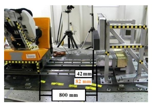
Figure 31: Standard (42 mm) and varied (82 mm) alignment of the honeycomb face from the plane of the door face
