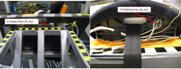
Figure 9: Instrumentation locations
