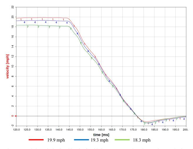
Figure 24: Relative velocity time histories for side impact tests conducted at varying speeds, time shifted to align time-of-impact with the door (tests conducted with the 225 lb secondary carriage)
