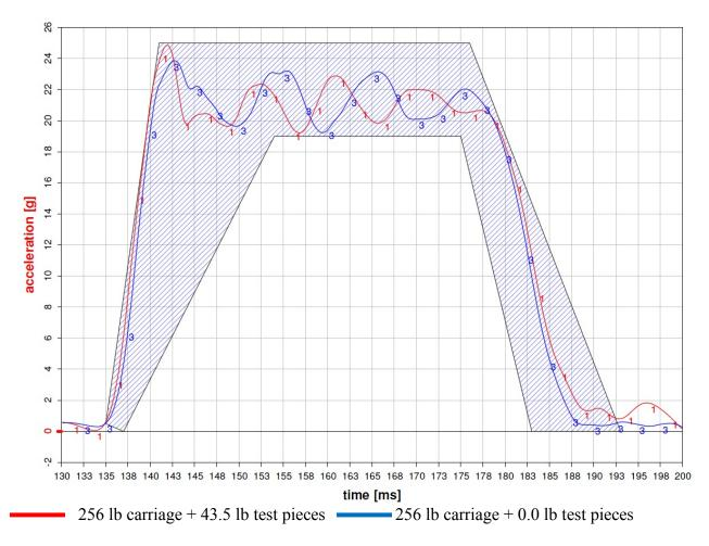
Figure 28: Acceleration (with corridor) for tests conducted with and without test pieces
