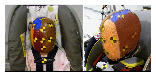
Figure B4: CRABI 12 and Q3s heads prepared for testing with targets, copper mesh cover, and test chalk
