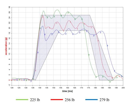
Figure 26: Acceleration of secondary carriage (with corridor) for three different weights
