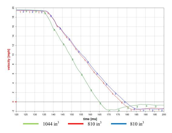
Figure 30: Relative velocity of the secondary carriage for varied aluminum honeycomb volume
