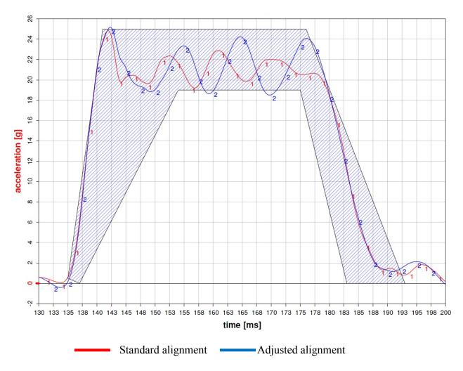
Figure 33: Acceleration of the secondary carriage (with corridor) for tests with two different impact plane alignments
