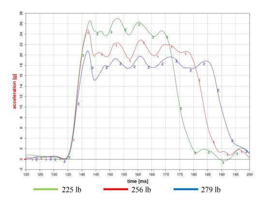
Figure 25: Acceleration of secondary carriage for three different weights
