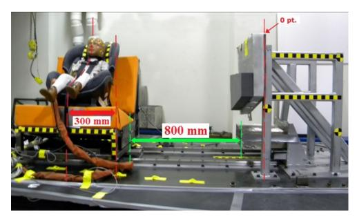
Figure B7: Pretest fixture dimensions
