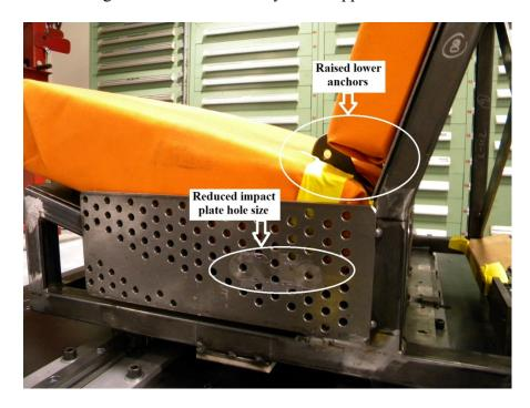
Figure 6: Modifications to the aluminum honeycomb striking plate and the lower anchor attachment brackets
