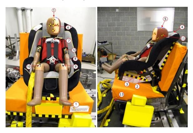
Figure B9: Layout of sample CMM measurement locations
