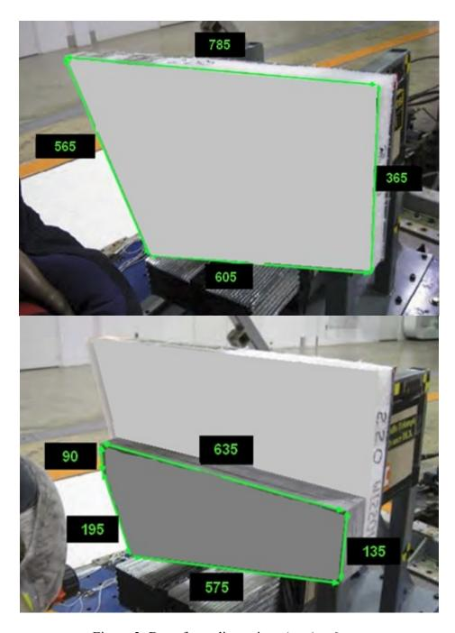
Figure 3: Door foam dimensions (mm)  $\pm$  6 mm
