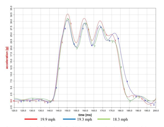
Figure 22: Acceleration time histories for side impact tests conducted at varying speeds (tests conducted with the 225 lb secondary carriage)
