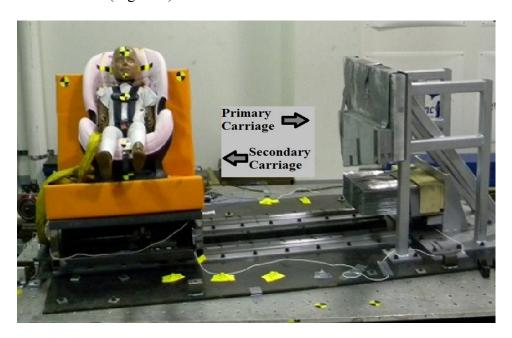
Figure 1: Side view of the side impact fixture attached to the deceleration sled
